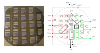
**Figure 5.6** – Electrosprayed 6 inch E-STARS wafer with different parameters for the study of morphology
