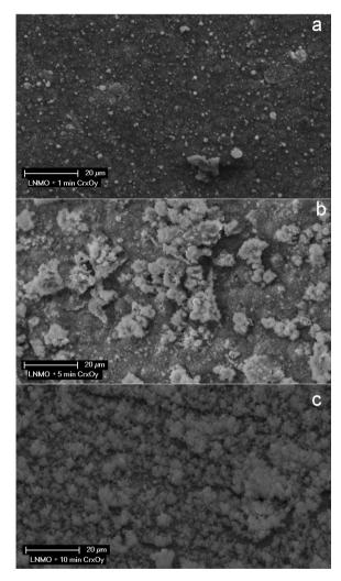
$\label{eq:Figure 6.5-SEM images of LiNi_0.5Mn_{1.5}O_4 films (dense background) with a $$ Cr_2O_3$ coatings (sponge-like on top) at different deposition times: (a)1 minute; (b) 5 minutes; and (c) 10 minutes$
