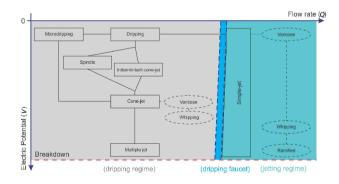
Figure 2.3 – Electrospraying modes as a function of the applied potential and flow rate. Adapted from [Agostinho, 2013]
