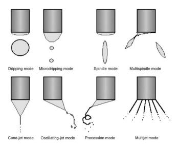
Figure 2.2 – Main modes of electrospraying. Adapted from [Jaworek et al., 2008]
