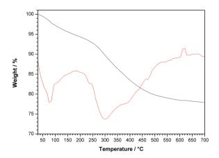
Figure 6.4 – Thermogravimetric analysis (and its derivative in red) obtained for the non-annealed sample synthesised at 400  $^{\circ}$ C
