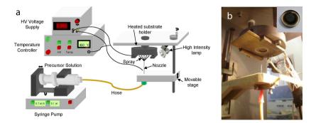
Figure 3.2 – Schematic drawing (a) and photo (b) of the electrostatic spray deposition setup used for the synthesis and coating of cathode electrodes, as will be discussed in Chapters 5 and 6. The picture on the right shows the circular mask used and the resulting film sprayed on a CR2320 coin cell cap.
