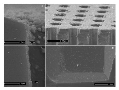
Figure 5.13 – SEM and XSEM images of the Si wafer presenting 3D HAR architecture. Cross section showing the layer on different parts of the trench (a) top (b) middle and (c) bottom. An overview of the film is shown in (d).
