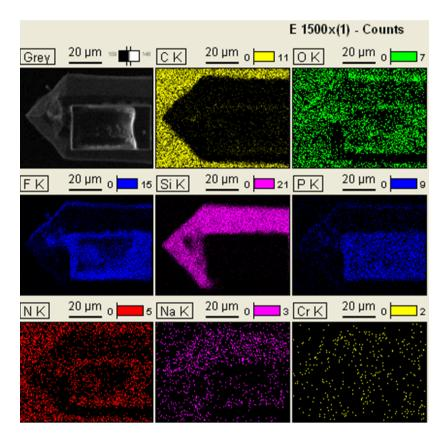
Figure 7.9 – EDX pictures of a probe cantilever and tip, from experiment F, taken one month after Figure 7.4(a and b). Color scales give the counts of elements in the picturer
