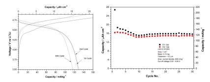
Figure 5.18 – Galvanostatic test on LAR E-STARS substrate with liquid electrolyte.
