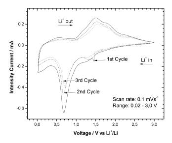
Figure 4.9 – CV plot for the Fe<sub>2</sub>O<sub>3</sub>/PVdF electrode deposited by ESP.
