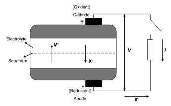
Figure 1.1 – Elements of an Electrochemical Cell Direction of the arrows correspond to the discharge.
