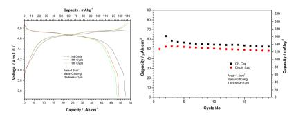
Figure 5.17 – Galvanostatic test using optimized parameters of Table 5.2 and a deposition time of 25 min.
