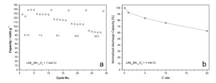
**Figure 6.11** – Rate capability and rate capability retention of 1 min Cr<sub>2</sub>O<sub>3</sub> partial-coated LiNi<sub>0.5</sub>Mn<sub>1.5</sub>O<sub>4</sub>. 1C=195 mA g<sup>-1</sup>
