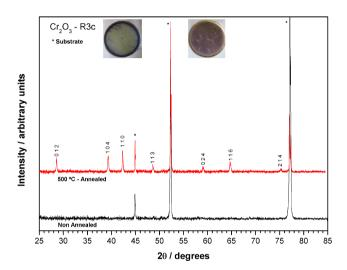
Figure 6.3 – XRD patterns of films synthesised by ESD at 400  $^{\circ}$ C (inset with pictures of the as-deposited materials). Black spectrum for the non-annealed sample (dark brown layer with reddish hue) and red pattern for the sample annealed at 500  $^{\circ}$ C (greenish layer). The peaks marked with asterisks belong to the support material.
