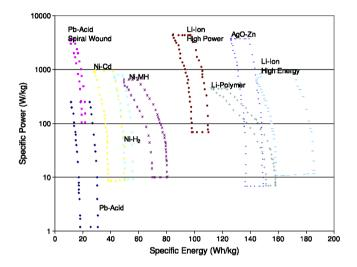
Figure 1.3 – Ragone plot comparing the performance of various battery electrochemistries. Note also that the various time intervals, in which the energy is being delivered, are indicated by the dotted lines. Adapted from [Cook-Chennault et al., 2008]
