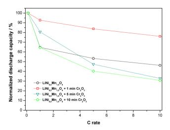
Figure 6.10 – Normalized discharge capacity values of  $LiNi_{0.5}Mn_{1.5}O_4$  samples before and after surface modification at various C rates
