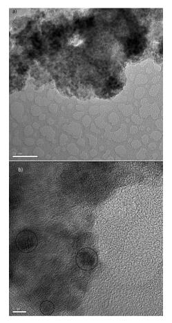
$\label{eq:Figure 4.5-TEM} \textbf{Figure 4.5} - \text{TEM bright field images showing (a) morphology and size of the $$\text{CuO/PVdF}$ nanocomposites and (b) lattice fringes of CuO at high resolution.}$
