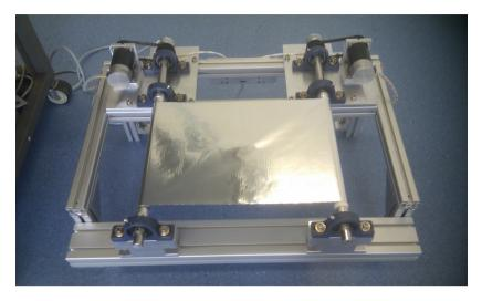
**Figure 3.6** – Preliminary design of a roll-to-roll system to be coupled with ESP coating device for the production of advanced electrodes.
