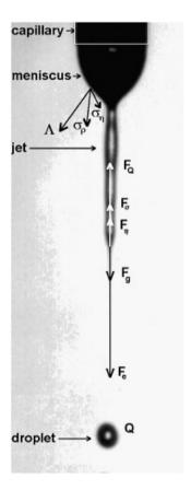
$\begin{tabular}{ll} \textbf{Figure 2.1} - Schematic illustration of stresses and forces on a liquid jet (spindle mode) flowing out from a capillary nozzle. Adapted from [Jaworek et al., 2008] \\ \end{tabular}$
