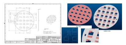
Figure 5.2 – Technical drawing of the metal mask (left hand image) for the deposition of the positive electrode (blue layer) on top of current collector layer (red layer) (right hand image)
