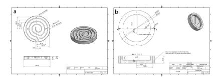
Figure 3.4 – Technical drawings of: (a) the heating plate containing two separate heating elements; and (b) the thermal isolation component.
