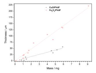
Figure 4.2 – Plot of the values of thickness vs. mass for the deposited electrodes of Cu/PVdF (open stars) and Fe<sub>2</sub>O<sub>3</sub>/ PVdF (solid stars) obtained for various sprayed volumes of the precursor solutions.
