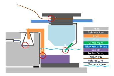
Figure 7.13 – Schematic of the faulty connections in the setup, half the cell is shown
