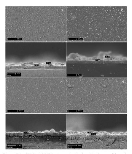
Figure 5.9 – SEM and XSEM micrographs showing the influence of the molar concentration in the morphology of the layers. (a) 0.01; (b) 0.025; (c) 0.05; (d) 0.1 M
