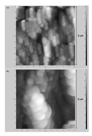
**Figure 4.3** – AFM images of the surface morphology of the nanocomposites. a) scan of CuO/PVdF (height bar 0-90 nm) and b) Fe<sub>2</sub>O<sub>3</sub>/PVdF (height bar 0-850 nm). The scanned areas are 2  $\mu$ m x 2  $\mu$ m wide.
