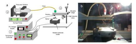
Figure 3.1 – Schematic drawing (a) and photo (b) of the electrostatic spray deposition setup used for the direct synthesis and assembly of coated nanocomposite electrodes, as will be discussed in Chapter 4. The nozzle, feeding hose and the heated substrate holder are clearly visible. The halogen lamp helps with the visualisation of the spraying mode.
