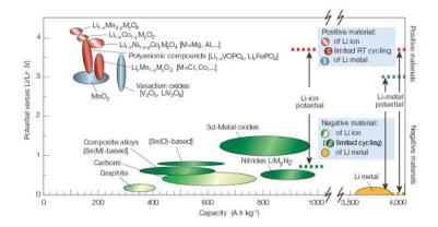
Figure 1.5 – Voltage versus capacity for positive- and negative-electrodes of rechargeable Li-based cells. Adapted from [Tarascon et al., 2001]
