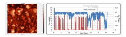
Figure 7.12 – (a) AFM scan of LNMO with chromium oxide, scanned in electrolyte (40x40  $\mu$ m); (b) Electrochemical behaviour of Si vs Li during AFM scanning
