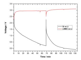
Figure 7.7 – Three-electrode measurements of LNMO (WE) vs Si (CE) and Li (RE)
