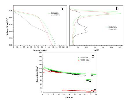
Figure 5.16 – Galvanostatic measurements of the high voltage spinel layers annealed at different temperatures: (a) charge-discharge voltage profiles; (b) differential capacity; (c) capacity retention upon progressive charge-discharge.
