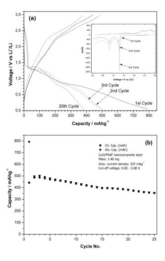
Figure 4.8 – Galvanostatic measurements of the composite CuO/PVdF electrode between 0.05 and 3.0 V at 337 mAg<sup>-1</sup>: (a) charge-discharge voltage profiles. The inset is a graph representing the differential capacity. (b) Capacity retention upon progressive charge-discharge.
