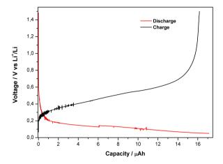
Figure 7.3 – Charge and discharge of silicon probe vs. metallic lithium (experiment B)
