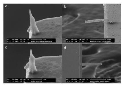
Figure 7.8 – NSG03 probes; (a) lithiated tip stored for 2 months; (b) bended cantilever, same as a; (c) same tip as a, directly after lithiation; (d) stored pristine probe, with no bended cantilever
