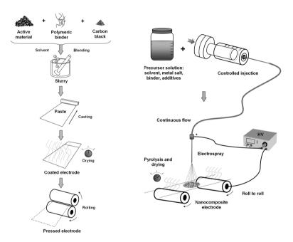
Figure 3.5 – Schematic drawing of (a) a typical manufacturing process of coated electrodes; and (b) the proposed on-step fabrication process. Adapted from Valvo, 2010 [19]
