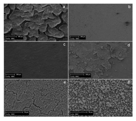
Figure 6.2 – SEM micrographs of the as-deposited layers using 2-propanol as solvent at different temperatures: (a) 300; (b, e) 350; (c, f) 400 and (d) 450  $^{\circ}{\rm C}.$
