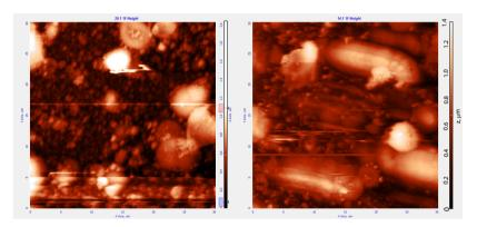
Figure 7.10 – AFM scan of LNMO with chromium oxide; (a) scanned with a pristine probe (30x30  $\mu$ m); (b) scanned with a lithiated probe(30x30  $\mu$ m)
