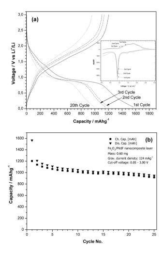
$\label{eq:Figure 4.10-Galvanostatic measurements of the composite $Fe_2O_3/PVdF$ electrode between 0.05 and 3.0 V at 124 mAg^{-1}: (a) charge-discharge voltage profiles. The inset is a graph representing the differential capacity. (b) Capacity retention upon progressive charge-discharge.$
