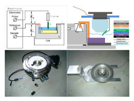
Figure 7.2 – (a) Scheme of the electrochemical setup with layout of connections: (1) sample (working electrode); (2) current-collector;(3) Li<sup>0</sup> reference electrode;(4) electrolyte; (5) cell housing; (6) Silicon SPM tip (counter electrode). (b) Cross-section schematic drawing of the liquid cell for the AFM; images of (c) bottom part; and (d) top part
