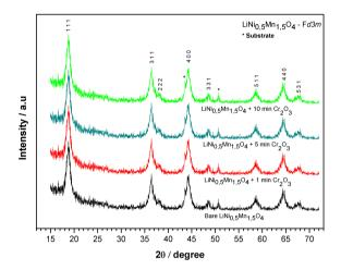
Figure 6.6 – XRD patterns of the non-coated and  $Cr_2O_3$  partially-coated  $LiNi_{0.5}Mn_{1.5}O_4$
