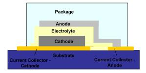
Figure 1.4 – Schematic representation of a planar solid-state thin film battery
