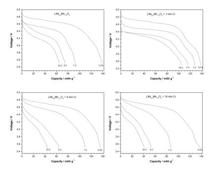
Figure 6.9 – Rate capability of  ${\rm Cr_2O_3}$  partial-coated and bare  ${\rm LiNi_{0.5}Mn_{1.5}O_4}$
