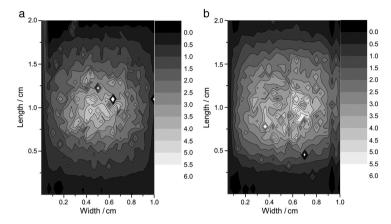
**Figure 5.5** – Surface morphology of film on Silicon wafer sprayed for (a) 10 min and (b) 40 min. Scale-bar on the left is in  $\mu$ m.
