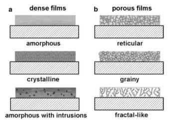
Figure 2.4 – Film structure morphologies: dense (a), porous (b). Adapted from [Jaworek, 2007]
