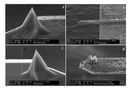
Figure 7.4 – SEM pictures of NSG30 tips; a) once discharged tip(in exp. E); b) once discharged tip and cantilever (in exp. E); c) pristine tip; d)once discharged and charged tip (in exp. F)
