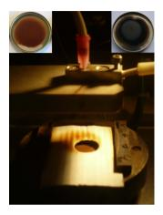
$\begin{tabular}{ll} {\bf Figure~4.1-Photo~of~the~reaction~chamber~were~the~direct~synthesis~and~assembly~of~coated~nanocomposite~electrodes~takes~place.~Examples~of~composite~coatings~with~PVdF~are~shown~as~insets~in~the~photo.\\ {\bf Fe_2O_3}~in~the~top~left-hand~corner~and~CuO~in~top~right-hand~corner.\\ \end{tabular}$
