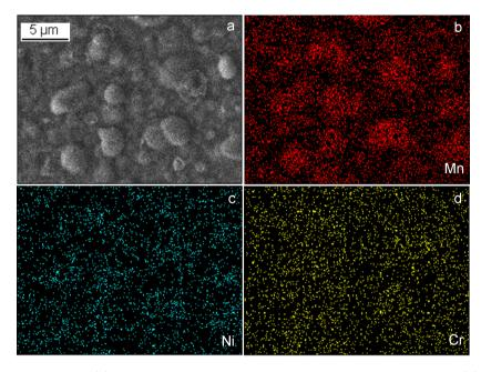
$\label{eq:Figure 6.7-(a) SEM image and corresponding EDX elemental mappings of (b) Mn, (c) Ni, and (d) Cr for the 1 min Cr_2O_3-coated LiNi_{0.5}Mn_{1.5}O_4$
