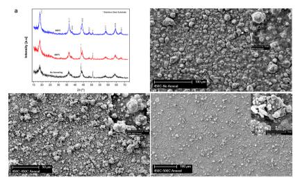
Figure 5.10 – Films synthesised at  $450^{\circ}\mathrm{C}$  and annealed at different temperatures. The effect in cristallinity can be seen in (a) XRD pattern (the peaks marked with dotted lines belong to the support material); SEM micrographs of (b) non annealed; (c) annealed at  $450^{\circ}\mathrm{C}$ ; (d) annealed at  $500^{\circ}\mathrm{C}$ .
