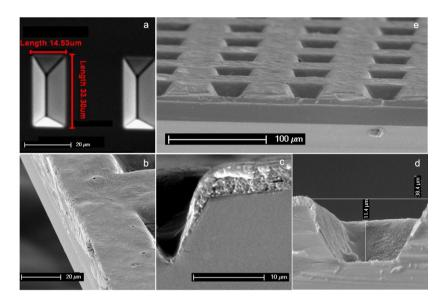
Figure 5.12 – SEM and XSEM images of the Si wafer presenting 3D LAR architecture (a) before and (b, c, d, e) after film deposition. (c, d) Cross section showing the film thickness.
