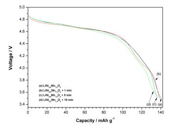
**Figure 6.8** – Discharge curves of  $LiNi_{0.5}Mn_{1.5}O_4$  before and after coating with  $Cr_2O_3$ . Discharge current density: 195 mA g<sup>-1</sup>
