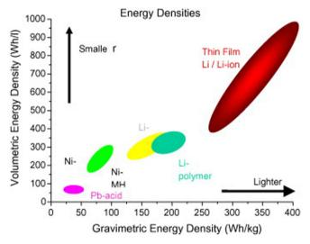
Figure 1.2 – Comparison of (rechargeable) battery technologies in terms of volumetric and gravimetric energy density. This particular graph excludes other technologies like lithium-sulphur and metal-air batteries. Adapted from [Patil et al., 2008]
