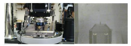
Figure 7.1 – Electrochemical cell in the AFM setup with SMENA head attached. (a) Side image and (b) digital microscope image (top) of immersed probe.
