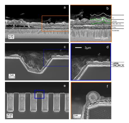
Figure 5.15 – Cross section SEM images of the complete stack on: flat substrate (a, b); LAR substrate (c, d); HAR substrate (e, f). SEM micrographs courtesy of CEA.
