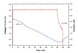
Figure 7.6 – Time profile of galvanostatic discharge (3  $\mu$ A) to a voltage value of 0.3 V, followed by 10 min potentiostatic discharge (experiment H)
