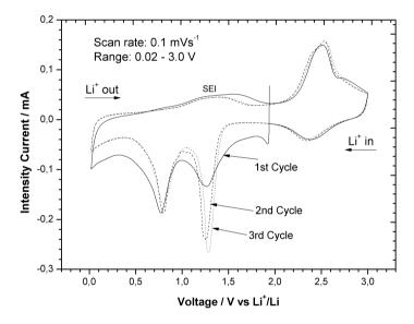
**Figure 4.7** – CV plot for the CuO/PVdF electrode deposited by ESP.
