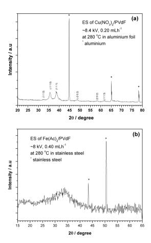
**Figure 4.4** – XRD spectra of the nanocomposite electrodes by electrostatic spray pyrolysis of (a)  $Cu(NO_3)_2.3H_2O$  /PVdF and (b)  $Fe(C_2H_3O_2)_2$ /PVdF at 280 °C. The peaks marked by an asterisk refer to the characteristic diffractions of the substrates used.
