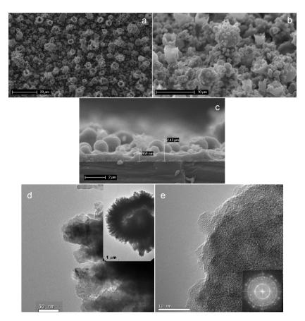
Figure 5.4 – (a and b) SEM micrograph of the film; (c) Cross section SEM; (d) TEM picture of the film texture (inset low magnification showing the fractal texture); (e) HR-TEM picture (inset Fourier Transform of the image)
