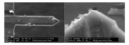
Figure 7.11 – Probe which was used to scan Figure 7.10(b); (a) cantilever (b) tip end
