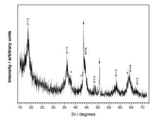
Figure 5.3 – XRD pattern of the  $LiNi_{0.5}Mn_{1.5}O_4$  film synthesised at 450°C. The peaks marked with asterisks belong to impurities, while those with arrows to the support material
