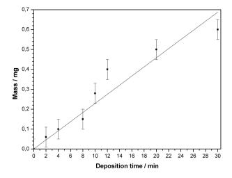
Figure 5.11 – Plot of the values of mass vs. time of deposition for deposited electrodes of  ${\rm LiNi_{0.5}Mn_{1.5}O_4}$  obtained for various sprayed volumes
