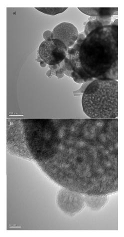
$\label{eq:Figure 4.6-TEM bright field images showing (a) morphology and size of the $$Fe_2O_3/PVdF$ nanocomposites and (b) local structure at high resolution showing the absence of lattice fringes.$
