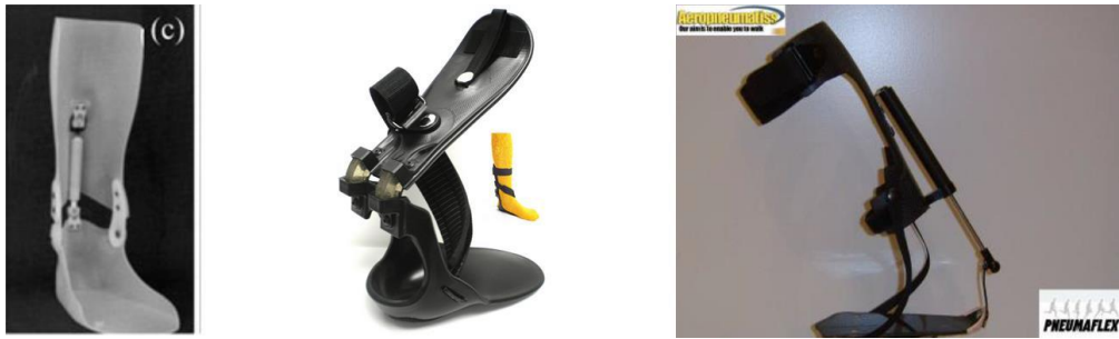
Figure 3: From left to right: DACS's AFO [10], Step Smart & Pneumaflex [11]. The three orthoses all add a positive stiffness to prevent plantarflexion while dorsiflexion is not hampered by any stiffness. From left to right different mechanisms are responsible to realize the stiffness; metal spring, rubber-like blocks and a pneumatic jack.
