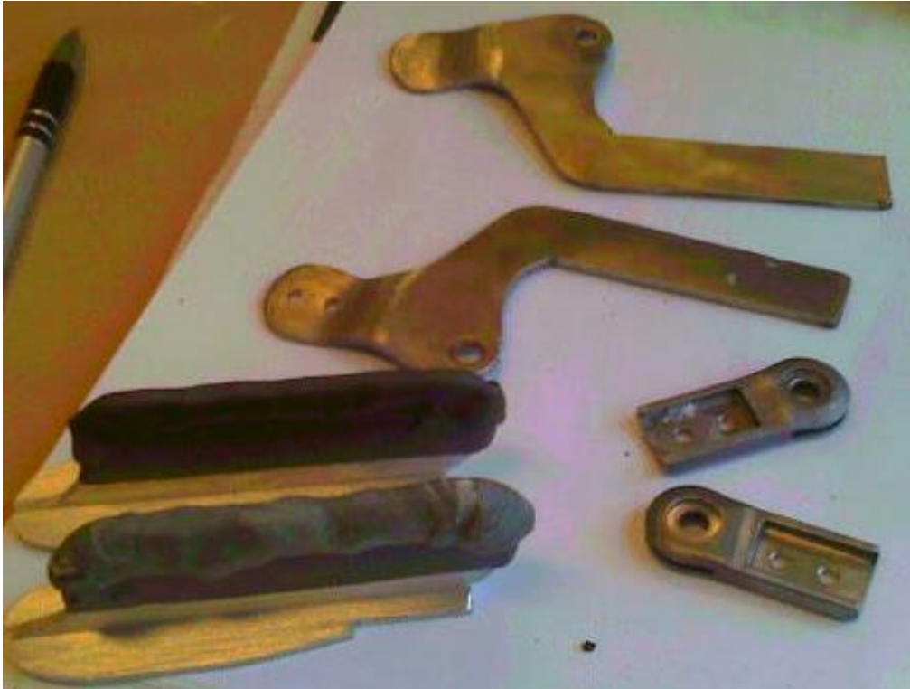
Figure 16, the prefabricated pieces. The two Otto-bock hinges at the bottom right side. The two stainless steel pieces to fit in the shoe side of the orthosis are shown above in the figure. The aluminum pieces are at the bottom left side, clay is added to prevent adhesion of epoxy raisin.
