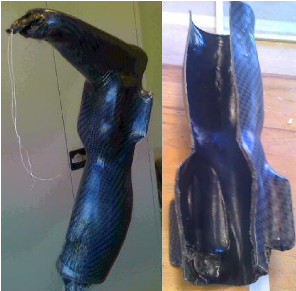
Figure 18. At the left side the NSO was just inseminated with raisin. At the right side the finalizing begins, the shin part of the NSO is separated from the cast mold.
