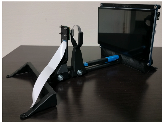
Figure 2.12: Compact star-tracker HIL setup ( Haraguchi, 2024 )
