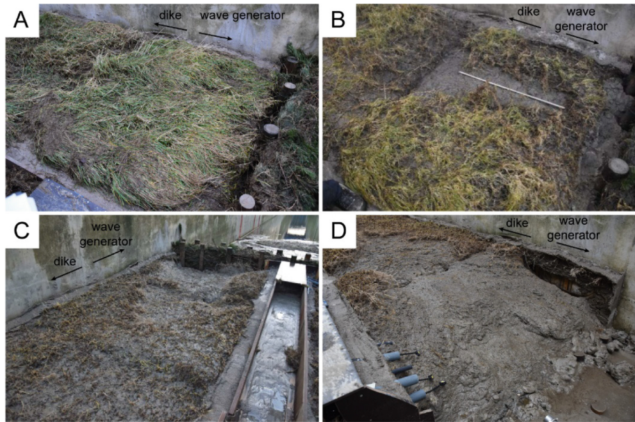
Fig. 3. Erosion at the saltmarsh cliff at the start of the experiment (A), after 17 h of testing (B), after 24 h of testing and mowing of vegetation (C) after removal brushwood dam and the end of the test program (D) (courtesy of Deltares)
