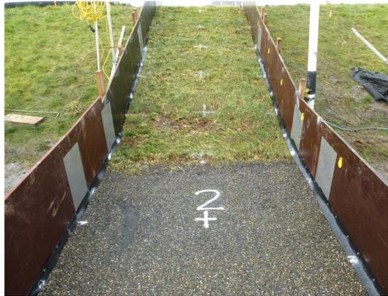
Figure 5.4. Slight erosion at the transition to the upper slope, test 2
