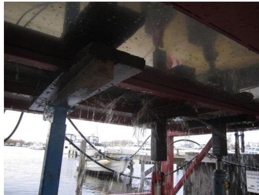
Picture 28. Small leakage with low filling level
