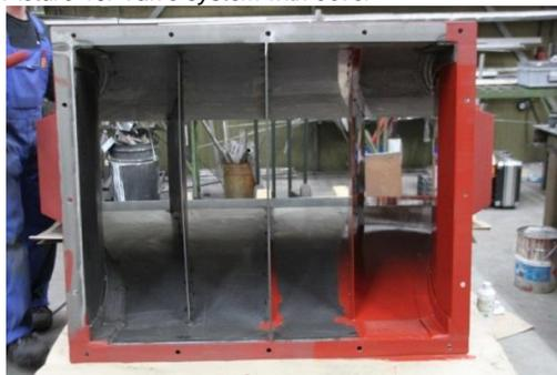
Picture 12. Inner part with guiding plates
