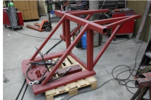
Picture 14 Frame for transport of modules
