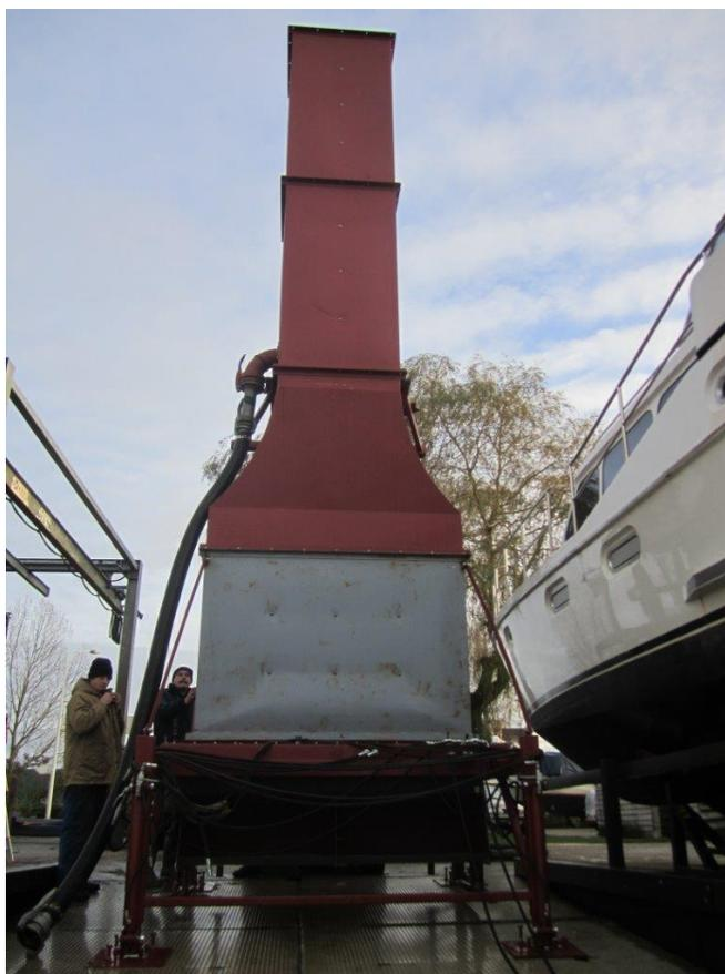
Picture 33. Testing with 7 m water column
