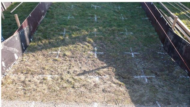
Figure 5.9. Quality of the grass berm was bad at Tholen (before testing)
