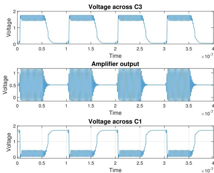
Figure 5.5: Envelope Detector Waveforms
