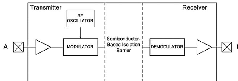
Figure 2.6: Conceptual Diagram of Inductive Communication protocol based system [1]
