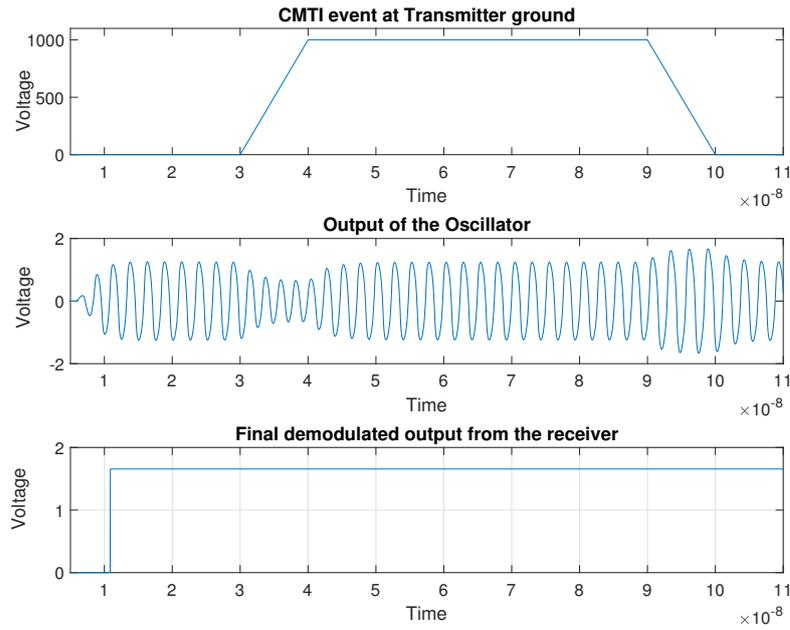
Figure 4.5: Effect of CMTI event after corrective measures
