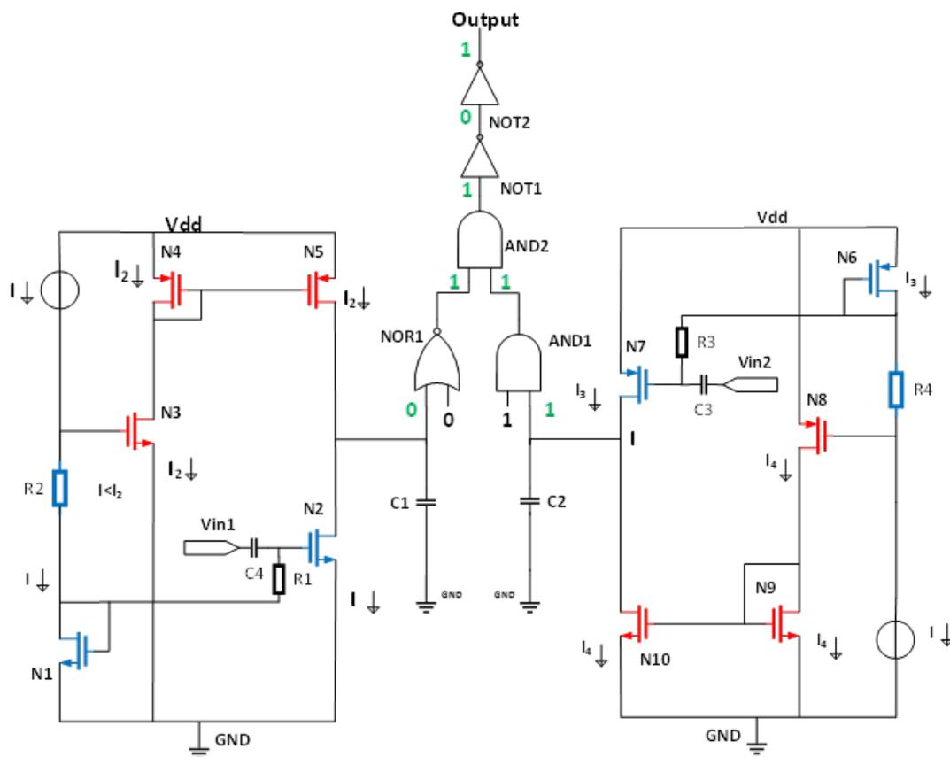
Figure 5.6: Envelope Detector Circuit during Oscillations
