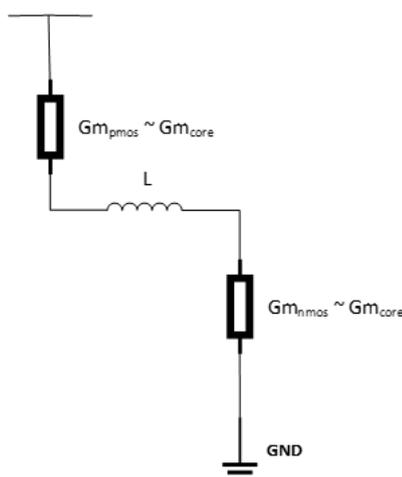
Figure 4.2: Equivalent Diagram of Oscillator during one half-cycle
