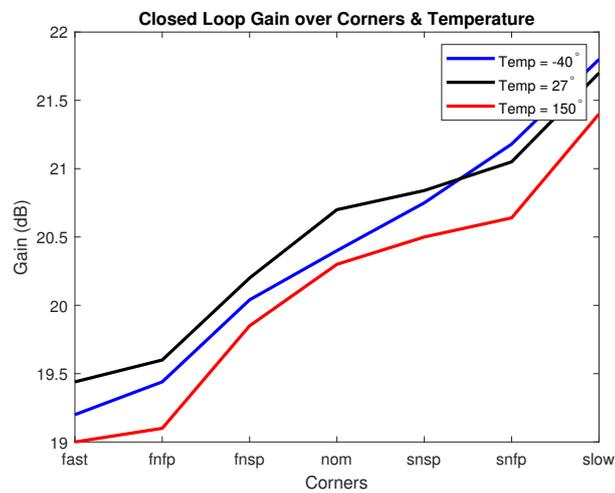
Figure 6.4: Amplifier Closed-Loop Gain over Corners and Temperatures
