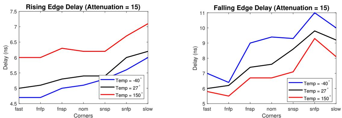
Figure 6.7: Delay Of signals when isolation offers an attenuation factor of 15
