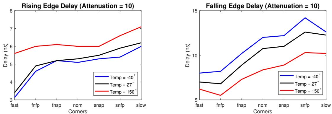
Figure 6.6: Delay of signals when isolation offers an attenuation factor of 10
