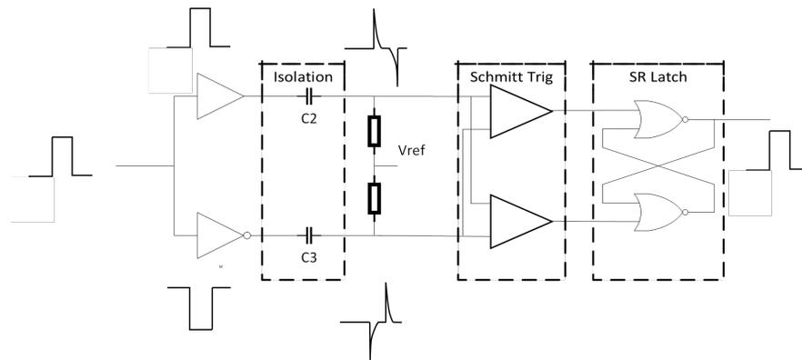
Figure 2.5: Capacitive Isolation Communication Protocol
