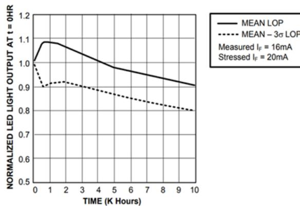
Figure 2.3: Optocoupler Light Output over Time [3]
