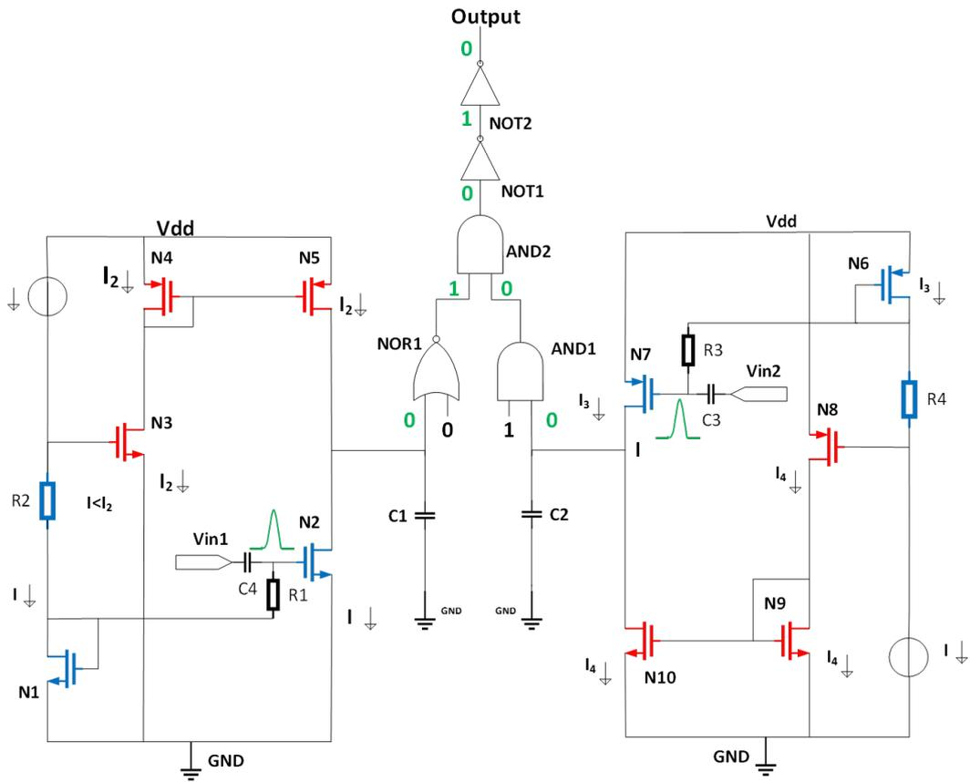
Figure 5.7: Envelope Detector Circuit during common-mode
