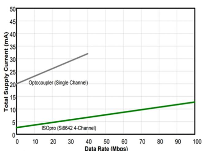
Figure 2.4: Current vs Data Rate Graph [3]
