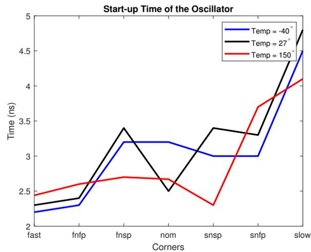
Figure 6.2: Time taken for the Oscillator to start Oscillating
