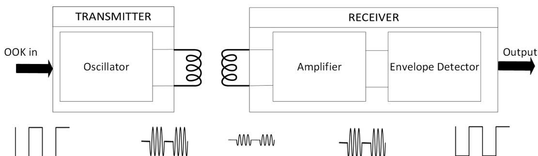
Figure 3.2: Signal Propagation across the system
