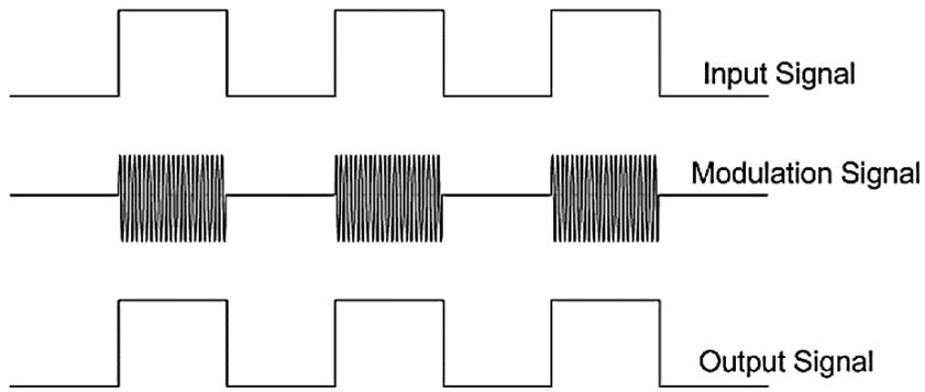
Figure 2.7: Representative signal in Inductive Communication
