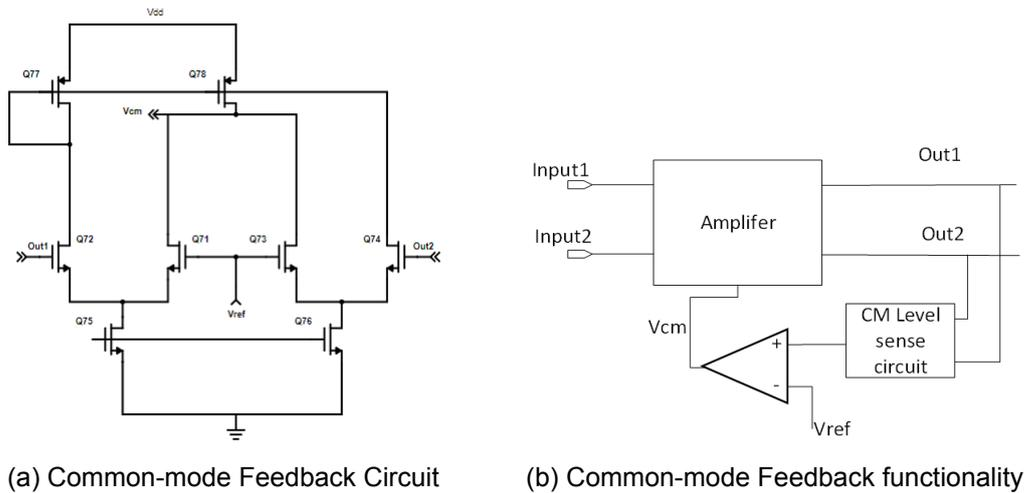
Figure 5.3: Common-mode Feedback
