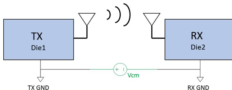
Figure 1.1: Basic Representation of a Digital Isolator
