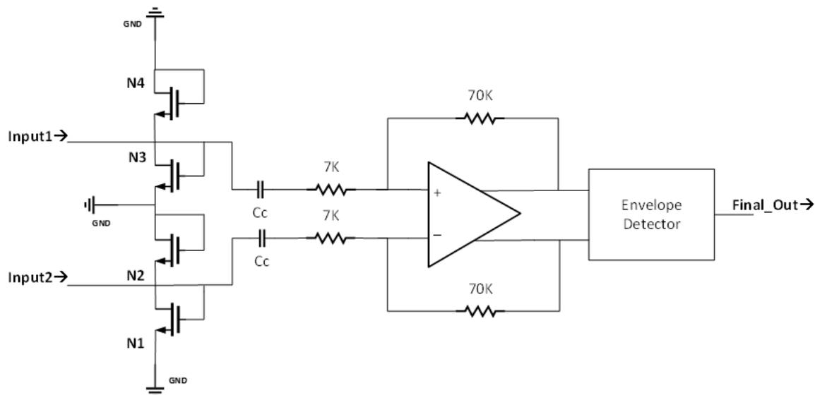
Figure 5.1: Receiver Structure
