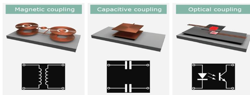
Figure 2.1: Different Types of Isolation Methods
