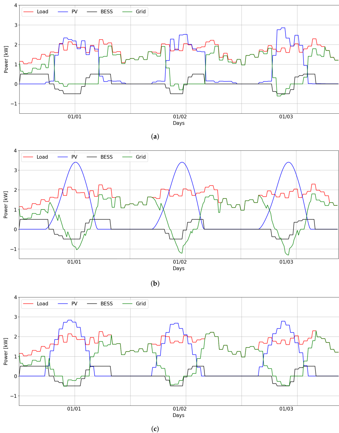
Figure 8. Comparison of (a) the instant power measured and the results obtained with (b) the Gaussian model and (c) the meteorological data-based model during a representative week, considering a self-consumption scenario.
