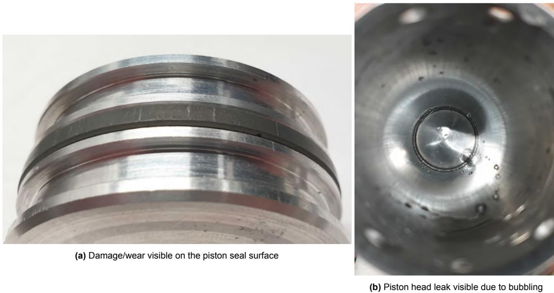
**Figure 6.2:** Damage to the piston seal and leak location visible
