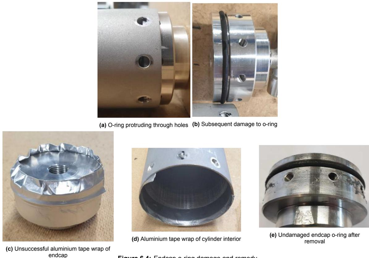
Figure 6.4: Endcap o-ring damage and remedy
