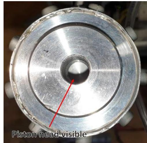
Figure 6.9: Piston head visible at top endcap after water filling
