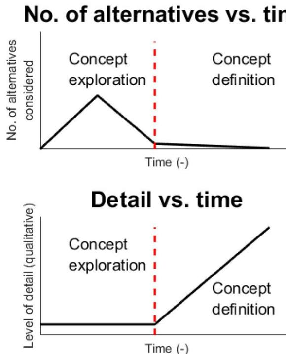
Figure 1: Concept exploration and definition process (van Oers *et al.*, 2018)
