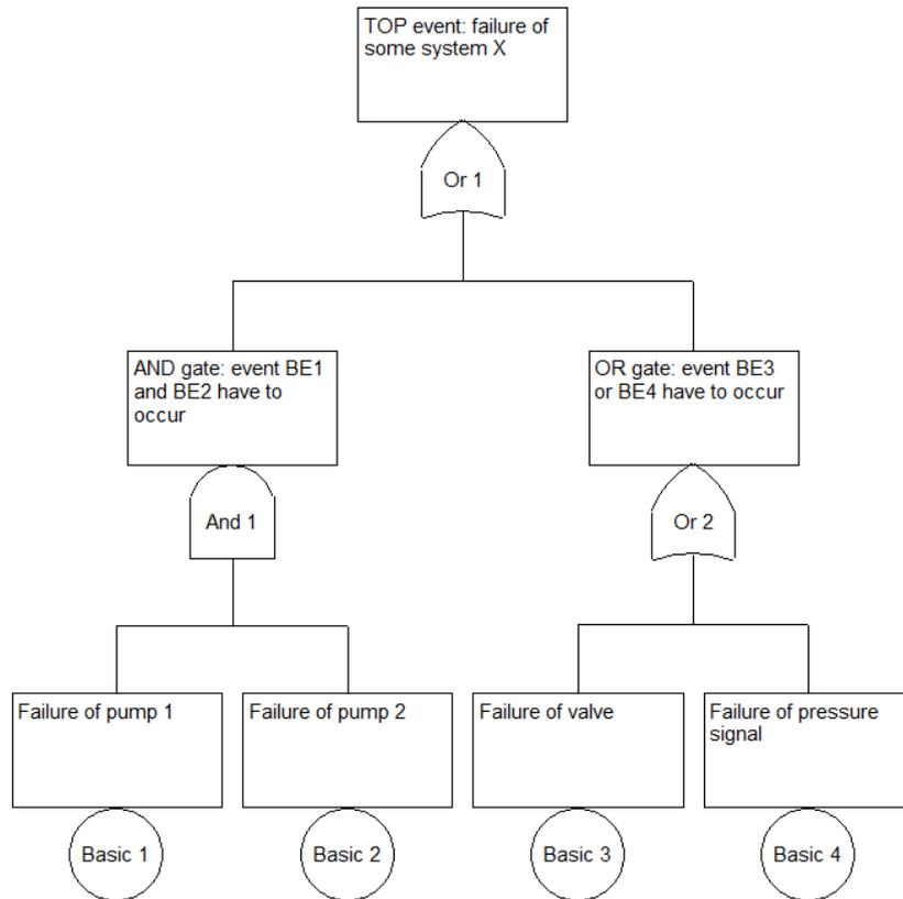
Figure 6: A simple fault tree for the top event that system X fails, own composition.
