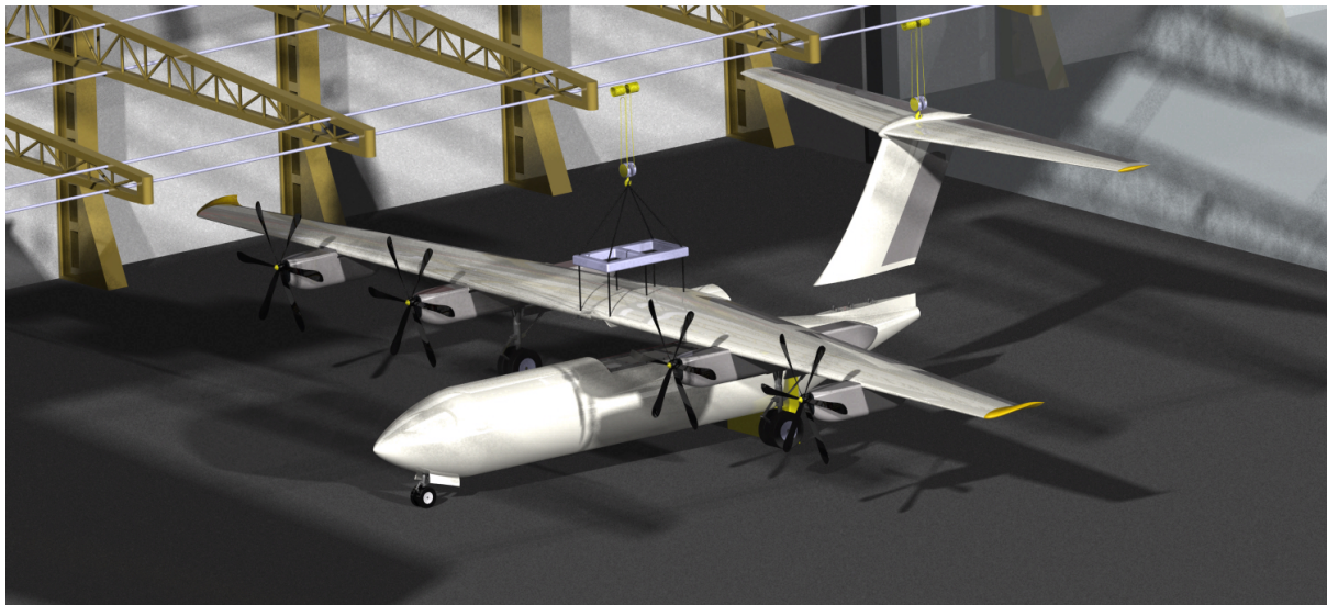
Figure 8.17: Reconfiguration of the ModuLR-300
