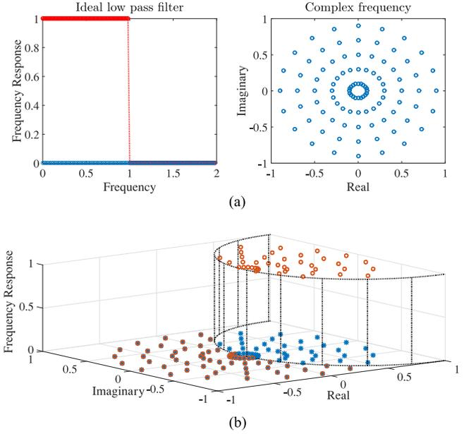
Fig. 2. (a) (Left) Ideal low pass filter response of universal design for undirected graph ( $N = 100$ ). (Right) Universal gridding for directed graph associated with the normalized adjacency matrix  $\mathbf{A}_n$  ( $N = 100$ ). (b) Ideal low pass filter response of universal design for directed graph with  $N = 100$ . The complex frequencies lying inside the circle with radius 1 centered at  $(1, 0)$  are “small” frequencies.
