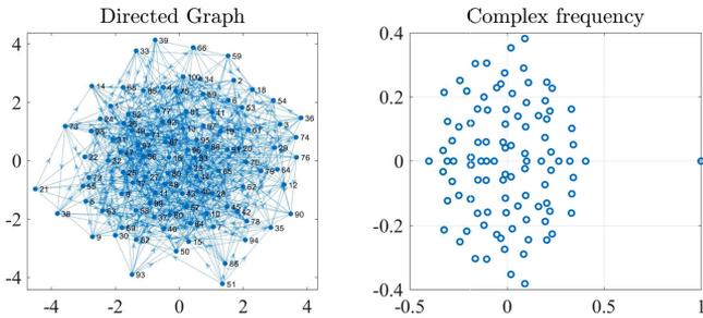
Fig. 1. Directed graph of  $N = 100$  nodes with  $E = 752$  edges having different weights in the interval  $[0, 3]$ . Complex-valued frequencies are generated by the eigenvalue decomposition of the normalized adjacency matrix  $\mathbf{A}_n$ . The “largest” frequency has magnitude one. Some frequencies live on the real axis while the remaining frequencies appear as conjugate pairs in the complex plane.
