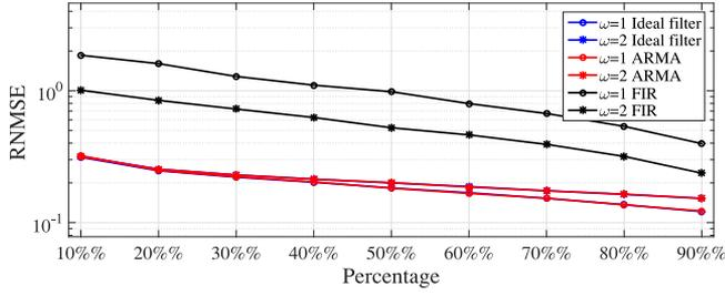
Fig. 6. RNMSE of the ARMA graph filter for interpolation of the Molene data set, where  $\omega = 1, 2$ . As two comparisons, the ideal graph filter and FIR filter with order  $K = 20$  are shown with the same values of  $\omega$ .
