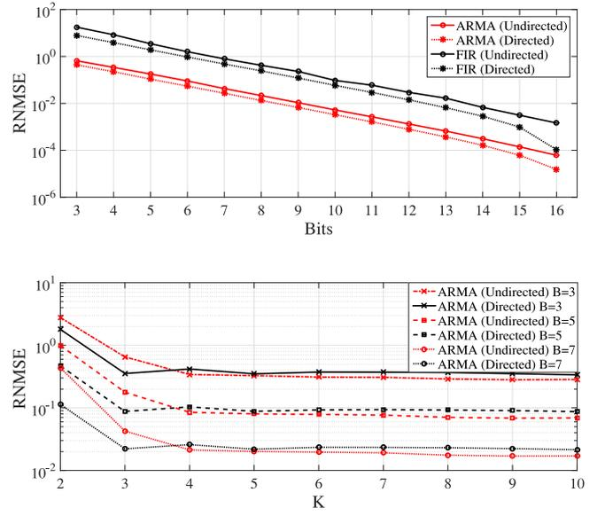
Fig. 8. Average RNMSE of linear prediction on the Molene temperature data set. (a) Average RNMSE of the approximated signal as a function of the number of bits ( $B$ ) for filter order  $K = 3$ . (b) Average RNMSE of the estimated signal for different order ARMA filters evaluated for  $B = 3, 5, 7$ .
