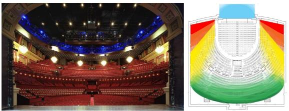
Figure 7.14a & 7.14b Sightlines from seats in auditorium of Carré, self-designed (Blue = the stage, Red sees up to 50% of the stage (about 74 seats), Orange sees up to 75% of the stage (about 90 seats), Yellow sees up to 90% of the stage (about 200 seats), Light Green has limited view because of distance to stage (about 238 seats), Dark green has very limited view because of extreme long distance to stage (about 90 seats) (Greiner, 2005; Stichtingtekening, 2005)
