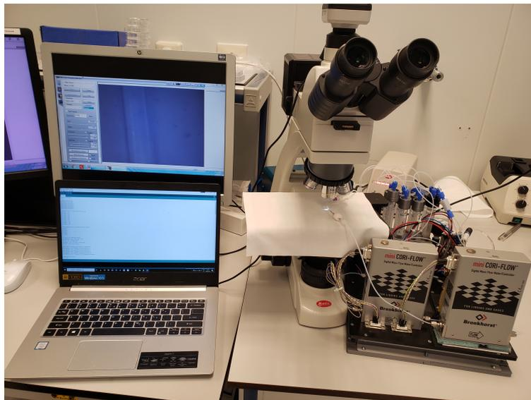
Figure E.3: Photo of bubble test experiment. The Arduino program is on laptop while the screen at upper-left is used to monitor the bubbles in microchannels. The platform is put beside the microscope because the equivalent chip is too bulky to keep sufficient distance for focusing. It will not be a problem in real-chip experiments since real chips are small enough to be put into the window.
