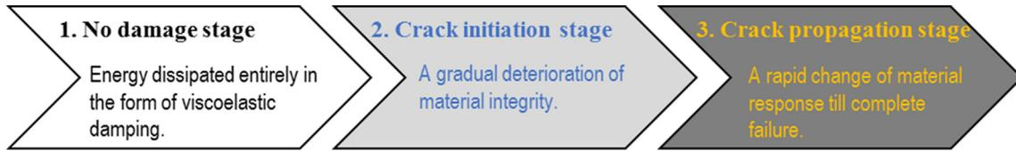
Fig. 3. Fatigue damage evolution of binders.
