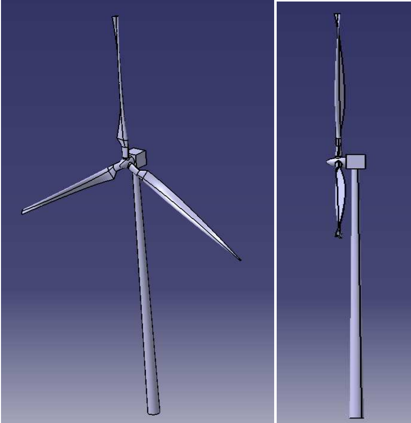
Figure 2.24: Isometric (left plot) and side view of the 2 nd symmetric torsion mode.
