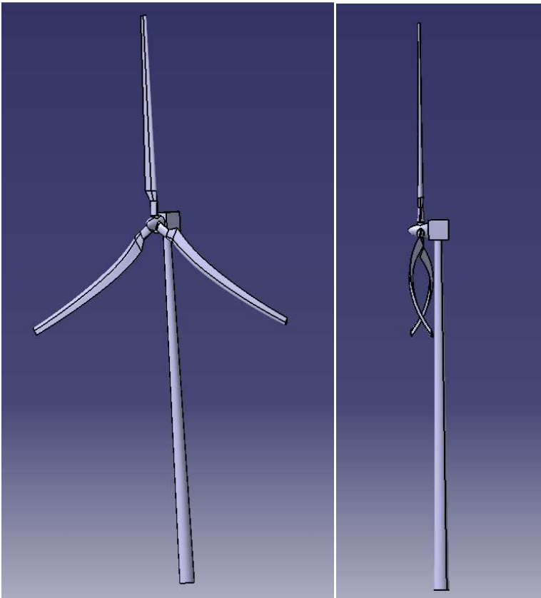
Figure 2.20: Isometric (left plot) and side view of the 2 nd flap-wise BW mode.
