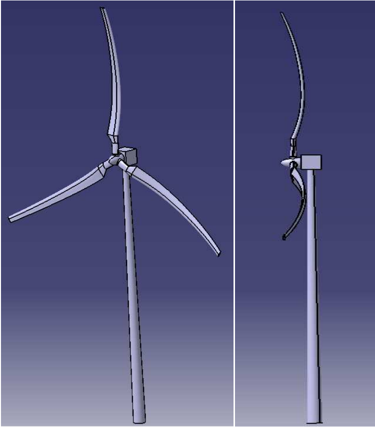
Figure 2.19: isometric (left plot) and side view of the 2 nd symmetric flap-wise mode.
