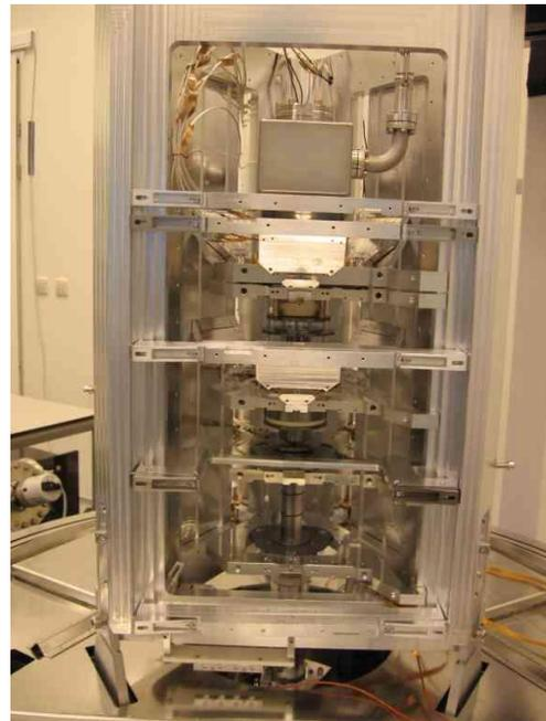
Figure 4. Photograph of one of the Demonstrators electron optics columns
