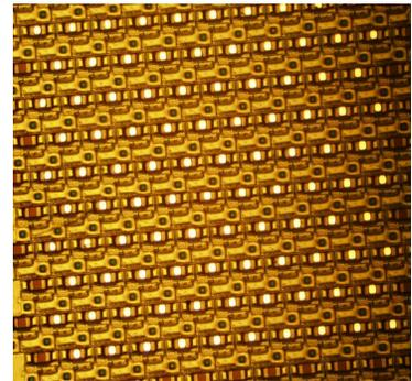
Figure 7. Optical microscope picture of real beam blaker array
