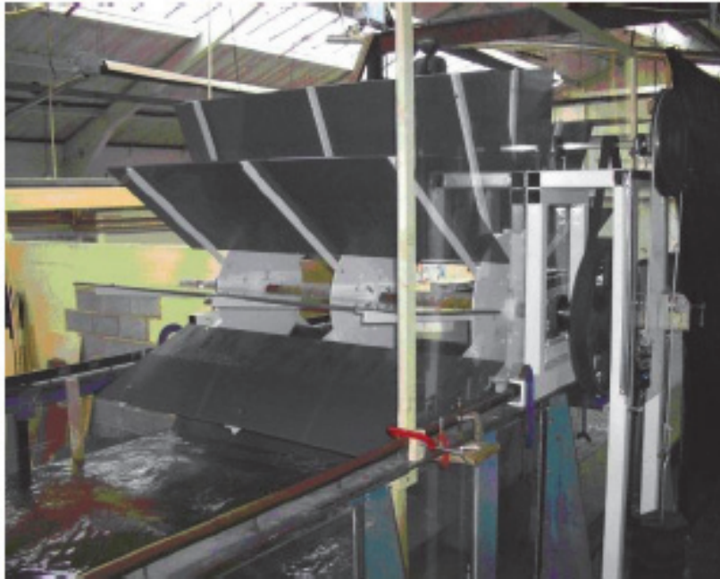
Figure 7-6: Hydrostatic pressure wheel in the laboratory flume
