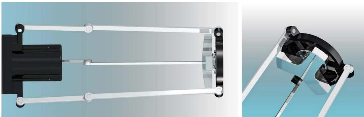
**Figure 11.8** Original design of secondary mirror [4]
