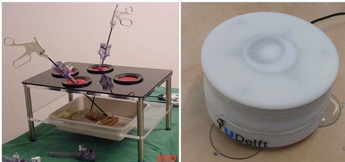
**Fig. 1** *Left* Standard box for laparoscopic training. *Right* New and waterproof version of the Force Platform
