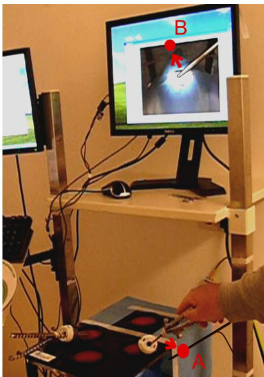
**Fig. 5** Determination of the total time delay. An additional camera (not in photo) is placed in front of the system and records the instrument's movements and monitor simultaneously. After recording, the number of frames can be counted between the moment the real instrument reaches point A and the moment that the displayed instrument reaches the corresponding point B at the screen
