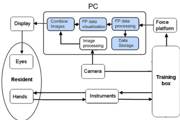
**Fig. 4** Time delays in the training system. The colored blocks show where noticeable processing time is lost during training. The total time delay is determined by a summation of the delays in each individual colored block in the representation
