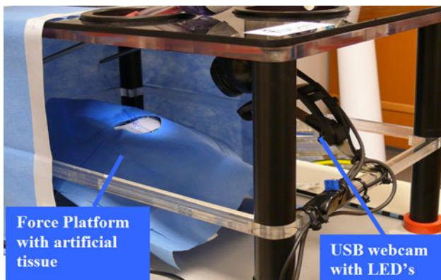
**Fig. 2** A webcam, light source, and new Force Platform equipped with artificial tissue are fixed inside the custom-made box trainer
