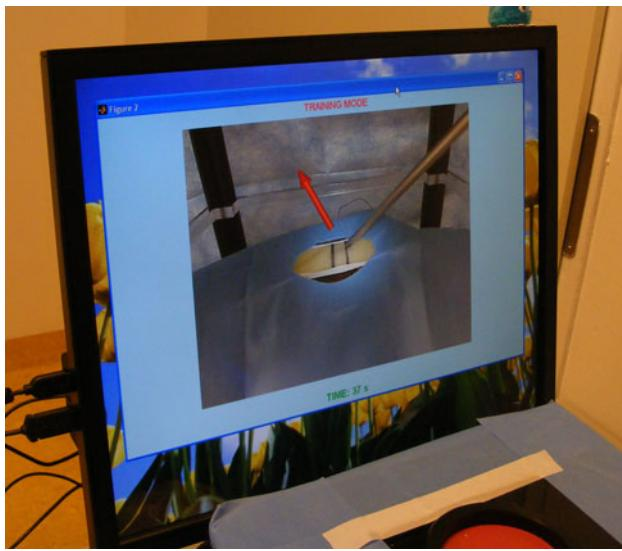
**Fig. 3** Arrow representation of the force magnitude and direction. The arrow is displayed as an overlay inside the laparoscopic image. An offset between point of needle insertion and arrow prevents blockage of the view of interest
