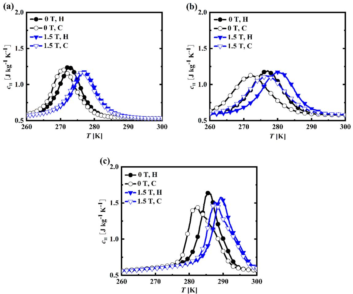
**Fig. 1.** Specific heat capacity versus temperature curves for (a)  $\text{Mn}_{1.32}\text{Fe}_{0.67}\text{P}_{0.52}\text{Si}_{0.49}$ , (b)  $\text{Mn}_{1.37}\text{Fe}_{0.63}\text{P}_{0.5}\text{Si}_{0.5}$ , and (c)
