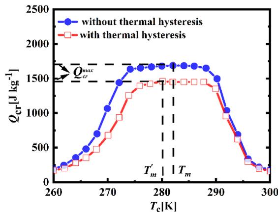
Fig. 5. The curves of  $Q_{cr}$  varying with  $T_c$  in the regenerative Brayton refrigeration cycles employing the composite material as the
