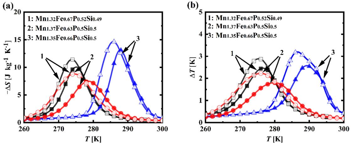
**Fig. 2.** (a) Isothermal magnetic entropy changes and (b) adiabatic temperature change versus temperature curves for Mn-Fe-P-Si materials with heating (filled symbols) or cooling (open symbols) under 1.5 T field change.
