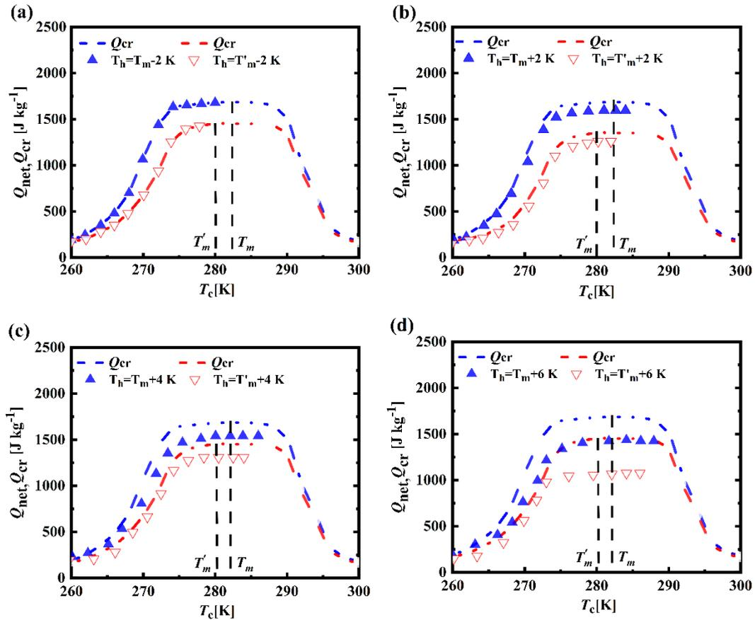
**Fig. 6.** The  $Q_{\text{net}}$  and  $Q_{\text{cr}}$  varying with  $T_c$  curves of the WOH or WH cycle employing the composite material as the working medium for a fixed  $T_h$  with (red) or without (blue) thermal hysteresis.
