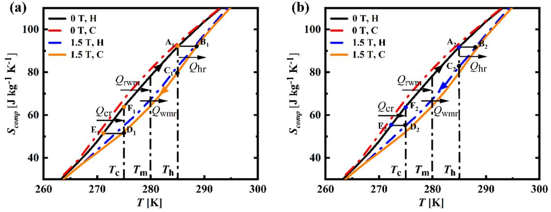
**Fig. 4.** Total entropy  $S_{comp}$  of the composite material varying with temperature  $T$  at 0 and 1.5 T magnetic fields and the schematic diagrams of regenerative Brayton refrigeration cycles (a) without or (b) with thermal hysteresis.
