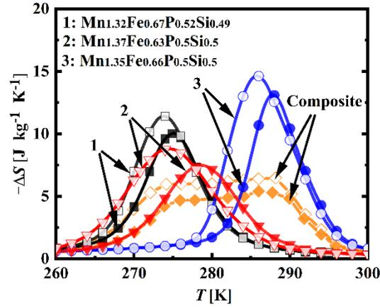
**Fig. 3.** Isothermal magnetic entropy changes for the Mn-Fe-P-Si composite and component materials varying with temperature under applied magnetic fields 0 and 1.5 T (solid icon: heating; hollow icon: cooling).
