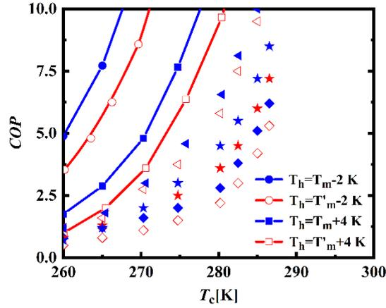
**Fig. 7.** The  $COP$  versus  $T_c$  curves in the WOH or WH cycle (WOH: blue; WH: red) employing the composite (circle and square) or component materials (1:  $Mn_{1.32}Fe_{0.67}P_{0.52}Si_{0.49}$ : rhombus; 2:  $Mn_{1.37}Fe_{0.63}P_{0.5}Si_{0.5}$ : triangle; and 3:  $Mn_{1.35}Fe_{0.66}P_{0.5}Si_{0.5}$ : star) as the working medium for given  $T_h$ .
