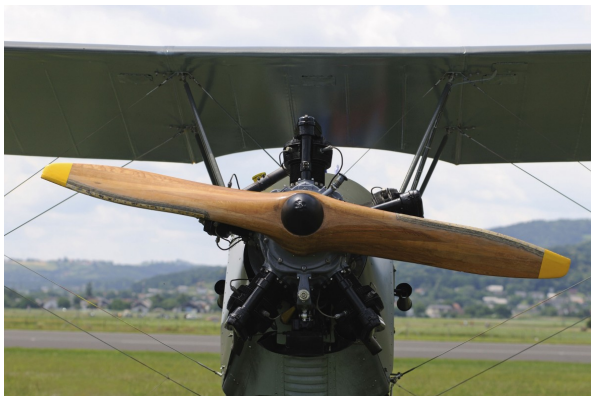
Figure 2.3: Picture of a fixed pitch propeller 2 .
