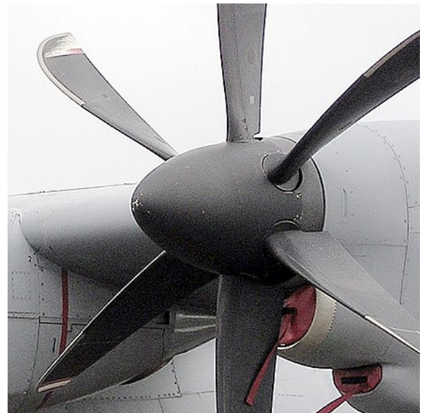
Figure 2.4: Picture of a variable pitch propeller 3 .
