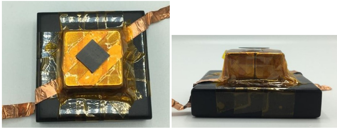
(a) The top view of the setup consisting of the magnets, the electrodes, the kepton tape and the levitating plate. (b) The side view of the setup consisting of the magnets, the electrodes, the kepton tape and the levitating plate.
