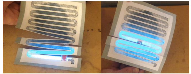
Figure 4. The gradient effect achieved by altering the form of the printed top-conductor.
