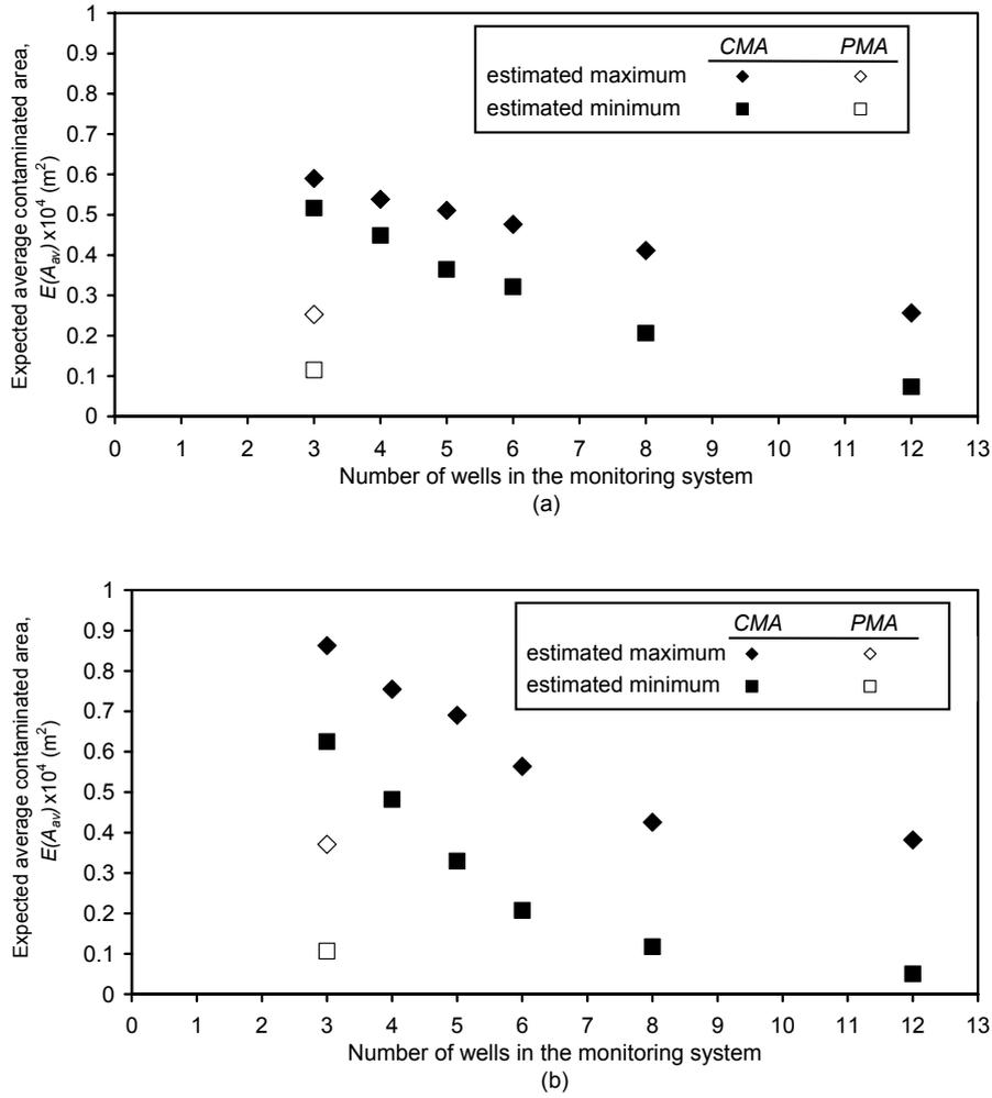
Figure 6.9: Comparison of the conventional monitoring approach (*CMA*) and the proposed monitoring approach (*PMA*) (pumping rate = 100 l/day) in terms of the expected average contaminated area  $E(A_{av})$  “in homogenous medium”: (a) transverse dispersivity,  $\alpha_T = 0.01$  m and (b) transverse dispersivity,  $\alpha_T = 0.03$  m.
