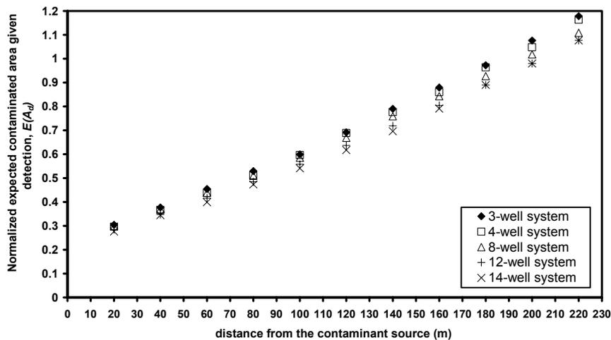
Figure 7.5: Normalized expected contaminated area given detection  $E(A_d)$  as a function of distance from the contaminant source  $d$  for selected monitoring systems for *MONIDAM* application.
