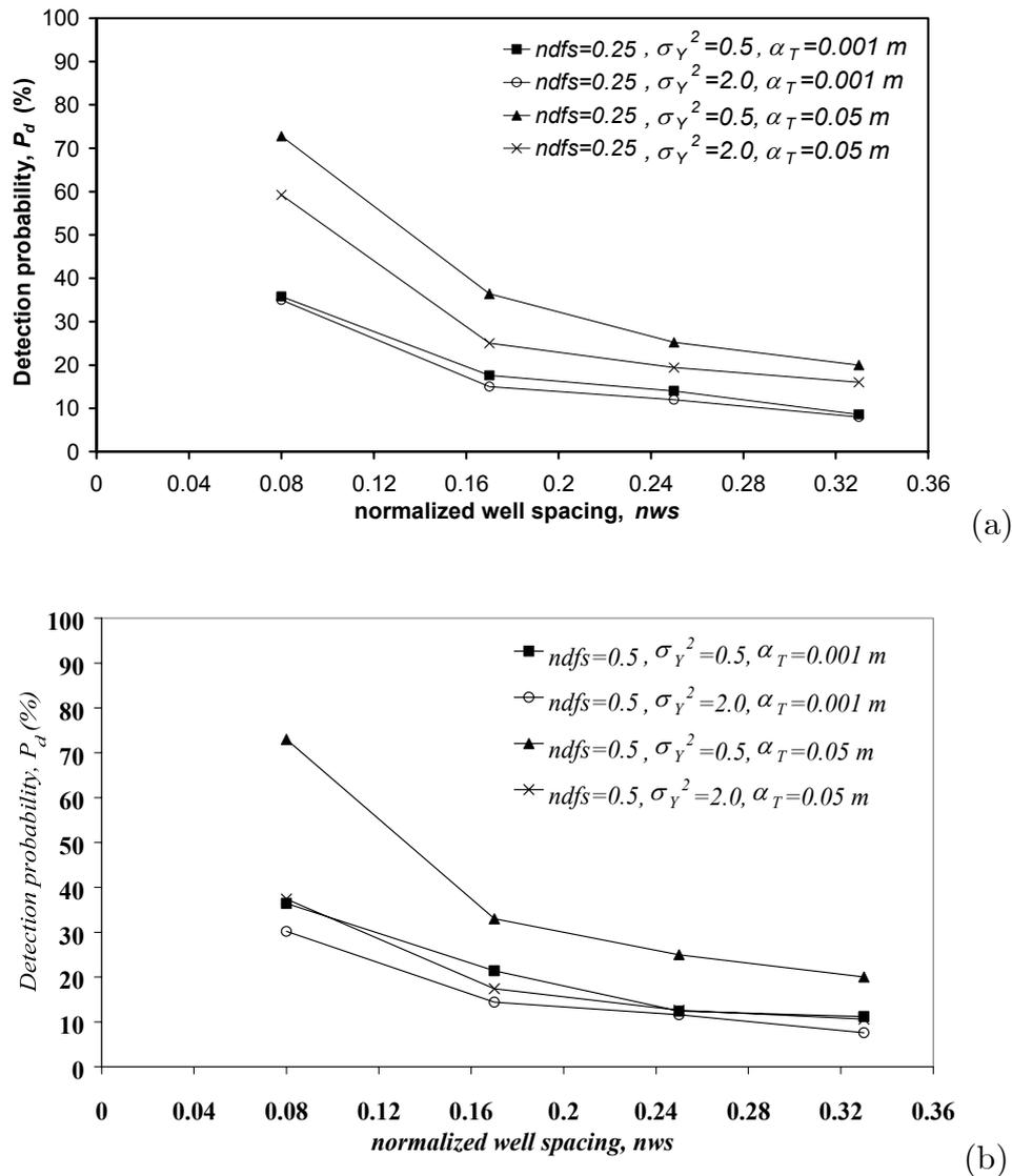
Figure 4.3: Detection probability,  $P_d$  as function of normalized well spacing,  $nws$  for medium with different degree of heterogeneity and dispersivity for normalized distance from the source, (a)  $ndfs=0.25$  and (b)  $ndfs=0.50$ .
