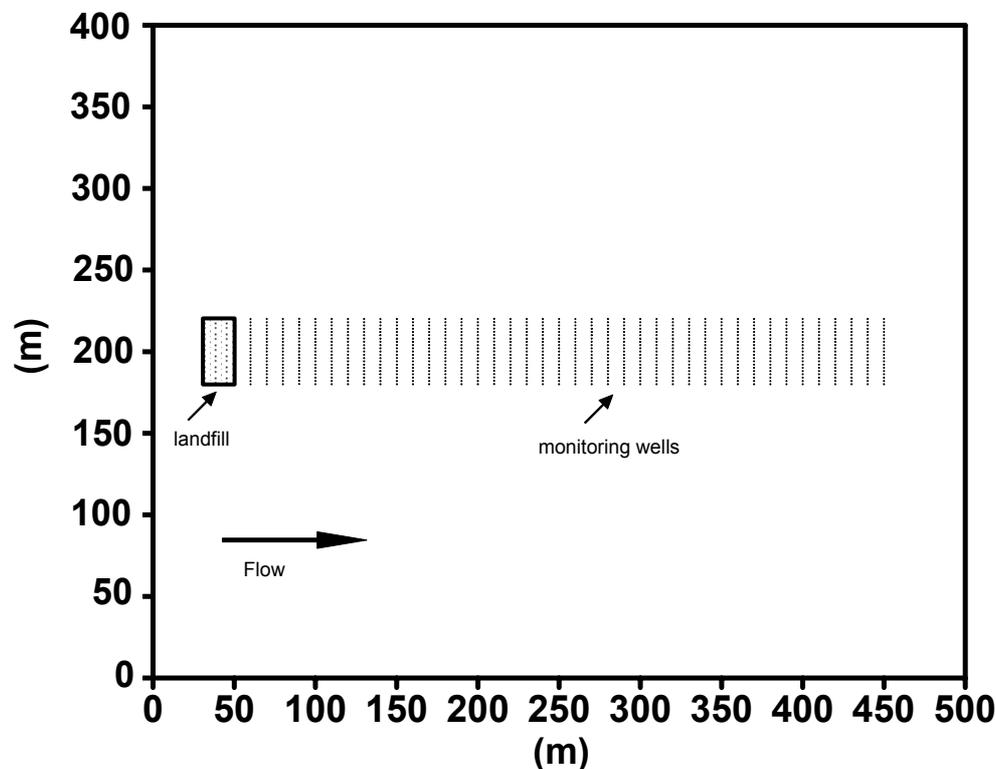
Figure 3.2: Dimensions and components of the example with 840 monitoring well locations.
