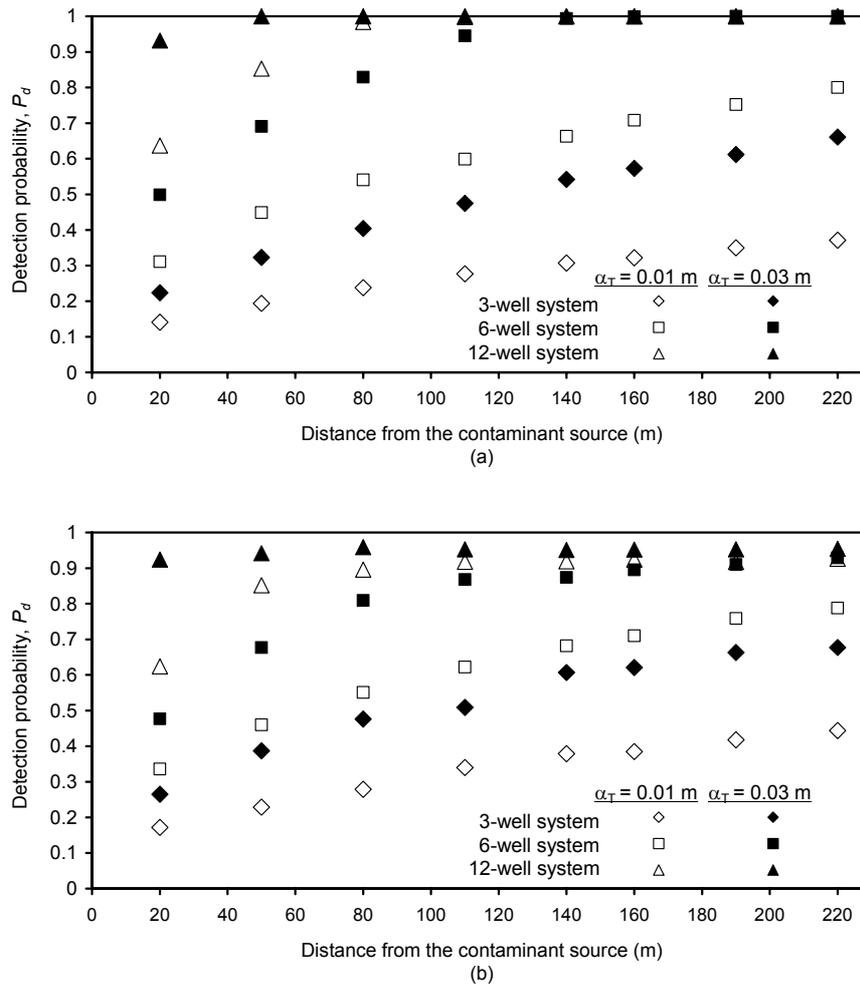
Figure 6.2: System reliability as a function of distance from the source for selected monitoring systems for conventional monitoring approach (CMA): (a) homogenous medium, and (b) heterogeneous medium.
