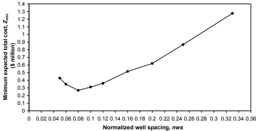
Figure 5.9: Minimum expected total cost as a function of normalized well spacing  $nws$ .
