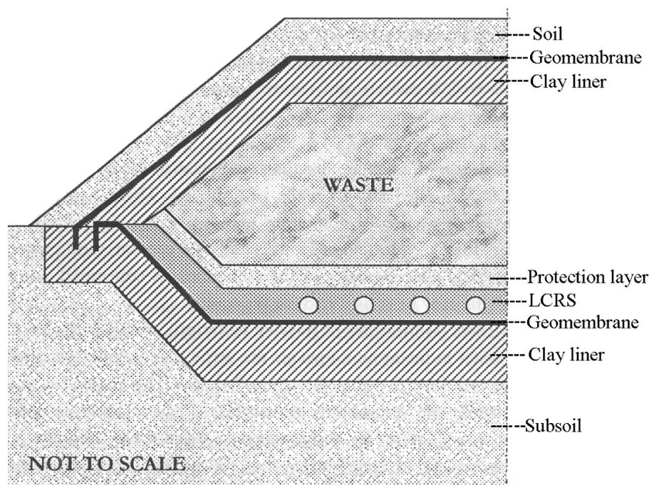
Figure 1.2: Cross-section of a landfill.
