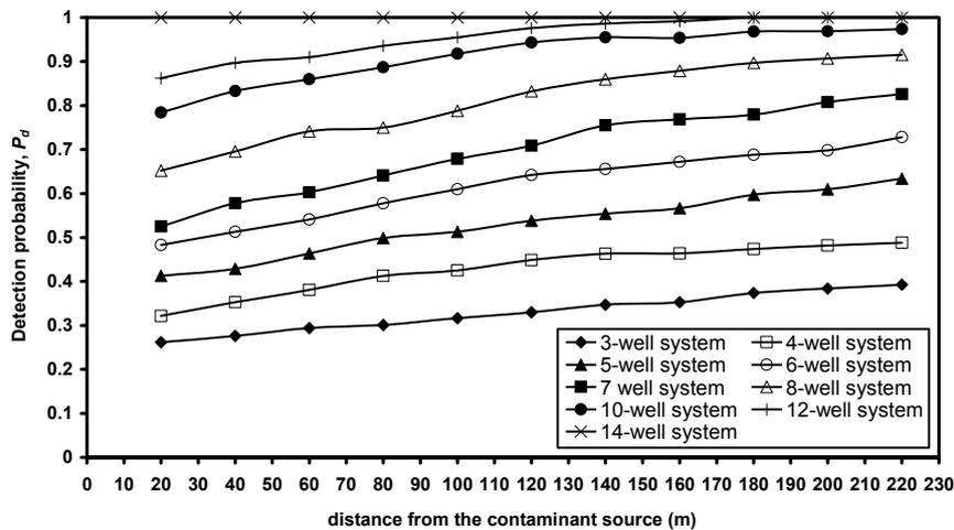
Figure 7.4: System reliability as a function of distance from the contaminant source  $d$  for different monitoring systems for the *MONIDAM* application.
