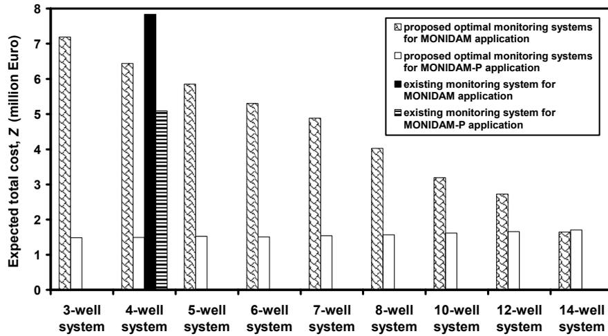
Figure 7.7: Comparison of the proposed monitoring systems to the existing monitoring system in terms of expected total cost,  $Z$ .
