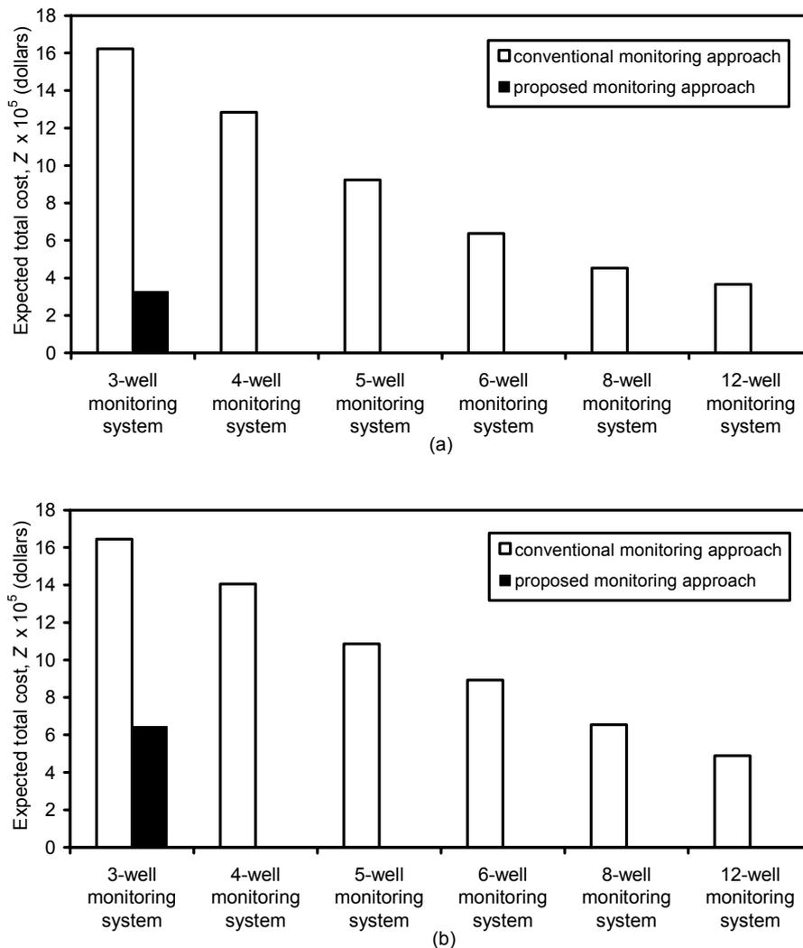
Figure 6.11: Expected cost as a function of number of wells in a monitoring system for transverse dispersivity,  $\alpha_T = 0.03$  m: (a) homogenous medium and (b) heterogeneous medium.
