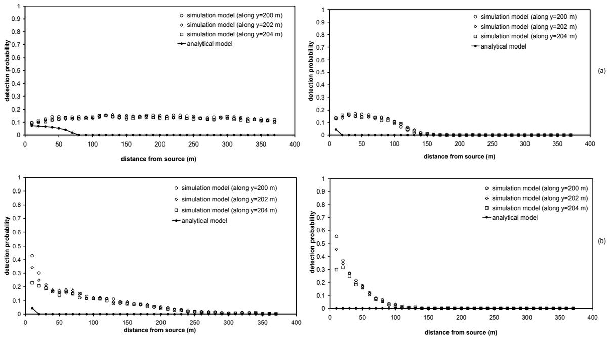
Figure 3.9: Comparison of detection probability values at selected well locations computed by simulation and analytical models for an instantaneous leak in the heterogeneous case (a) Case 1a and Case 2a, (b) Case 1d and Case 2d.
