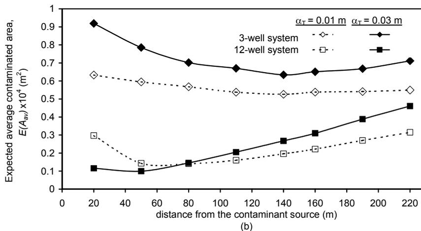
Figure 6.3: Expected average contaminated area  $E(A_{av})$  as a function of distance from the source for selected monitoring systems for conventional monitoring approach (CMA): (a) homogenous medium and (b) heterogeneous medium.
