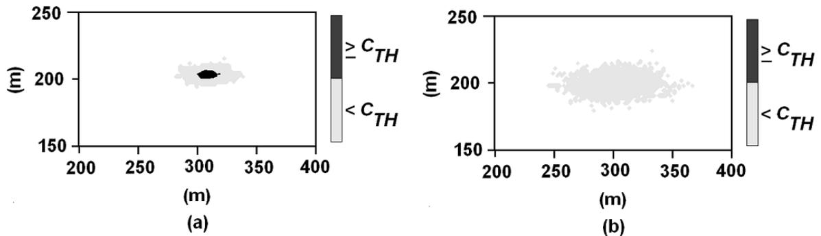
Figure 4.6: Single realization of a plume in a medium with transverse dispersivity,  $\alpha_T=0.02$  m where a) variance of  $Y$ ,  $\sigma_Y^2=0.5$  b) variance of  $Y$ ,  $\sigma_Y^2=2.0$ .
