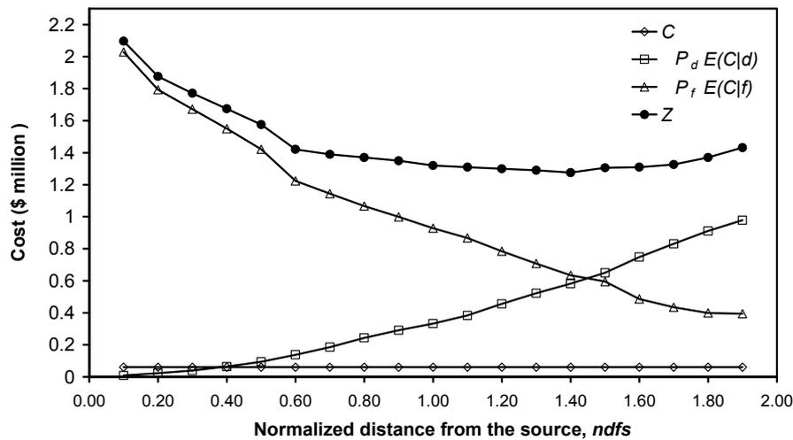
Figure 5.6: Cost values as a function of normalized distance from the source  $ndfs$  for a single row monitoring system with 3 wells ( $nws=0.33$ ).
