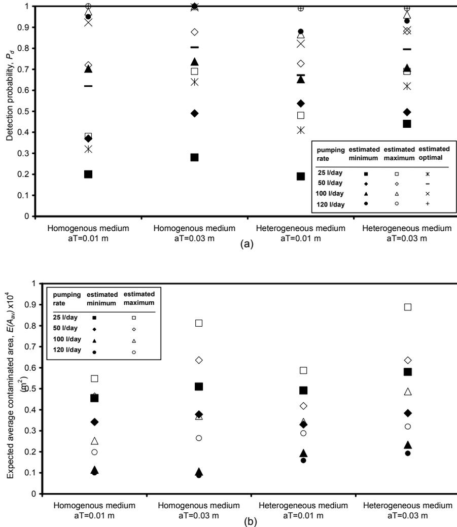
Figure 6.6: Influence of the pumping rate on (a) detection probability  $P_d$  of a 3-well system and (b) expected average contaminated area  $E(A_{av})$ .
