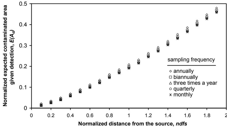
Figure 5.14: Normalized expected contaminated area given detection  $E(A_d)$  as a function of normalized distance from the source  $ndfs$  for a single row monitoring system with 3 wells ( $nws = 0.33$ ) for different sampling frequencies.
