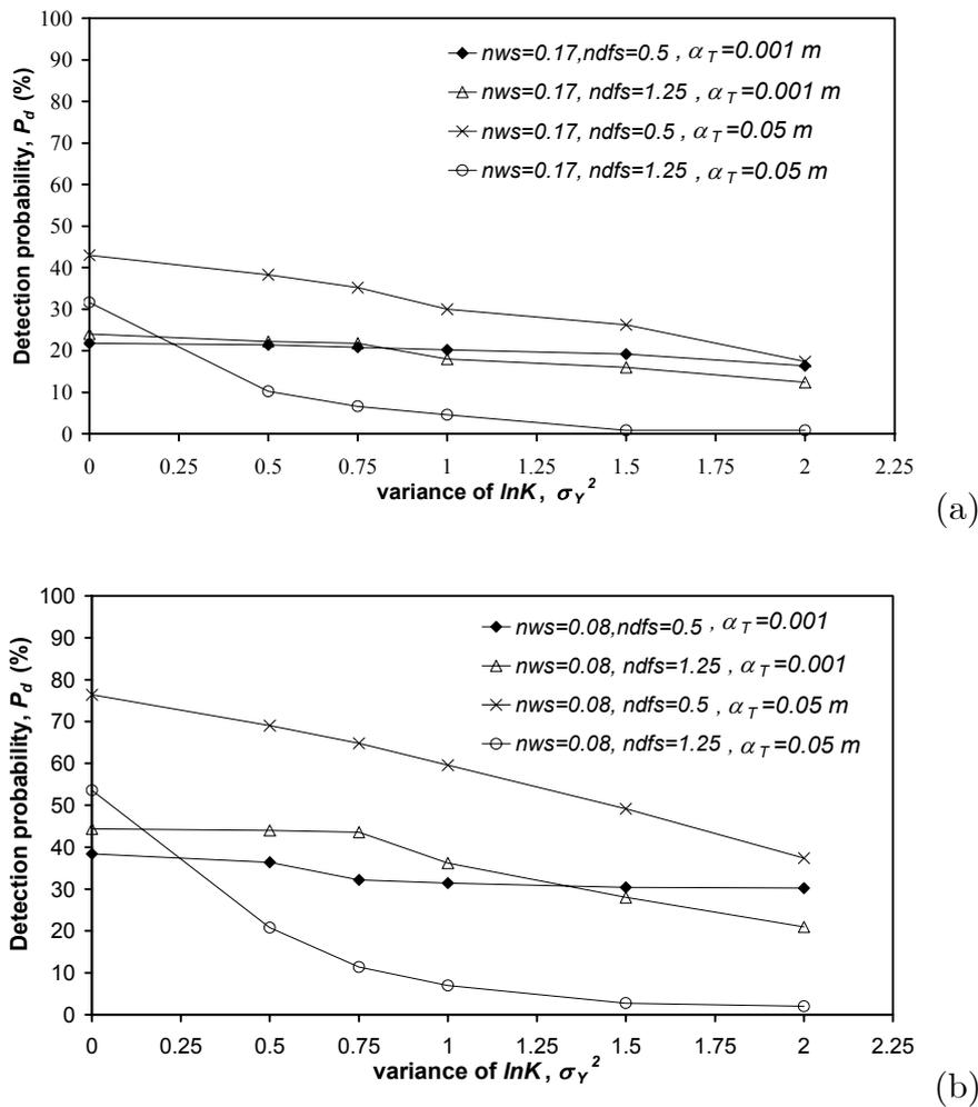
Figure 4.8: Detection probability,  $P_d$  as a function of variance of  $Y$ ,  $\sigma_Y^2$  for a monitoring well system, with a normalized well spacing,  $nws$  of (a) 0.17 and (b) 0.08, for normalized distance from the source,  $ndfs=0.50$  and  $ndfs=1.25$ , where transverse dispersivity,  $\alpha_T$  is equal to 0.001 m and 0.05 m, respectively.
