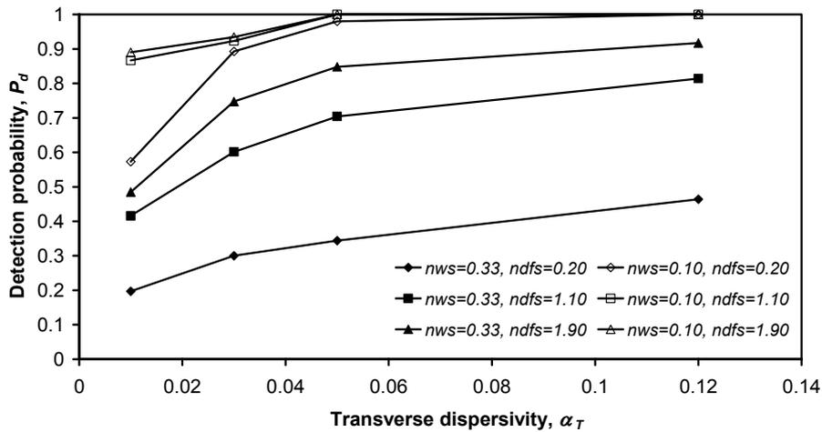
Figure 5.10: Detection probability  $P_d$  as a function of transverse dispersivity  $\alpha_T$ , for selected single row monitoring systems.
