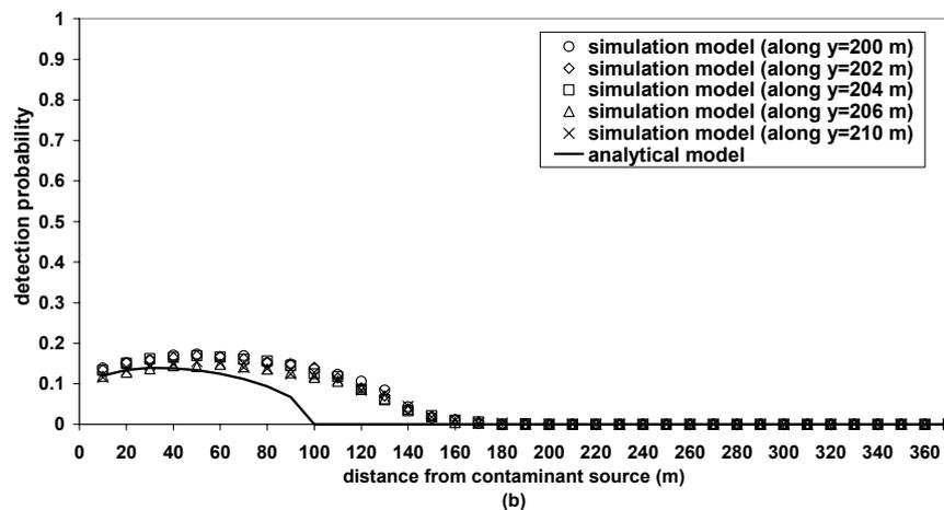
Figure 3.4: Comparison of detection probability values at selected well locations computed by simulation and analytical models for an instantaneous leak in the homogeneous case (a)  $\alpha_L=0.1$  m,  $\alpha_T=0.01$  m and (b)  $\alpha_L=0.5$  m,  $\alpha_T=0.05$  m.
