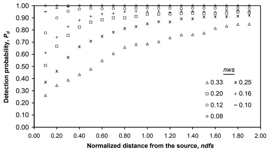
Figure 5.3: Detection probability,  $P_d$  as a function of normalized distance from the source  $ndfs$  for single row monitoring systems with different normalized well spacing  $nws$ .
