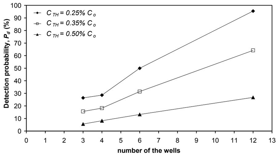
Figure 4.4: Detection probability of monitoring networks in a homogenous and highly dispersive ( $\alpha_L=2$  m,  $\alpha_T=2$  m) medium, for three different concentration threshold values.
