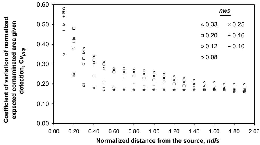
Figure 5.5: Coefficient of variation of expected contaminated area given detection  $CV_{A(d)}$  as a function of normalized distance from the source  $ndfs$  for single row monitoring systems with different normalized well spacing  $nws$ .
