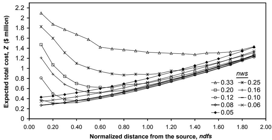
Figure 5.7: Expected total cost,  $Z$  as a function of normalized distance from the source  $ndfs$  for single row monitoring systems with different normalized well spacing  $nws$ .
