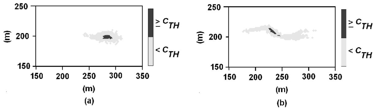
Figure 4.5: Single realization of a plume in homogenous medium a) transverse dispersivity,  $\alpha_T=0.2$  m b) transverse dispersivity,  $\alpha_T=0.1$  m.
