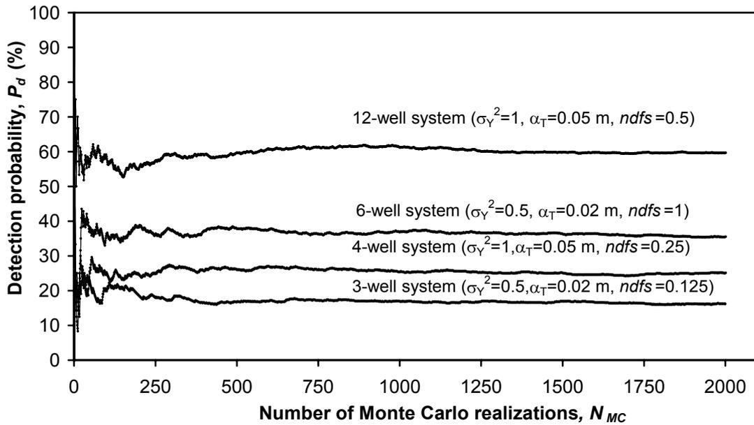
Figure 4.2: Detection probability,  $P_d$  as a function of number of Monte Carlo realizations,  $N_{MC}$  for different monitoring systems.
