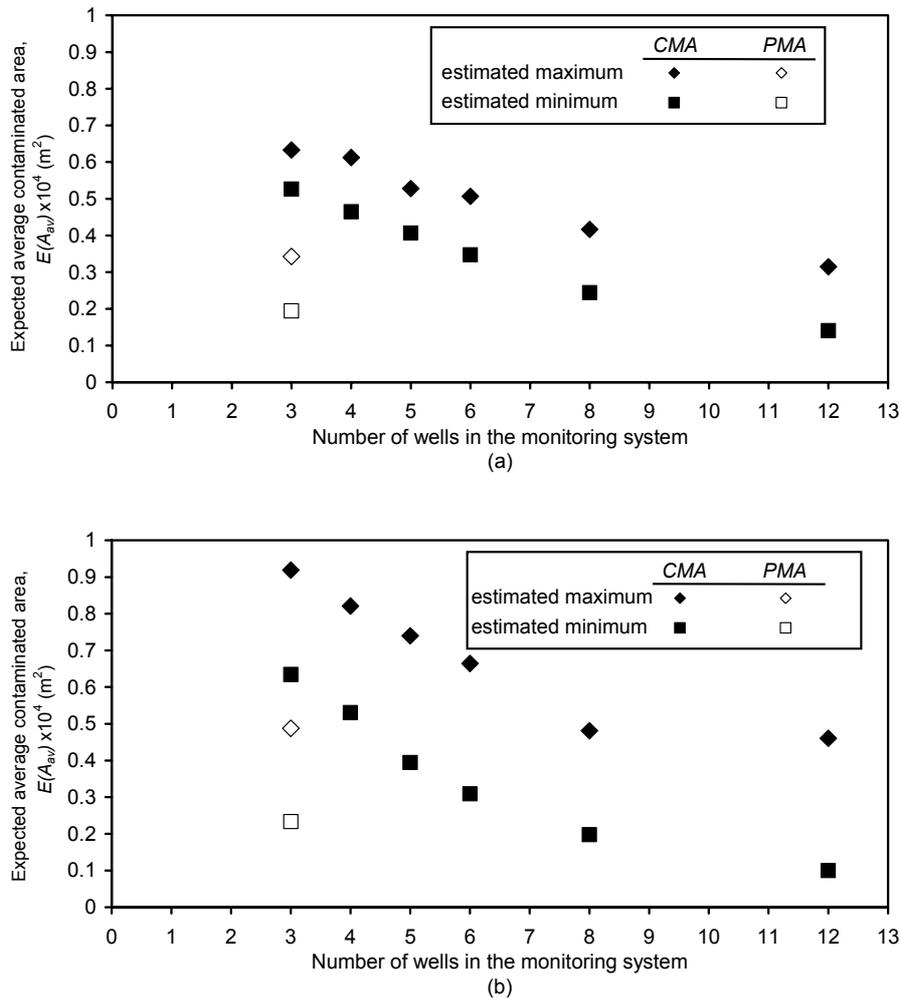
Figure 6.10: Comparison of the conventional monitoring approach (*CMA*) and the proposed monitoring approach (*PMA*) (pumping rate = 100 l/day) in terms of the expected average contaminated area  $E(A_{av})$  “in heterogeneous medium”: (a) transverse dispersivity,  $\alpha_T = 0.01$  m and (b) transverse dispersivity,  $\alpha_T = 0.03$  m.
