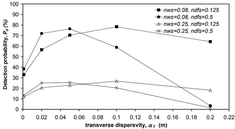
Figure 4.7: Detection probability,  $P_d$  as a function of transverse dispersivity,  $\alpha_T$  in a homogeneous media, for monitoring systems with normalized well spacing,  $nws=0.08$  and  $nws=0.25$ .
