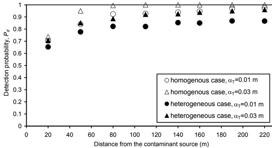
Figure 6.4: System reliability as a function of distance from the source for a 3-well monitoring system for the proposed monitoring approach (*PMA*) (pumping rate is 100 l/day).
