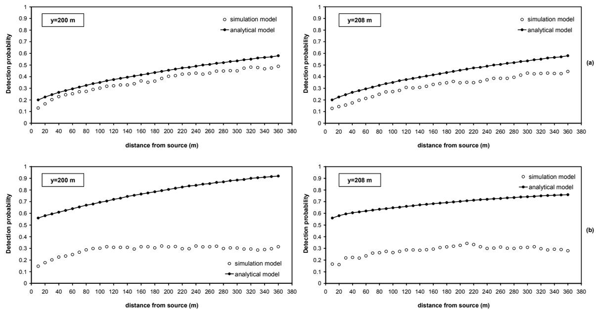
Figure 3.11: Comparison of detection probability values at selected well locations computed by simulation and analytical models for continuous leak in a heterogeneous medium along  $y=200$  m (left column) and  $y =208$  m (right column) (a) Case 1a, and (b) Case 1d.
