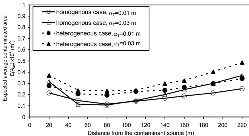
Figure 6.5: Expected average contaminated area  $E(A_{av})$  as a function of distance from the source for a 3-well monitoring system for the proposed monitoring approach (*PMA*) (pumping rate is 100 l/day).
