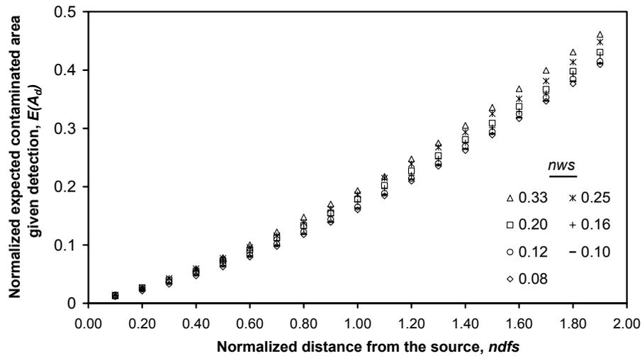
Figure 5.4: Normalized expected contaminated area given detection  $E(A_d)$  as a function of normalized distance from the source  $ndfs$  for single row monitoring systems with different normalized well spacing  $nws$ .
