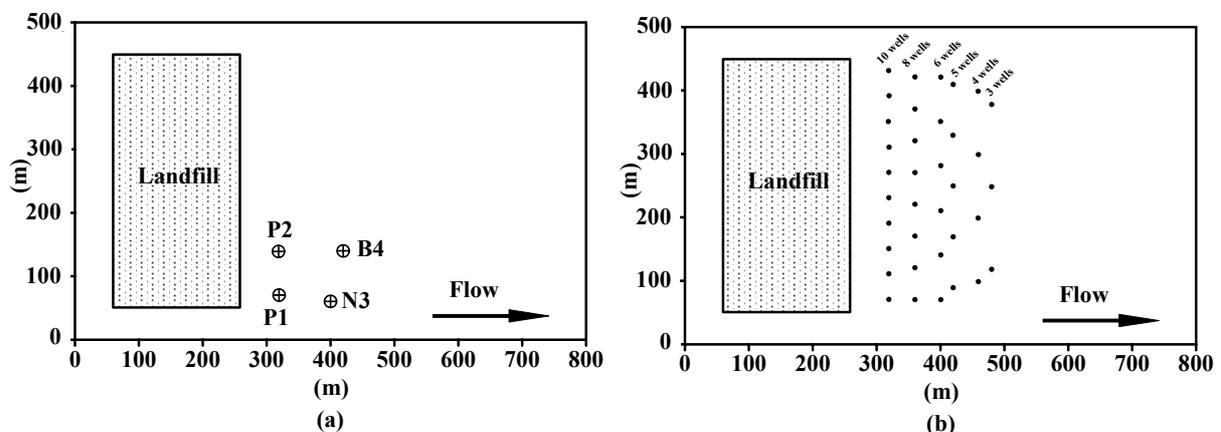
Figure 7.3: Discretized Maarsbergen Landfill model domain (a) with existing detection monitoring system, and (b) with selected monitoring system alternatives in relation to the landfill.
