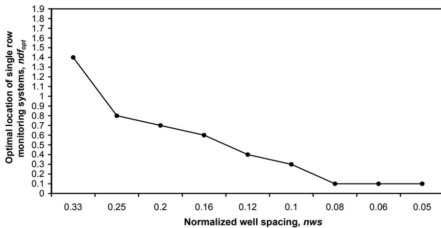
Figure 5.8: Optimal location of single row monitoring systems  $ndfs_{opt}$  as a function of normalized well spacing  $nws$ .
