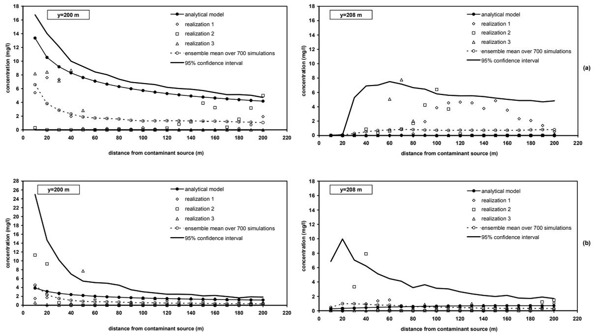
Figure 3.10: Simulation and analytical model comparison of a contaminant plume originated from a continuous leak ( $y=200$  m) in the heterogeneous case for longitudinal sections along  $y=200$  m (left column) and  $y=204$  m (right column) (a) Case 1a, and (b) Case 2d.
