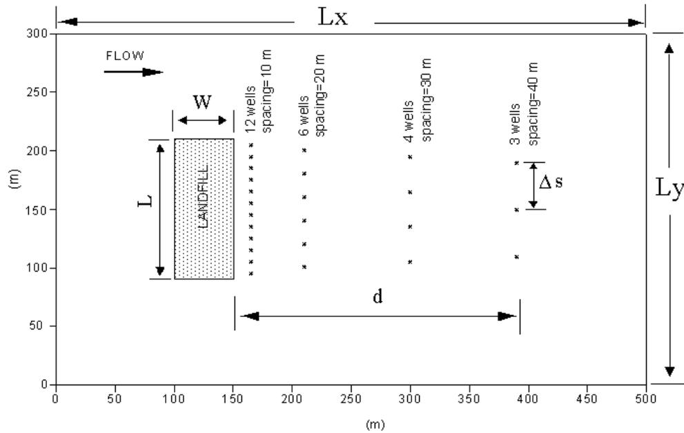
Figure 4.1: Plan view of the hypothetical problem used in numerical experiments.
