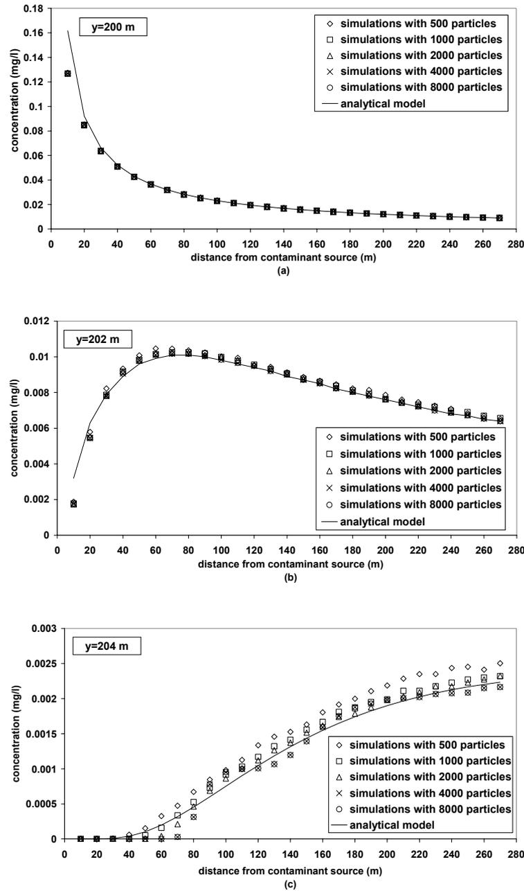
Figure 3.3: Comparison of simulation and analytical model of a contaminant plume originated from an instantaneous leak ( $y=200$  m) in the homogeneous case for  $\alpha_L=0.1$  m,  $\alpha_T=0.01$  m for longitudinal sections along (a)  $y=200$  m, (b)  $y=202$  m and (c)  $y=204$  m.
