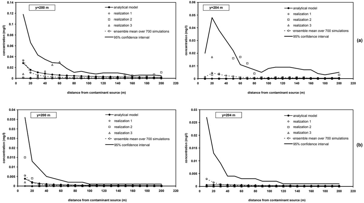
Figure 3.8: Comparison of simulation and analytical model of a contaminant source plume originated from an instantaneous leak ( $y=200$  m) in the heterogeneous case for longitudinal sections along  $y=200$  m (left column) and  $y=204$  m (right column) (a) Case 1a (b) Case 2d.
