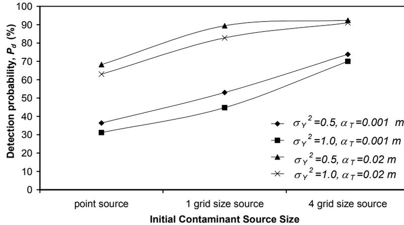
Figure 4.9: Influence of the initial contaminant source size on detection probability,  $P_d$  of a 12-well system, for  $ndfs=0.50$ .
