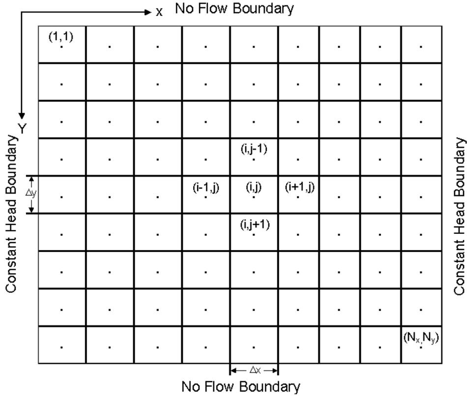
Figure 2.1: 2D finite difference grid discretization with flow boundary conditions (adapted from Kinzelbach, 1986).
