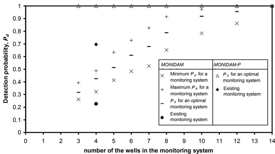
Figure 7.6: Comparison of proposed monitoring systems to existing monitoring system in terms of detection probability,  $P_d$ .
