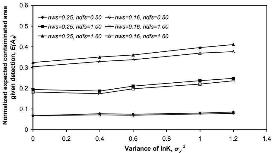
Figure 5.13: Normalized expected contaminated area given detection,  $E(A_d)$  as a function of variance  $\sigma_Y^2$  of  $Y$  for selected single row monitoring systems.
