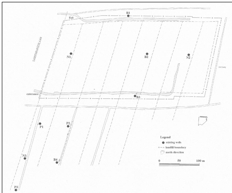
Figure 7.2: Map of the Maarsbergen Landfill site illustrating the main disposal area and existing monitoring wells.
