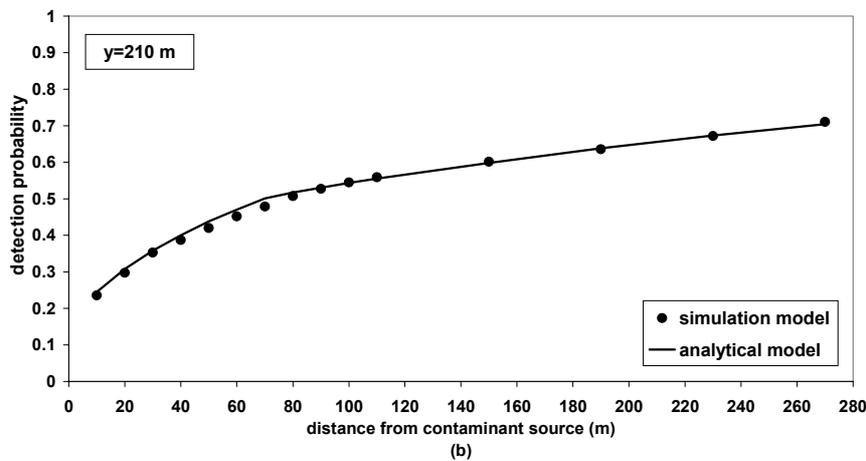
Figure 3.7: Comparison of detection probability values at selected well locations computed by simulation and analytical models for a continuous leak in the homogeneous case ( $\alpha_L=0.5$  m,  $\alpha_T=0.05$  m) (a) along  $y=200$  m and (b) along  $y=210$  m.
