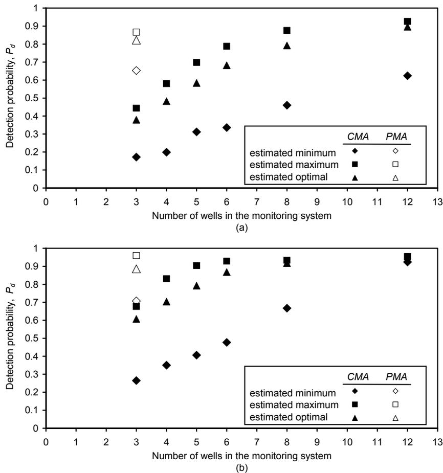
Figure 6.8: Comparison of the conventional monitoring approach (*CMA*) and the proposed monitoring approach (*PMA*) (pumping rate=100 l/day) in terms of reliability “in heterogeneous medium”: (a) transverse dispersivity,  $\alpha_T=0.01$  m, (b) transverse dispersivity,  $\alpha_T=0.03$  m.
