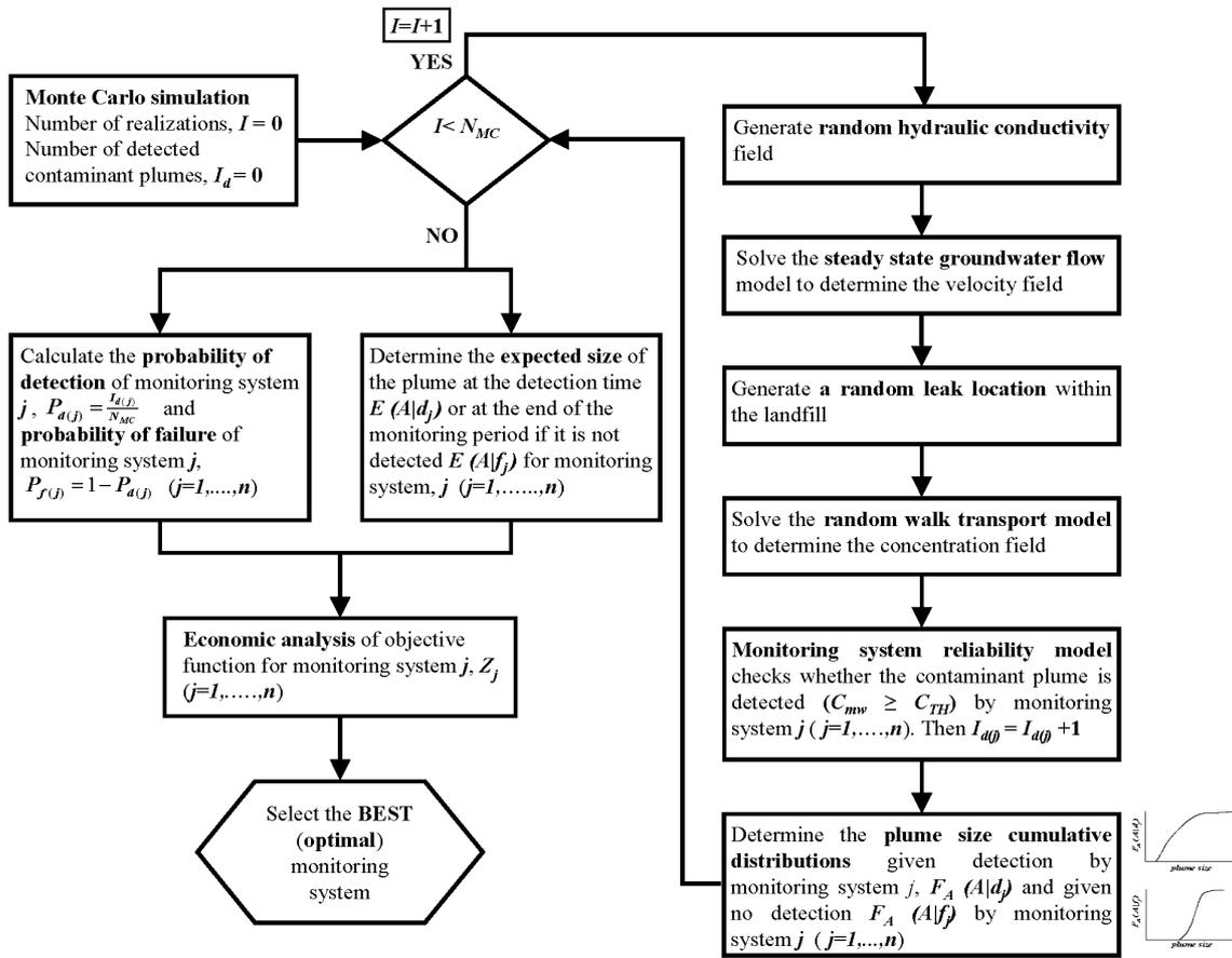
Figure 5.1: Flow chart illustrating the structure of the decision model *MONIDAM*
