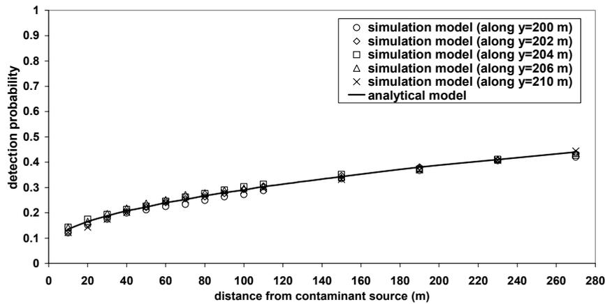
Figure 3.6: Comparison of detection probability values at selected well locations computed by simulation and analytical models for a continuous leak in the homogeneous case ( $\alpha_L=0.1$  m,  $\alpha_T=0.01$  m).
