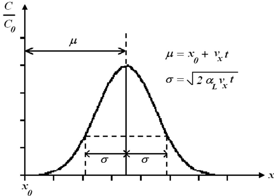
Figure 2.2: Solution of the transport equation in one dimension viewed as normal distribution (after Kinzelbach, 1986).
