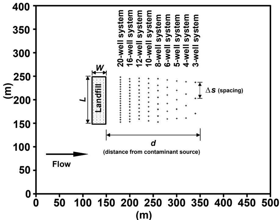
Figure 5.2: Dimensions and components of example problem used in numerical experiments. (Note: the spacing between the first (or last) well and the  $y=150$  m (respectively  $y=250$  m) line equals to  $\Delta s/2$  and each monitoring system (i.e., with a fixed number of monitoring wells) is located at a different distance from the landfill which result in 171 potential monitoring system alternatives).
