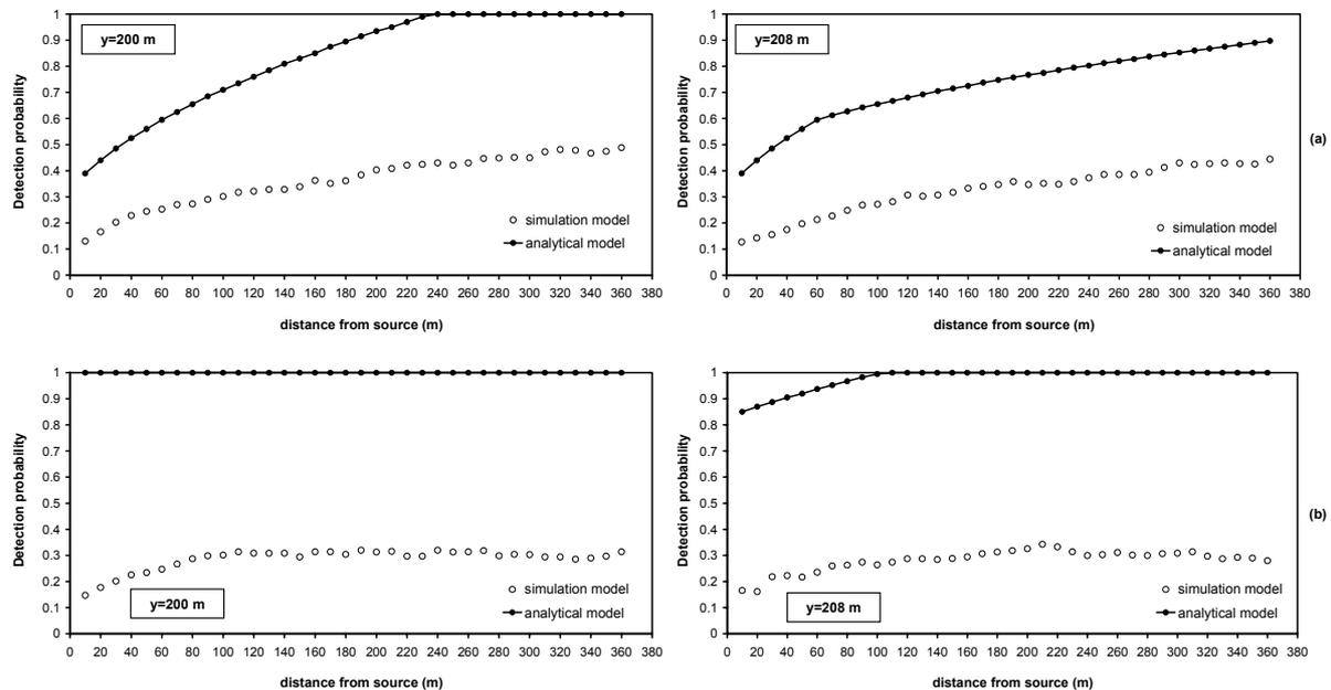
Figure 3.12: Comparison of detection probability values at selected well locations computed by simulation and analytical models for continuous leak in a heterogeneous medium along  $y=200$  m (left column) and  $y =208$  m (right column) (a) Case 2a, and (b) Case 2d.
