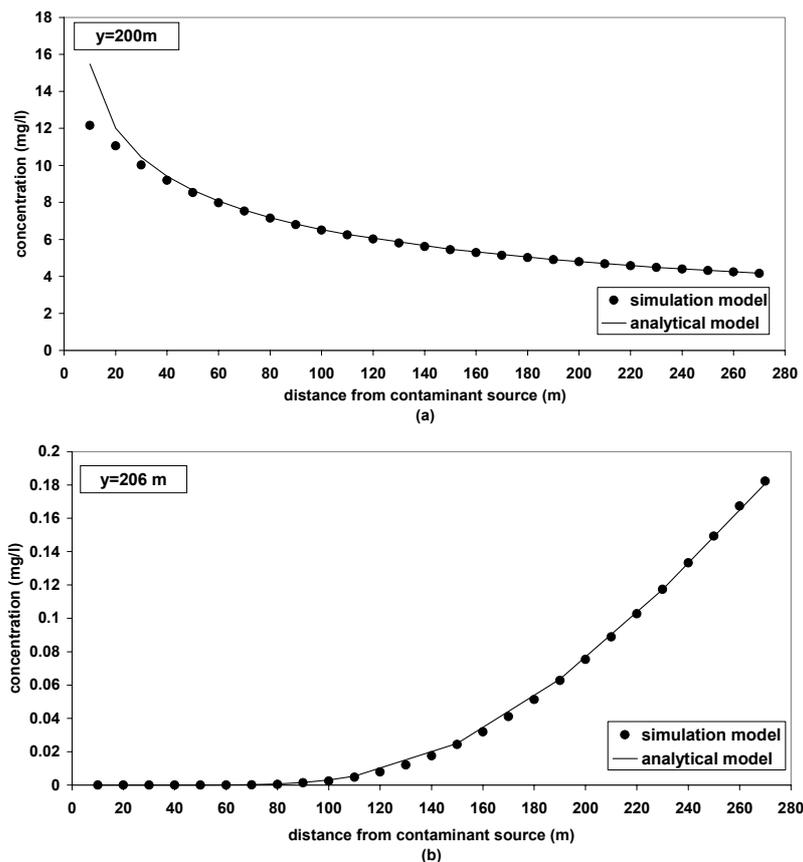
Figure 3.5: Comparison of simulation and analytical model of a contaminant plume originated from a continuous leak in the homogeneous case with  $\alpha_L=0.1$  m,  $\alpha_T=0.01$  m for longitudinal sections along (a)  $y=200$  m and (b)  $y=206$  m.
