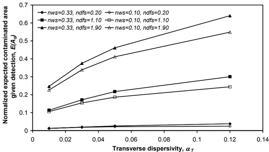
Figure 5.11: Normalized expected contaminated area given detection  $E(A_d)$  as a function of transverse dispersivity  $\alpha_T$ , for selected single row monitoring systems.
