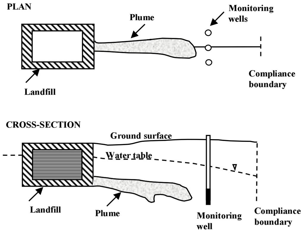
Figure 1.1: Groundwater contamination scenario (after Massmann and Freeze, 1987a).
