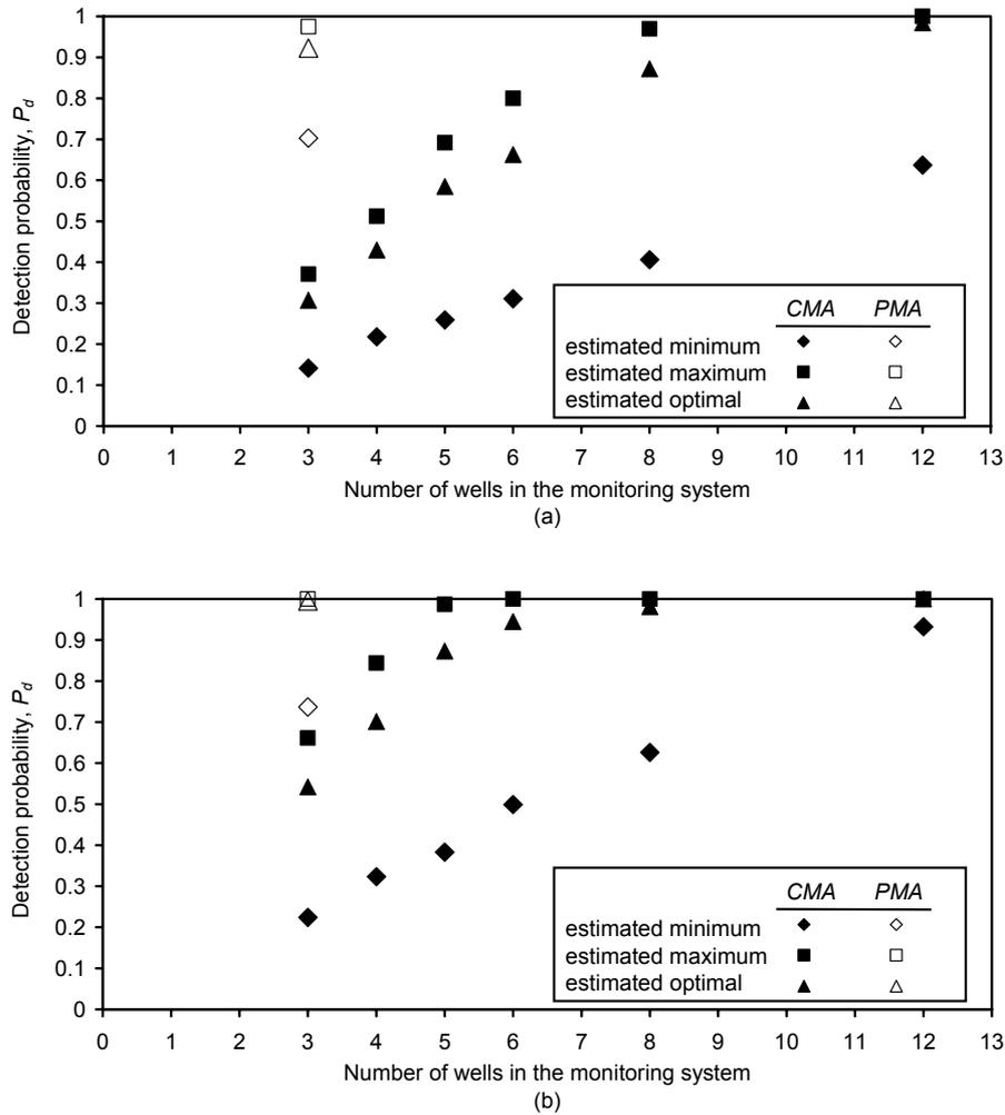
Figure 6.7: Comparison of the conventional monitoring approach (*CMA*) and the proposed monitoring approach (*PMA*) (pumping rate=100 l/day) in terms of reliability “in homogeneous medium”: (a) transverse dispersivity,  $\alpha_T=0.01$  m, and (b) transverse dispersivity,  $\alpha_T=0.03$  m.
