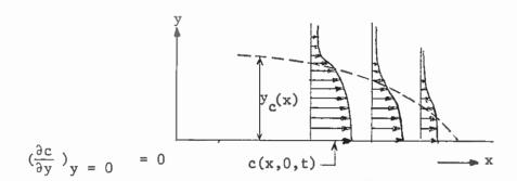
Denote y (x) as some measure of the salt wedge thickness
