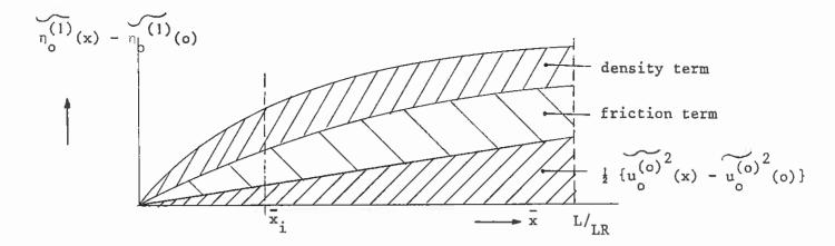
The region  $0 < x < x_i$  is the region of salt intrusion, where not enough information is available to determine the mean water level. Note that the slope of the waterlevel due to the tidal waves is an order of magnitude higher than the slope in waterlevel due to the discharge alone. The contribution of the latter does not appear in this order of approximation.
