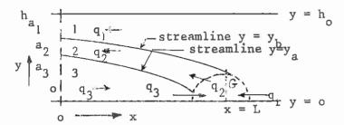
The fluid domain bounded by the bottom of the flume and the watersurface is divided into four regions. The regions denoted by 1, 2 and 3 in the above sketch are separated by the streamlines  $y = y_a$  and  $y = y_b$ . Across these lines the normal time mean velocities are zero. The last region G contains the salt wedge tip. The horizontal dimension of region G is small compared to the length of the salt intrusion.
