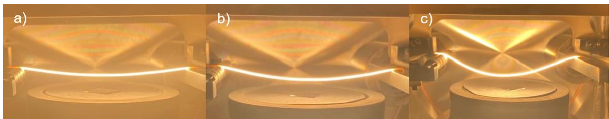
Figure 5.8: Deformation of W filament (exp. D4) after a) 8 h, b) 35 h, and c) 148 h of carburization
