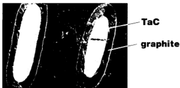
Figure 8.3: SEM micrographs showing the poisoning of Ta filaments after 16 hours of diamond deposition (1.0 vol % CH 4 and 2000 °C) [10]
