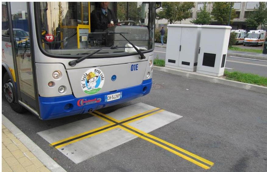
Figure 2-10 - Inductive electric vehicle charging at a bus stop in Torino. Source: Salucci (2015)
