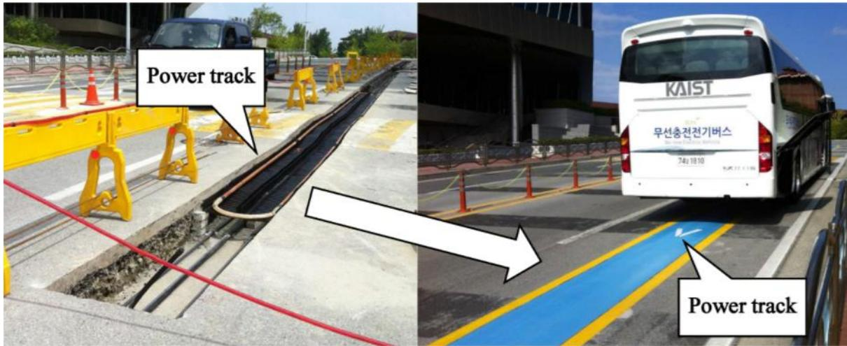
Figure 2-11 - Wireless in motion charged campus shuttle on the KAIST campus, China. Source: Jang et al. (2016)
