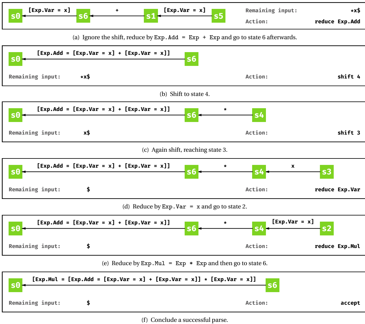
Figure 2.7: LR parsing x+x*x , continuing after the conflict by choosing reduce over shift.
