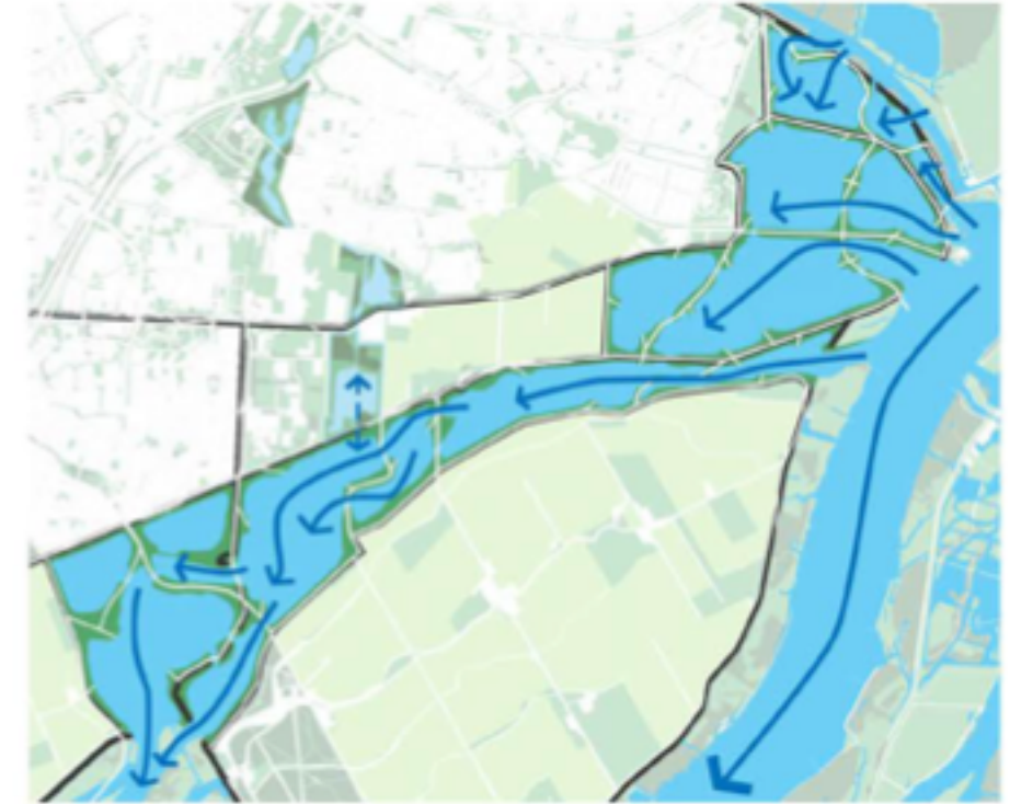
Extreme water condition 300cm above NAP Landscape flooded, lower access roads are flooded leaving vital evacuation access
