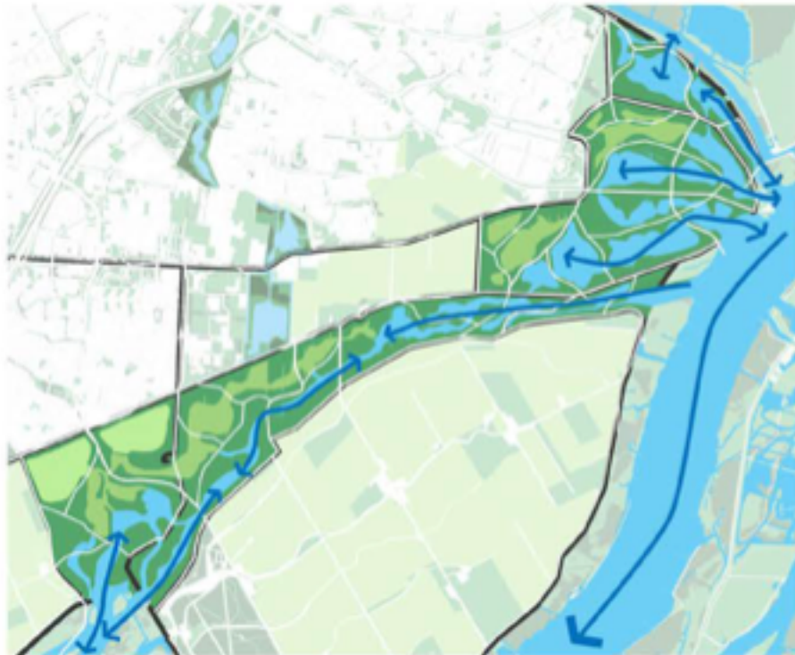
Normal tidal regime <120cm above NAP Water flows in and out of the site, flooding lowest areas of the landscape
