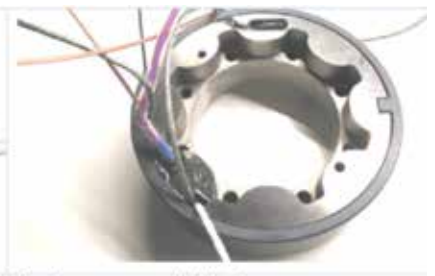
The iBearing sleeve with the sensors embedded.
