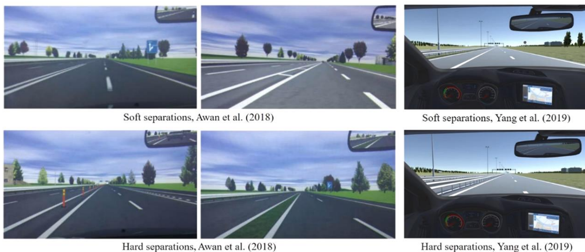
Figure 2-2 Examples of hard and soft separation on managed lanes used in the literature.
