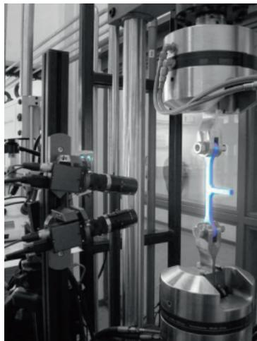
Figure 3.1: Example DIC setup (den Besten, 2015)
