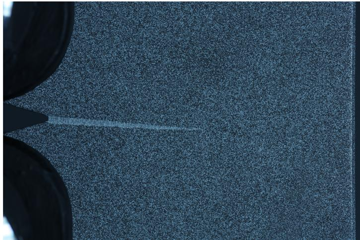
Figure 16.1: Intact paint layer over large crack.
