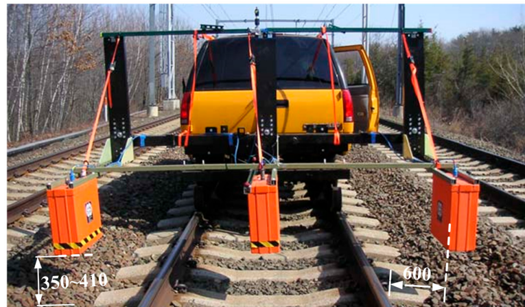
(a) GPR system with carrier (a van)
