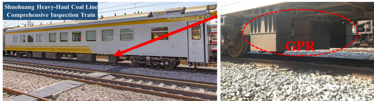
Figure 16. Integrated inspection vehicle with GPR system.
