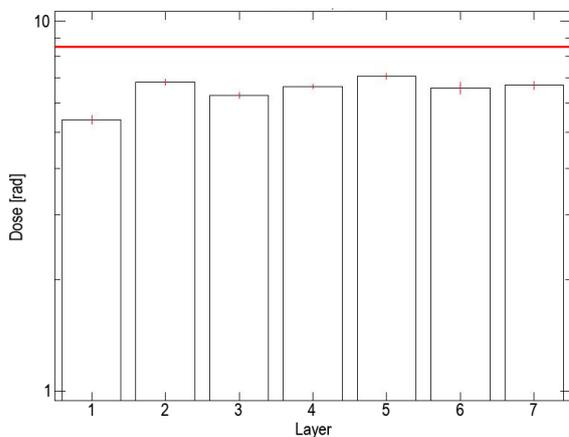
Figure 3.18: Analysis of average dose during GCR for the final soft-shell design.
