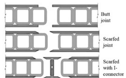
Figure 4.27: Floor panel connection possibilities<sup>[4]</sup>.
