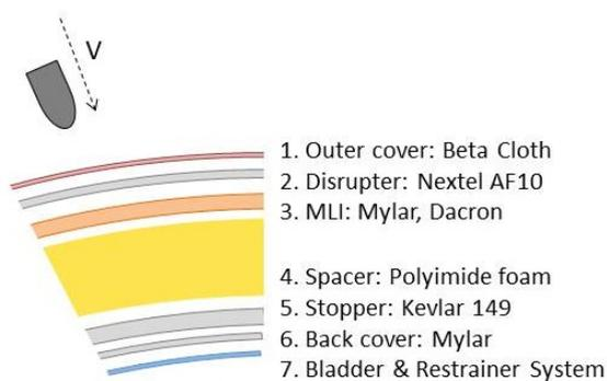
Figure 3.9: Cross section of the inflatable structure: multishock thermal blanket (MTB). The spacing in between the layers are only for visualisation purposes.
