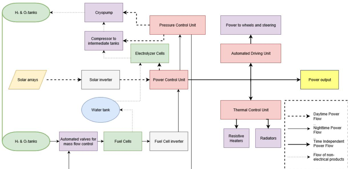
Figure 8.5: Electrical Block Diagram of one power module.
