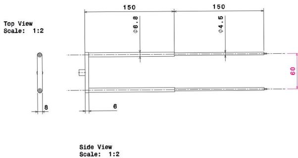
Figure 4.19: Schematic drawing of third iteration of mounting pin (dimensions are given in millimetres).
