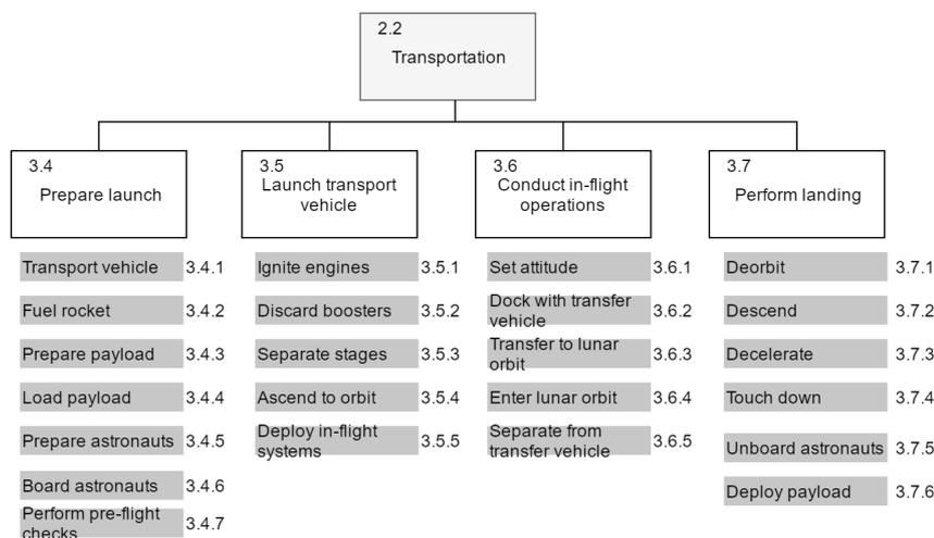
Figure 11.3: Functional Breakdown Structure of Transportation.
