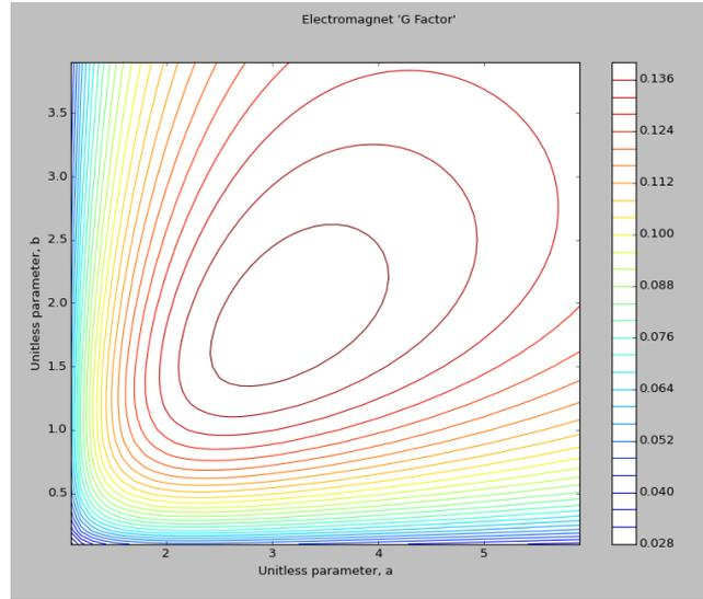
Figure 3.21: Color plot of the G-factor w.r.t. unitless coil dimensions (a,b).
