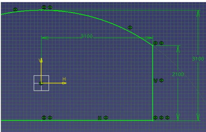
Figure 4.8: Schematic drawing of front cross section of third iteration of hard-shell module.
