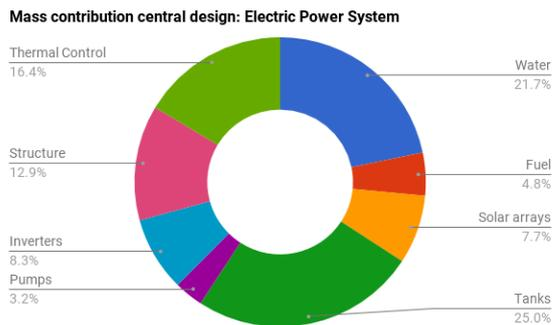
Figure 8.3: Mass contributions of the central power system design.
