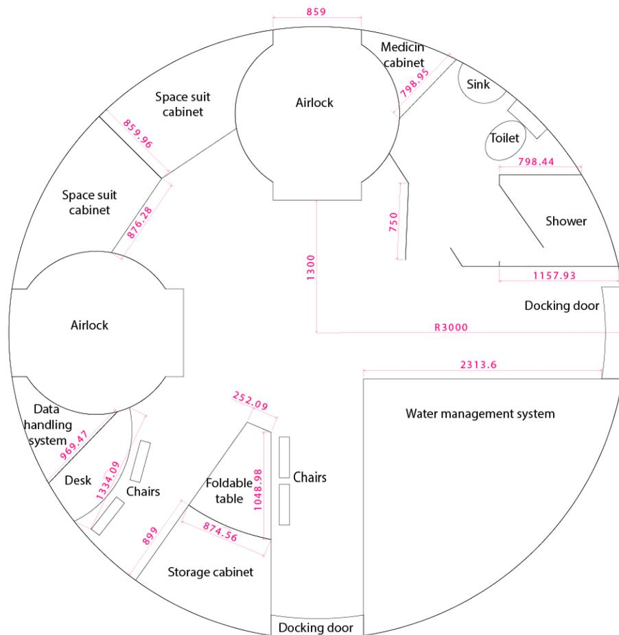
Figure 7.1: The ground plan of the The Shell.
