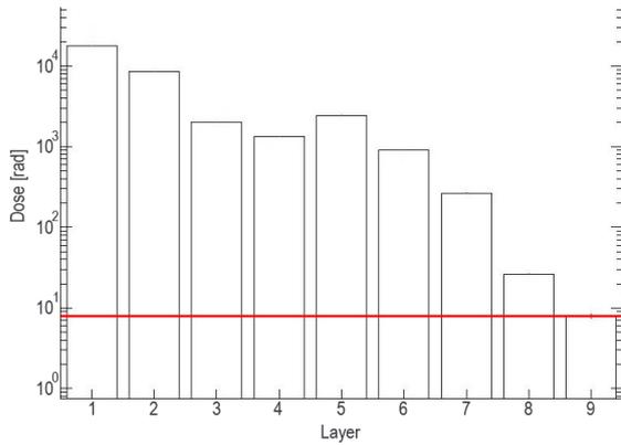
Figure 3.7: Analysis average dose in wall layers during SPEs with a layer of 23.5cm of polyethylene (8).
