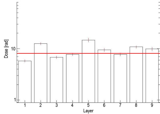
Figure 3.8: Analysis average dose in wall layers during GCR with a layer of 23.5cm of polyethylene (8).
