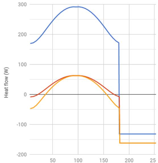
Figure 3.15: Heat flow coming inside or going outside the inflatable. From 180 degrees onwards the heat flow is constant. The blue line is the heat flow with a regolith tunnel of 20 cm thick and without MLI. The yellow and red lines are the heat flow for the inflatables with 29 layers of MLI.
