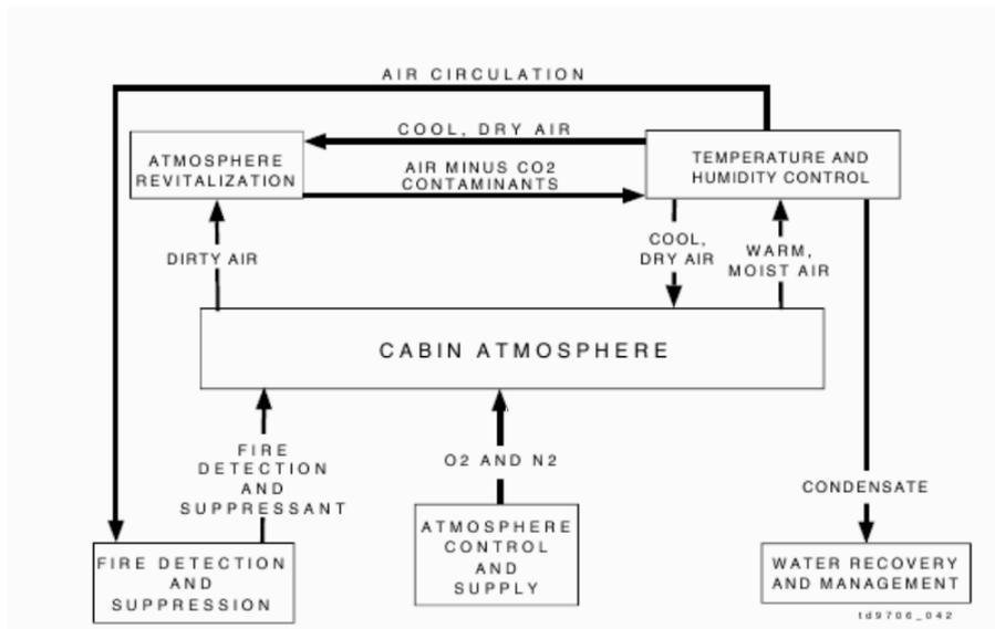
Figure 3.25: Atmospheric control system interfaces [24].
