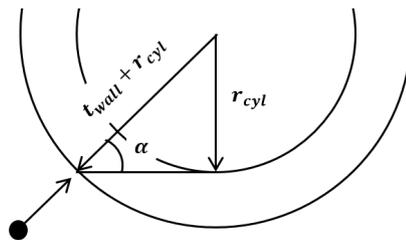
Figure 3.20: Minimal deflection angle ( $\alpha$ ) proton moving through habitat wall.
