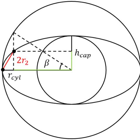
Figure 3.23: Angle, distance relations for equally distanced points on an ellipses.
