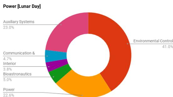
Figure 8.1: Power demand contribution of each subsystem during the lunar illumination time.
