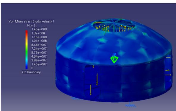
Figure 4.10: Structural analysis results for third iteration of hard-shell module generated in CATIA.
