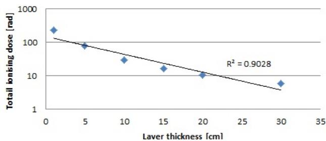
Figure 3.6: Dose analysis for different thicknesses of polyethylene
