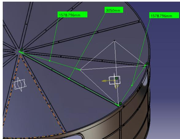
Figure 4.22: Different viewing angle of schematic demonstration of the construction of tetrahedral support system for the hard-shell module. Dimensions were measured in CATIA.
