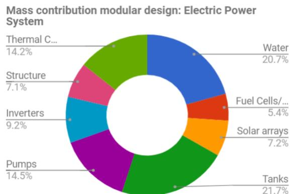
Figure 9.2: Mass composition of one modular power supplier: the Power Ranger.
