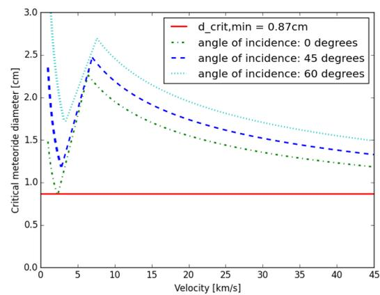
Figure 3.11: LEAP Blanket meeting minimum requirements:  $d_{crit,min}=0.87\text{cm}$ . Amount of layers: Disrupter (24), Spacer (24), Stopper (48).
