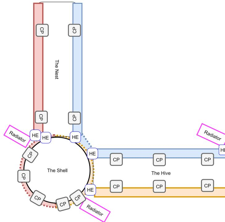
Figure 3.24: Layout Active thermal control. Dotted line means ammonia loop and continues line is water loop.
