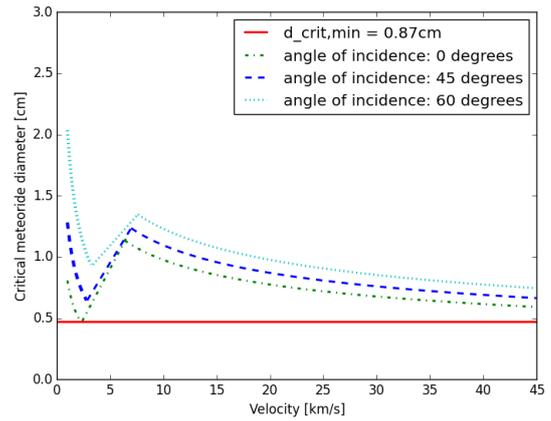
Figure 3.13: LEAP Blanket using lunar regolith meeting minimum requirements:  $d_{crit,min}=0.47\text{cm}$ . Amount of layers: Disrupter (15), Spacer (12), Stopper (24).
