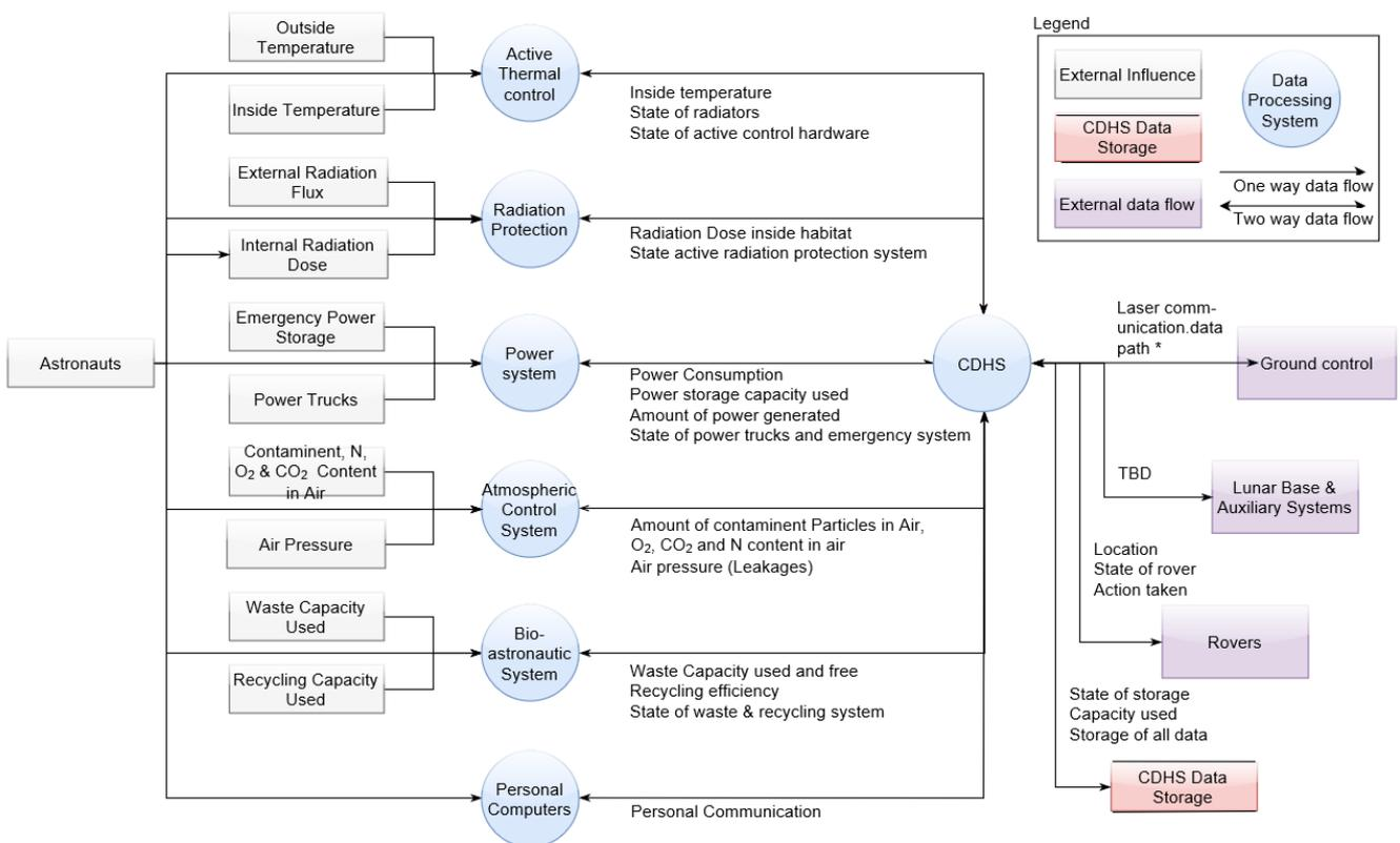
Figure 6.1: Data flow of LEAP. The detailed communication data path can be found in section 6.2.
