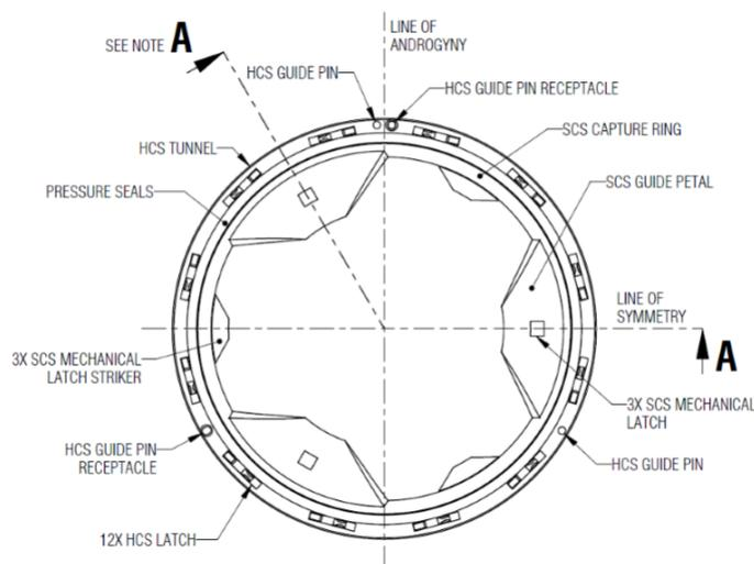
Figure 11.8: Axial view docking interface international standard docking system [54].
