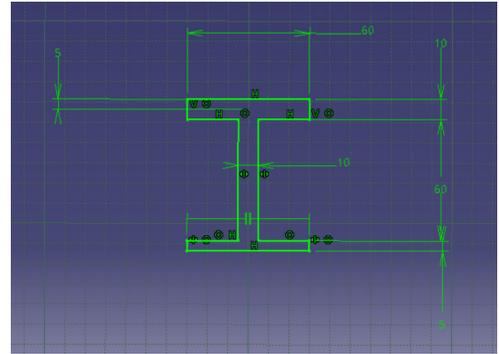
Figure 4.5: Sketch of I-beam (spar) cross section
