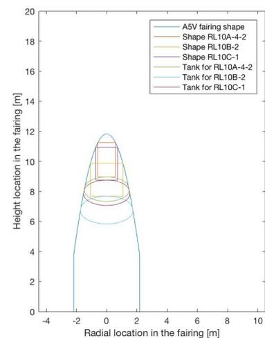
Figure 10.4: Fitting of the lander into the A5V.
