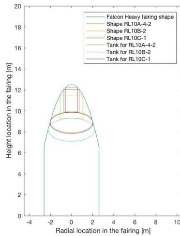
Figure 10.3: Fitting of the lander into the SLS.
