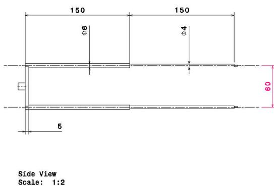
Figure 4.17: Schematic drawing of second iteration of mounting pin (dimensions are given in millimetres).
