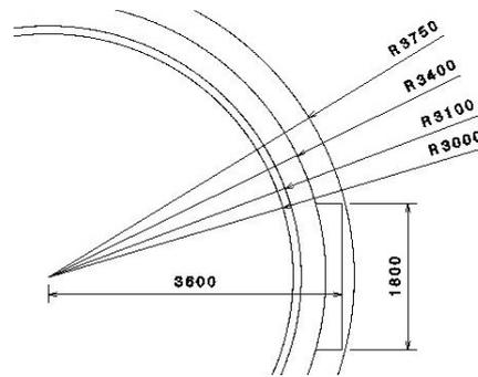
Figure 4.1: Schematic drawing of the sizing of the wall spacing for the hard-shell module. From inner to outer the layers are inner wall, pressure shell and rear wall of Whipple shield, bumper plate of Whipple shield and inner wall of SLS payload bay. The rectangular part represents the airlock and docking system.
