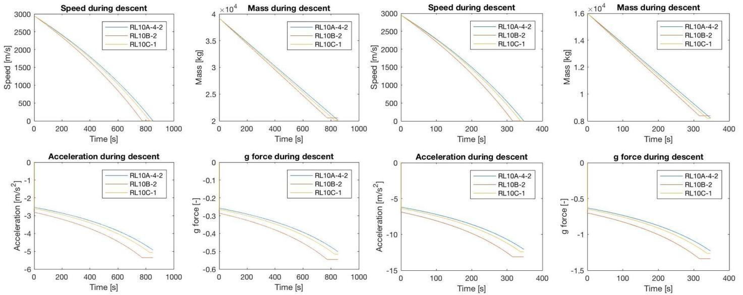
Figure 10.6: Loads during the deceleration of the SLS payload.
