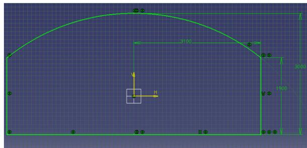
Figure 4.2: Schematic drawing of front cross section of first iteration of hard-shell module.
