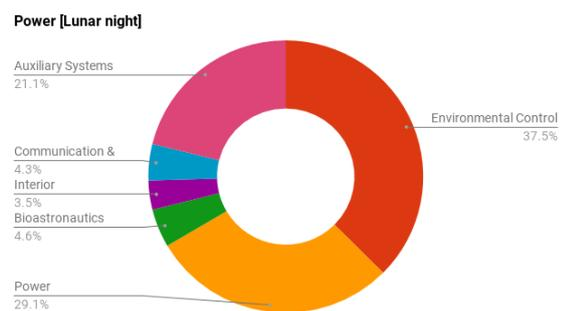
Figure 8.2: Power demand contribution of each subsystem during the lunar night.
