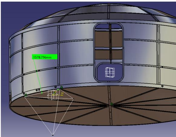
Figure 4.21: Schematic demonstration of the construction of tetrahedral support system for the hard-shell module. Eventually all sketch lines will be beams with adjustable length, to alter the attitude of the hard-shell structure to ease the docking of the inflatable modules.
