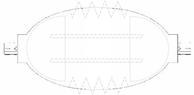
Figure 4.26: Impression of the folded structure. The sized are dependent on folding capabilities of the material and the folding pattern.
