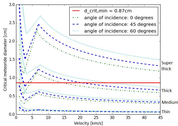
Figure 3.10: Meteorite shielding properties of several toughened several blankets. \*Thin and medium thermal blanket configuration taken from [13], Thick and super thick blankets: proposed configurations.
