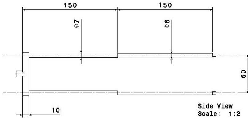
Figure 4.14: Schematic drawing of pin designed to mount the meteorite shield onto the pressure shell. The thicknesses and diameters are guesstimates and will be iterated further after the analysis of the load case (dimensions are given in millimetres).
