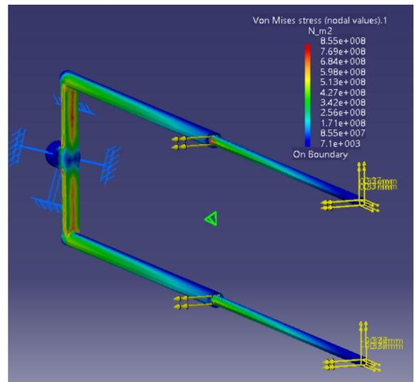
Figure 4.18: Structural analysis results for second iteration of mounting pin generated in CATIA. It can be observed that the pin is now under-designed.
