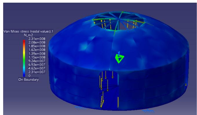
Figure 4.7: Structural analysis results for second iteration of hard-shell module generated in CATIA.
