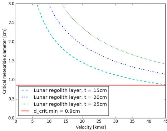
Figure 3.12: Meteorite shielding properties of lunar regolith: critical meteorite diameter of the projectile in centimetre as a function of projectile velocity in km/s.
