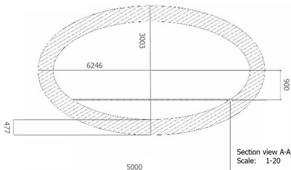
Figure 4.23: Front view of the inflatable structure.
