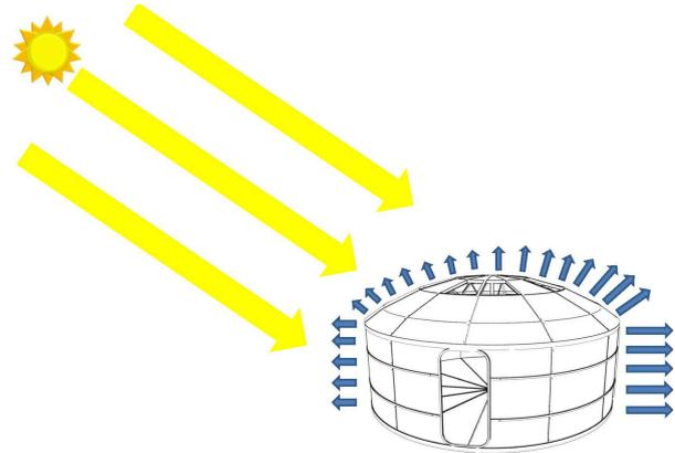
Figure 3.4: Heat rejection from the habitat (not to scale).
