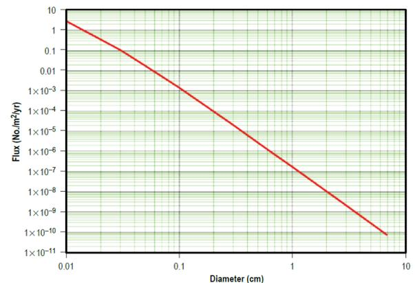
Figure 3.2: Meteorite impact flux near the Moon as a function of particle size (sizes were computed assuming a density of  $1\text{g/cm}^3$ ) [6].
