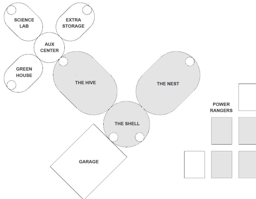
Figure 15.1: Preliminary layout lunar village. Gray parts are existing habitat design. White parts are auxiliary modules to be added. Ground trajectory Sun parallel to vertical axis.
