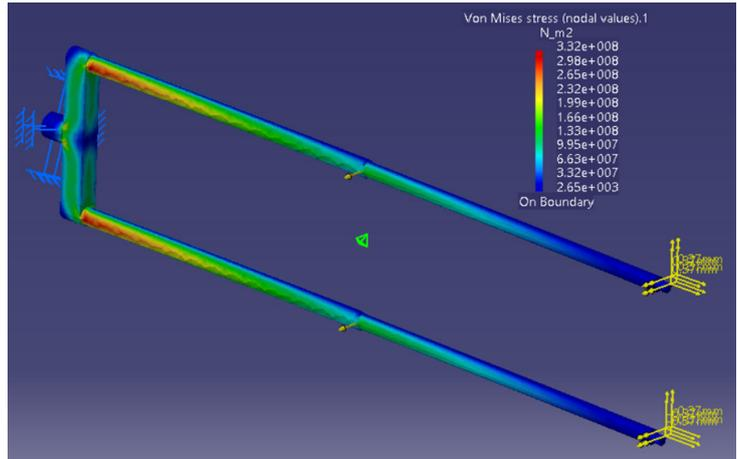
Figure 4.16: Structural analysis results for first iteration of mounting pin generated in CATIA. It can be observed that the pin is still over-designed and that the thicknesses can be reduced.
