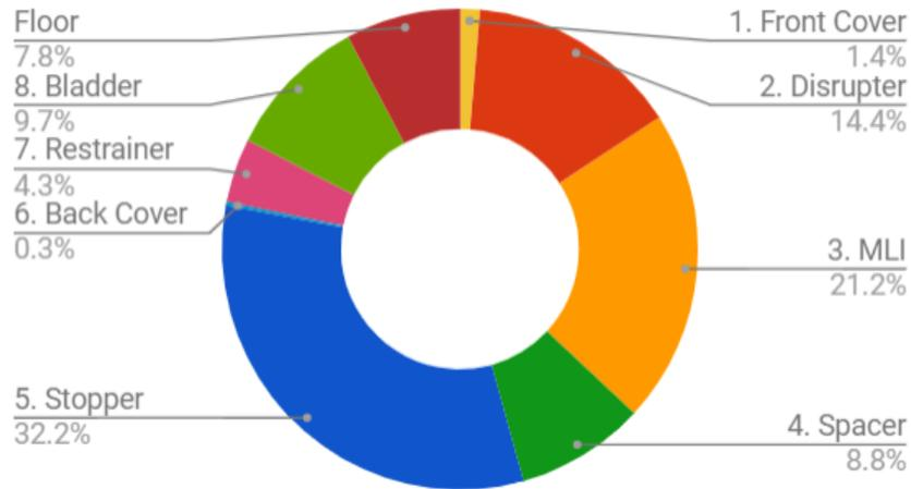
Figure 9.8: Composition of the complete inflatable structure: valid for the Nest and the Hive.
