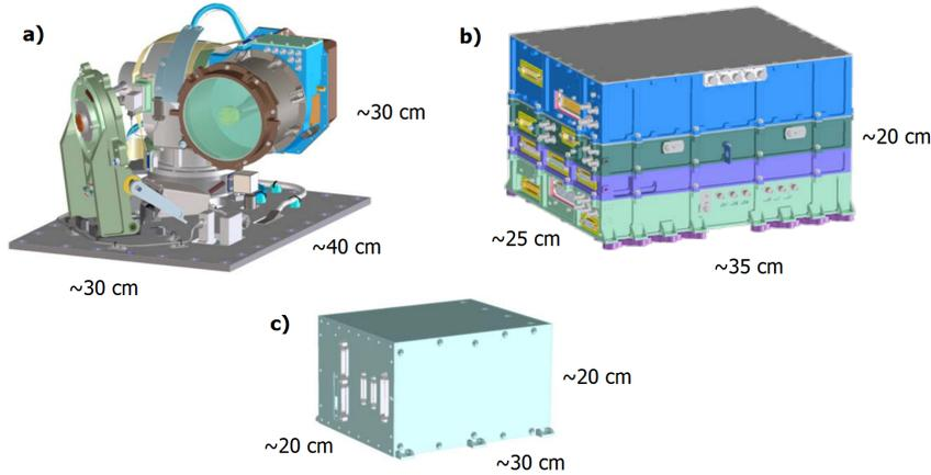
Figure 6.2: Lunar Lasercom Space Terminal. a) optical module, b) modem module, c) controller electronics module.
