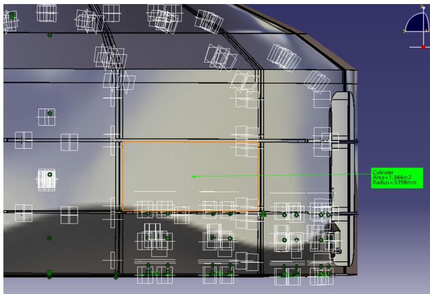
Figure 4.15: CATIA screenshot of hard-shell module with integrated whipple shield panel. The largest shield is highlighted and its data can be found in the green box.
