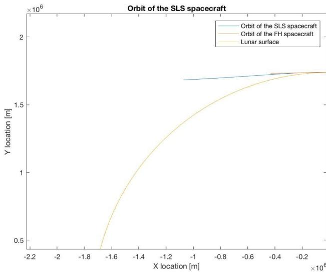
Figure 10.8: Difference in the orbits of the two payloads.
