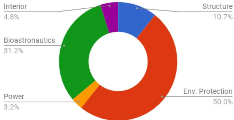
Figure 9.7: Net wet mass composition of the Nest. It consists of the MTB blanket featuring MMOD protection, thermal insulation, a load bearing layer and an airtight atmospheric layer.
