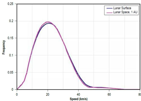
Figure 3.1: Velocity distribution of meteorites on the lunar surface and within the lunar space environment [6].
