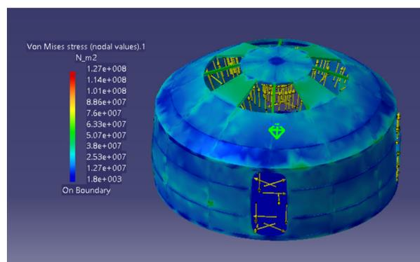
Figure 4.11: Structural analysis results for fourth iteration of hard-shell module generated in CATIA.
