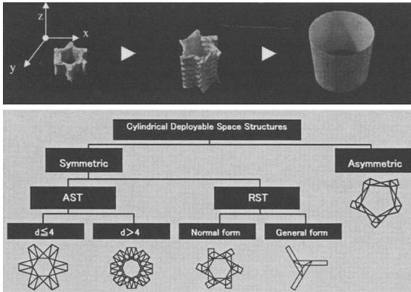
Figure 4.25: Deployment sequence and several folding patterns regarding cylindrical inflatable space structures[29].
