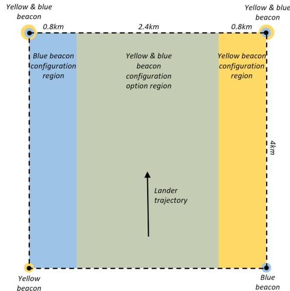
Figure 11.7: Beacon dependencies on target region and lander trajectory.
