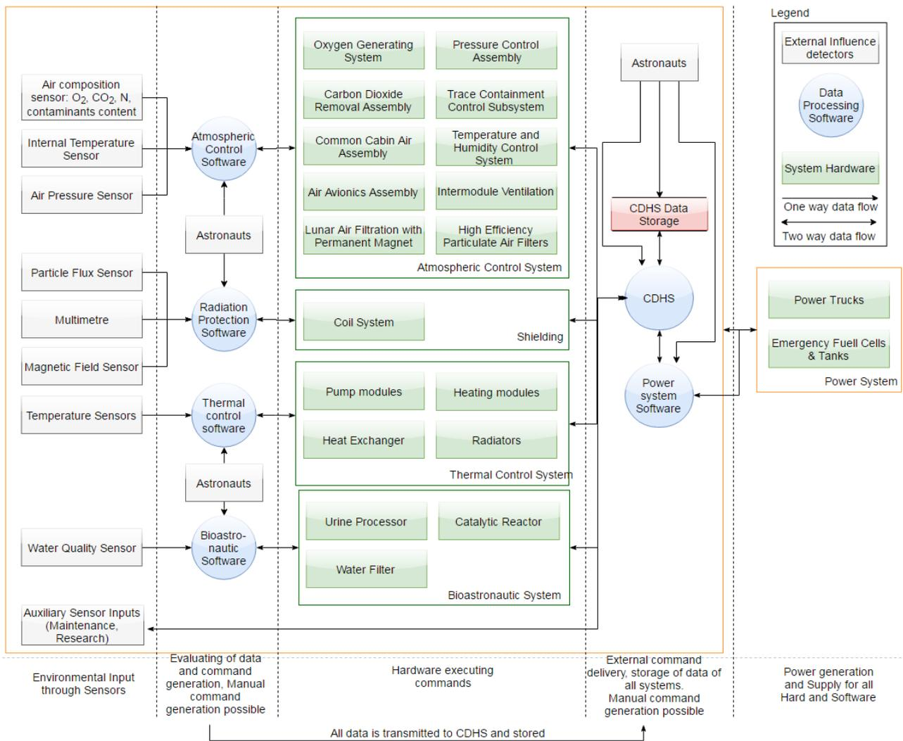
Figure 6.5: Hardware-Software interaction in the habitat system.
