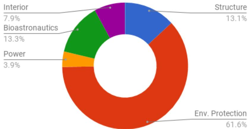
Figure 9.9: Net wet mass composition of the Hive. It consists of the MTB blanket featuring MMOD protection, thermal insulation, a load bearing layer and an airtight atmospheric layer.
