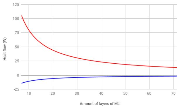
Figure 3.14: Amount of layers MLI against heat flow at certain inclination. Blue line is at night, red line is during the illumination time.
