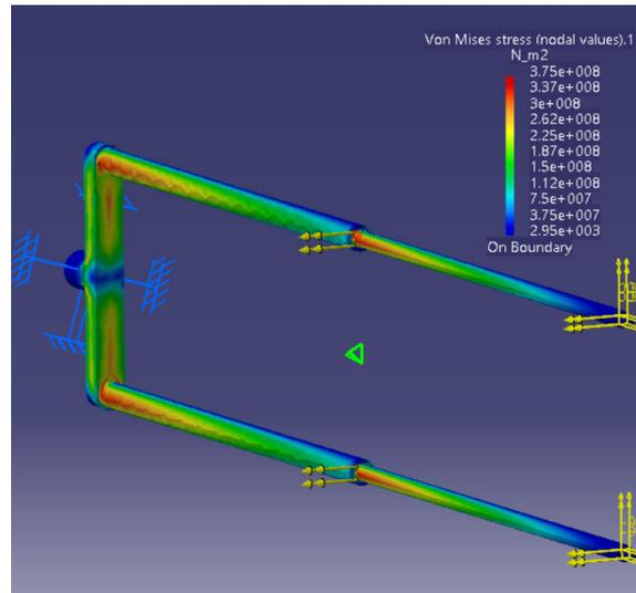
Figure 4.20: Structural analysis results for third iteration of mounting pin generated in CATIA. It can be observed that the pin is now well designed and that the maximum stress comes close to the yield of 393MPa.
