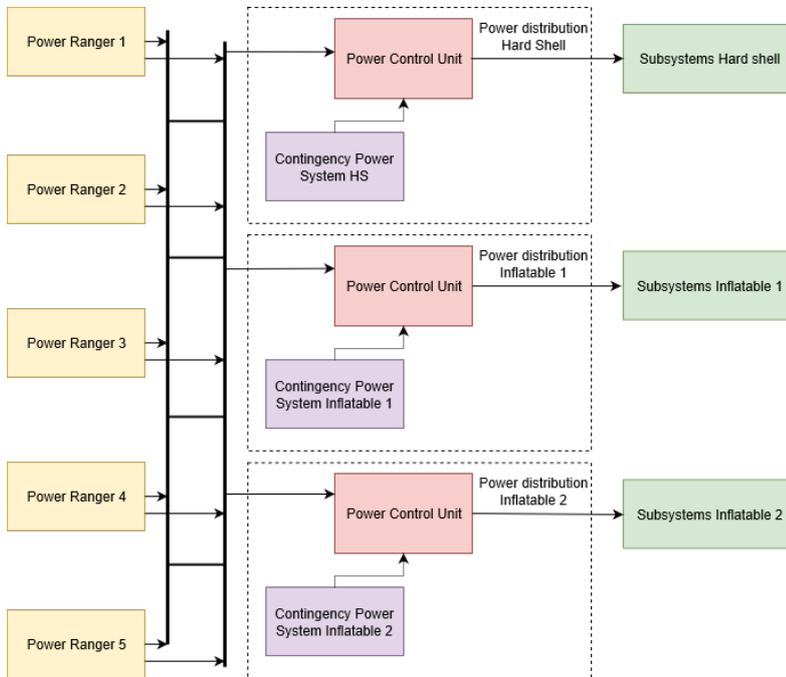
Figure 8.6: Electrical Block Diagram of the habitat.
