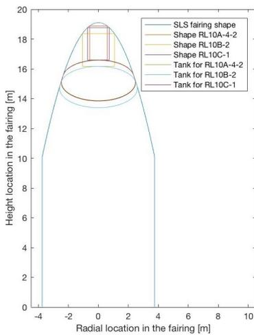
Figure 10.2: Fitting of the lander into the SLS.
