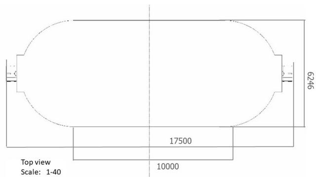
Figure 4.24: Top view of the inflatable structure.
