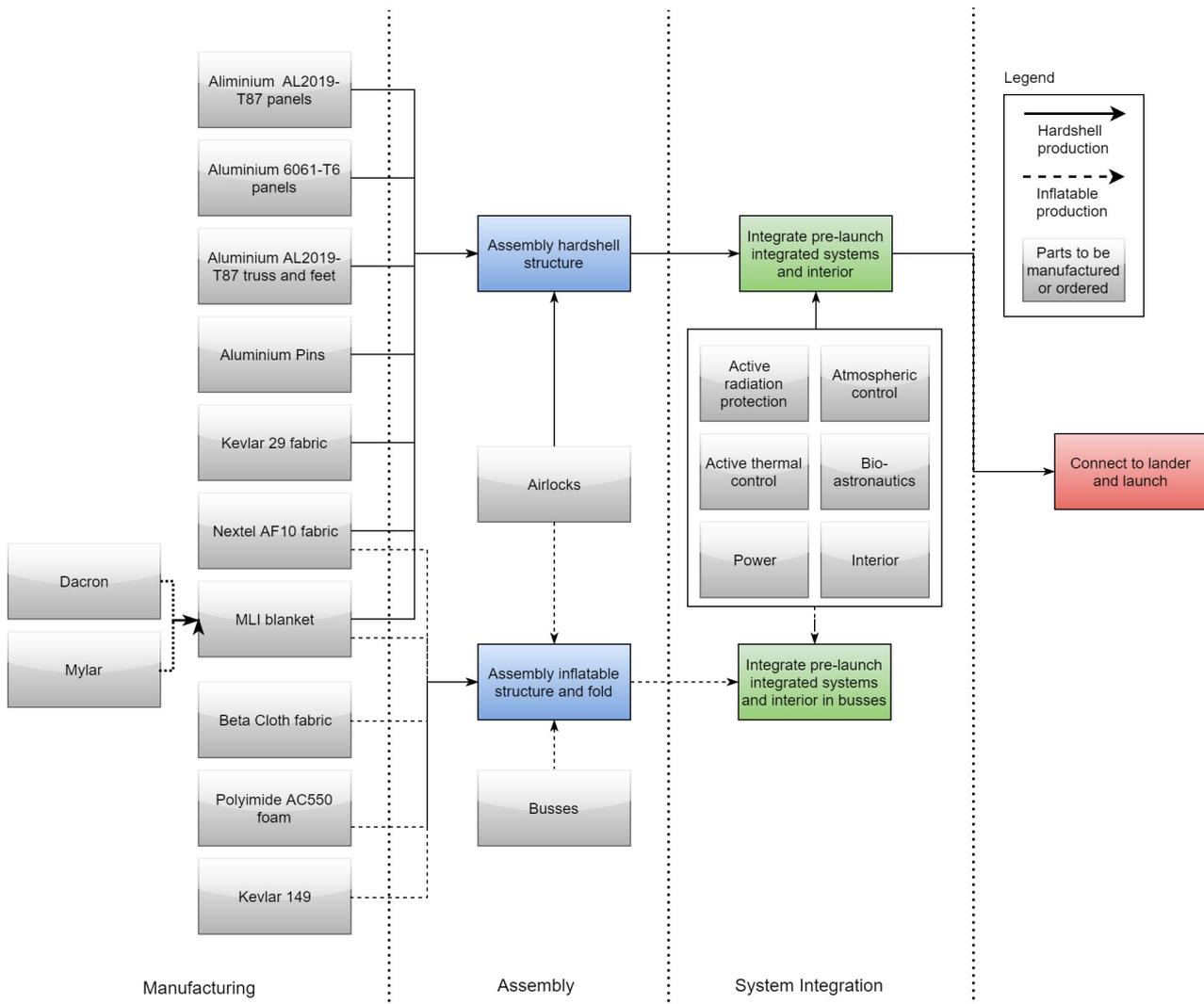
Figure 15.6: Rough production plan.
