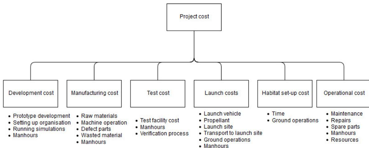
Figure 16.1: Cost breakdown structure of the lunar habitat.
