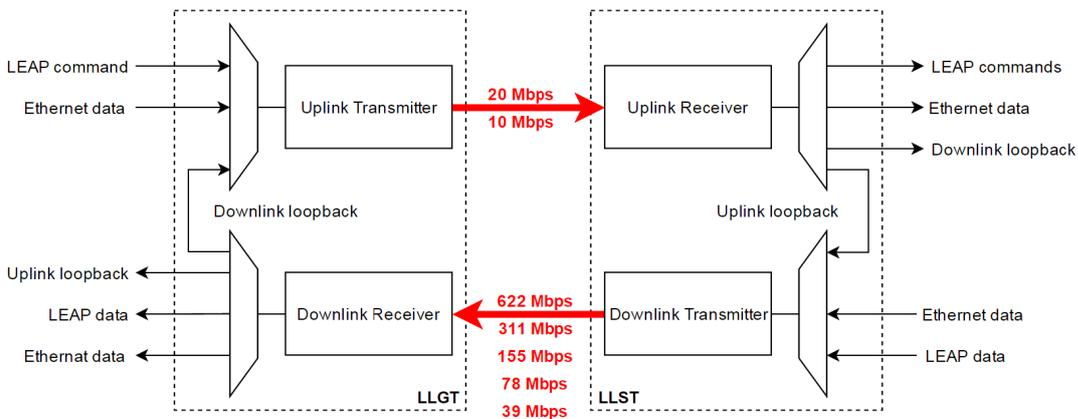
Figure 6.4: Data path of the lunar laser communication system [35].
