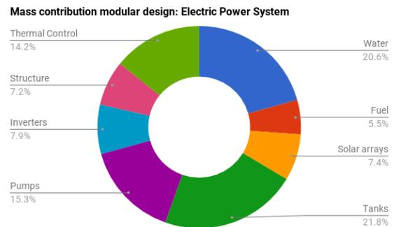
Figure 8.4: Mass contributions of the modular power system design.
