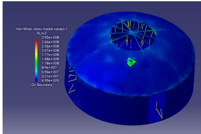
Figure 4.4: Structural analysis results for first iteration of hard-shell module generated in CATIA.
