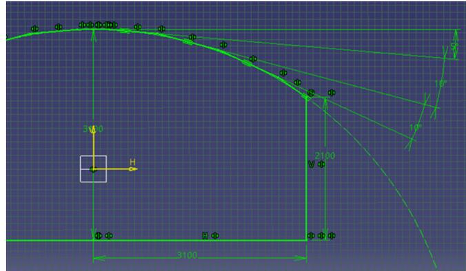
Figure 4.13: Schematic drawing of front cross section of fourth iteration of hard-shell module.
