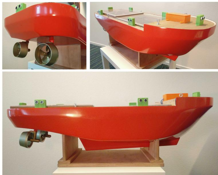
Figure 2.1: An overview of DASh. The colored boxes on deck contain indoor positioning sensors.
