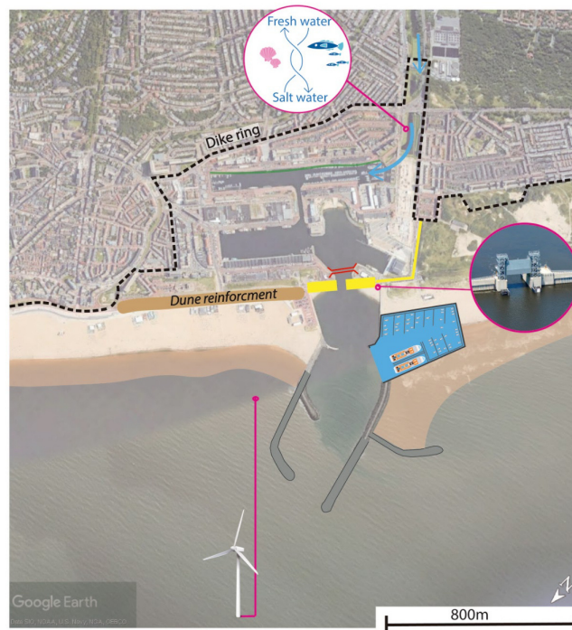
Figure 5.4: Conceptual sketch of Preserve strategy, phase 2: creation of salinity gradient and storm surge barrier in the port area and dune reinforcement in area just north of the port.
