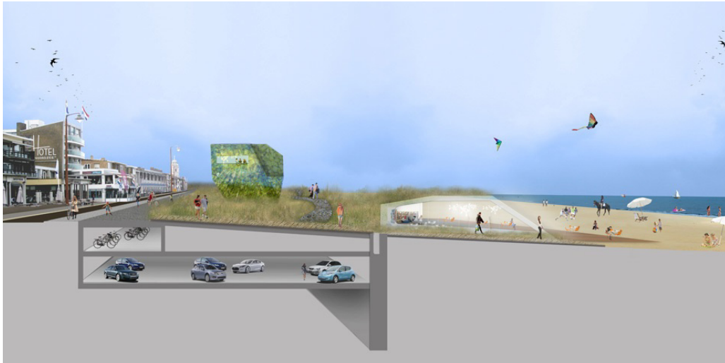
Figure N.6: Katwijk: sketch of the 'wall-in-dunes' alternative, with a parking garage combined in the flood defence (Mark Voorendt, 2021)
