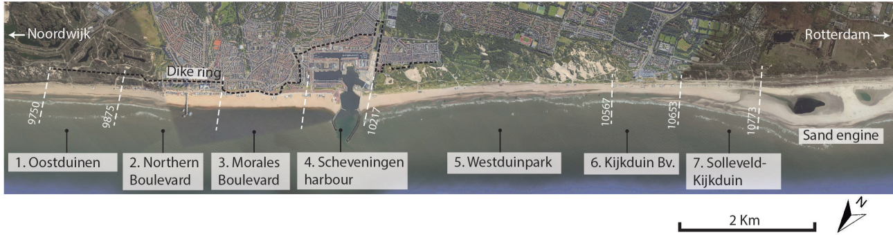
Figure 3.1: Subdivision of the study area into elements according to the type of water structure. Nr 1, 5, 6, and 7 correspond to flexible dune systems. Nr 2 is a fixed dune seawall. Nr 3 and 4 are hard structures (dike-in-boulevard and paved dike, respectively). The different elements are divided by cross-sections following the 'raai' lines defined by Rijkswaterstaat for the entire Dutch coast. Source of the background figure: Google Earth
