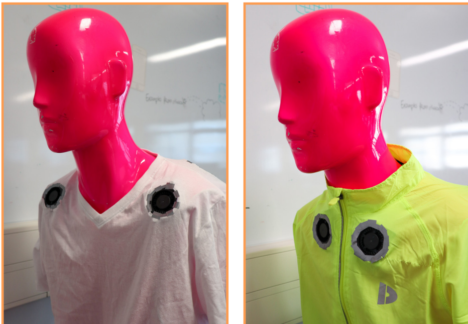
Figure 39: Cotton shirt (left) and windproof jacket (right) used for test (fans were placed at same spot for testing)
