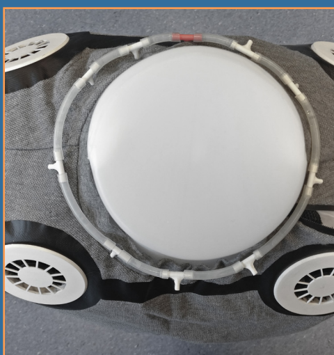
Figure 61: Placement tubing shown in prototype
