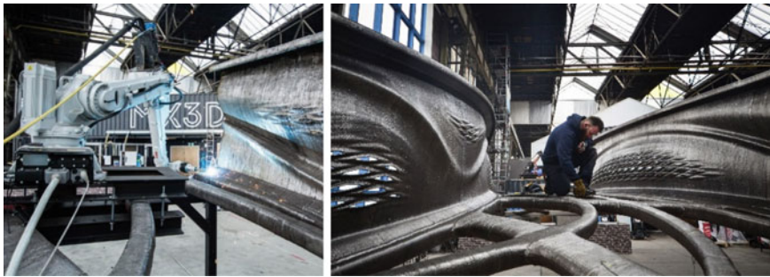
Fig. 4.1 Robotic fabrication of the metal MX3D bridge (2021)
