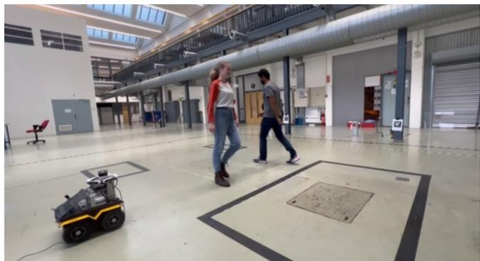
Fig. 1: Jackal robot used for recording pedestrian trajectory data at 3me faculty, TU Delft. The available detection and tracking pipeline can be used to observe the surrounding pedestrians continuously and adapt the behavior to new social contexts.
