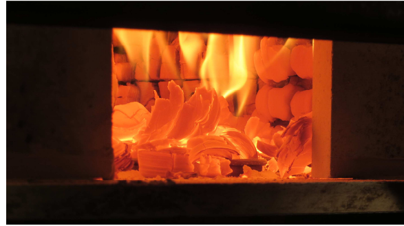
Figure 6.72 Delaminated and fallen pieces of CLT lie on the compartment floor. The CLT wall is in flaming combustion.
