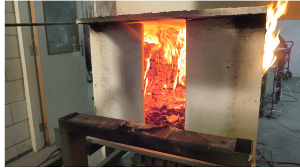
Figure 6.60 Flames were observed to penetrate the left-hand side CLT at the end of the experiment.
