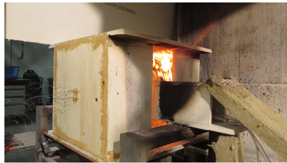
Figure 6.80 Flaming combustion increased in intensity and the complete compartment became involved in flaming again.
