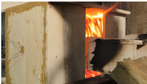
Figure 6.92 After seizing the propane fire, the intensity of flaming reduced.
