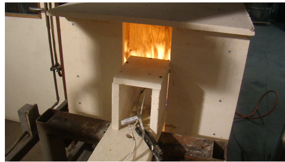
Figure 6.44 After ignition of the burners, the heat flux sensor and its protective encasing were placed inside the opening. The CLT discoloured.
