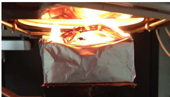
Figure 6.34 Bowing upwards of the top charred lamella of the sample in experiment 15.
