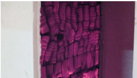
Figure 6.109 The glowing surfaces did not show any sign of delamination or fall-off.
