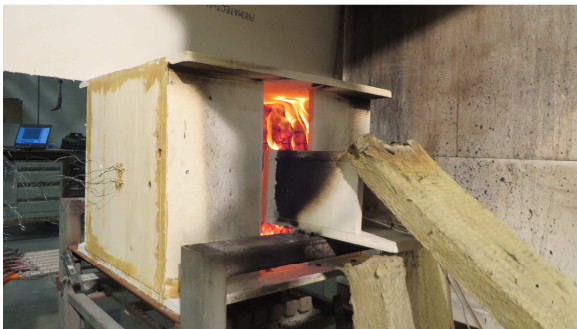
Figure 6.73 Within 10 minutes of reducing the propane flow, external flaming was no longer observed.
