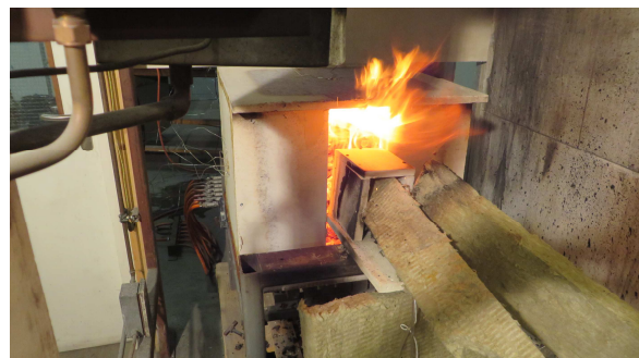
Figure 6.58 External flaming increased in severity after delamination and fall-off of large pieces.
