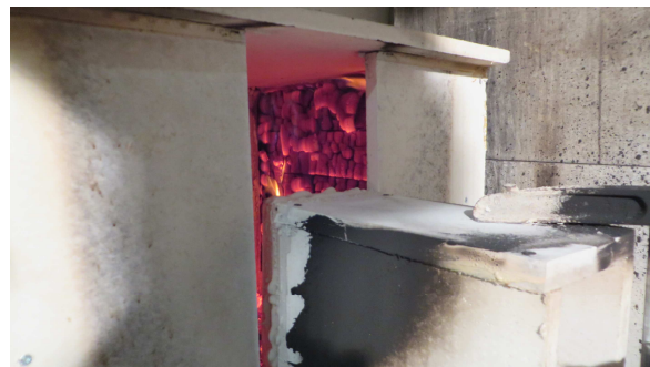
Figure 6.93 At 40 minutes, flaming had almost completely seized and the char was glowing.
