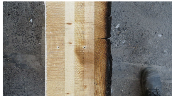
Figure 6.114 Along this edge, the char front progressed 20 mm into the first layer of 40 mm CLT.
