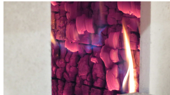
Figure 6.74 Flaming reduced in intensity, but remained visible on certain areas of the char.
