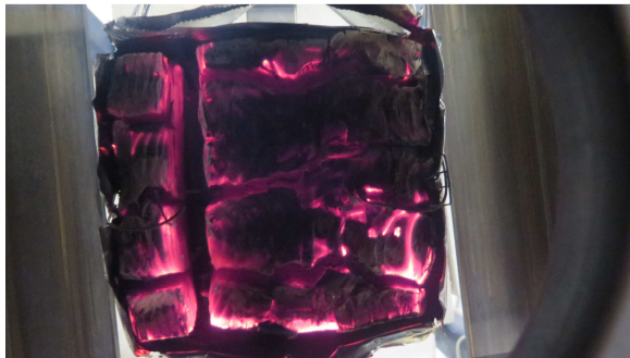
Figure 6.11 1 minute after switching, intense glowing and smoke production were observed, at 6 kW/m 2 exposure and additional airflow of 1,0 m/s.
