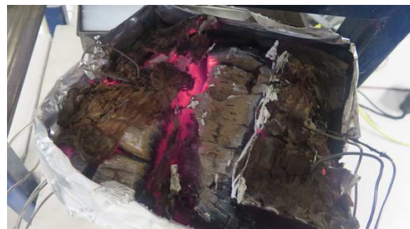
Figure 3.35 Brown-coloured ash after burning through in experiment 13.
