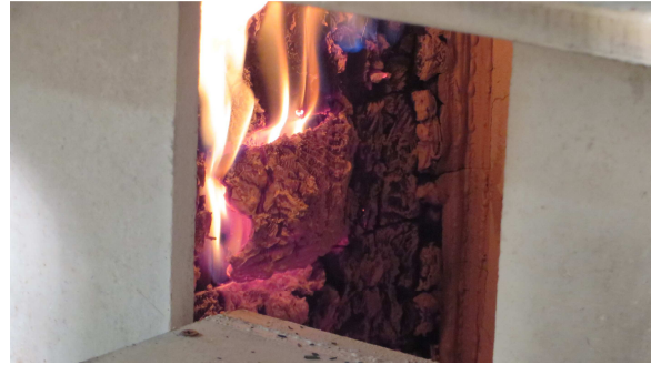
Figure 6.78 At 120 minutes, a piece delaminated on the left side. Flaming occurred behind it.
