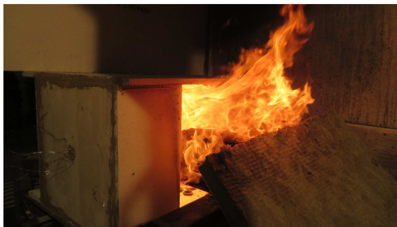
Figure 6.90 After ignition, the compartment became completely involved in flaming combustion.
