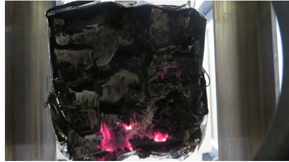
Figure 6.10 30 minutes after switching, glowing increased along the sample edge at 6 kW/m 2 exposure and additional airflow of 0,5 m/s.
