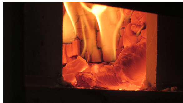
Figure 6.91 Several pieces of CLT delaminated and fell off during the first 25 minutes of the experiment.
