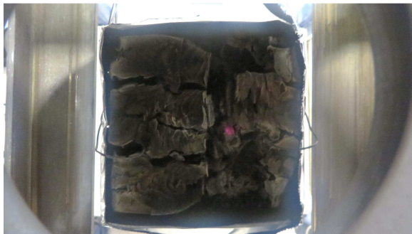
Figure 6.7 1 hour after switching, glowing reduced to only one area and continued to diminish in intensity at 6 \text{ kW/m}^2 exposure.
