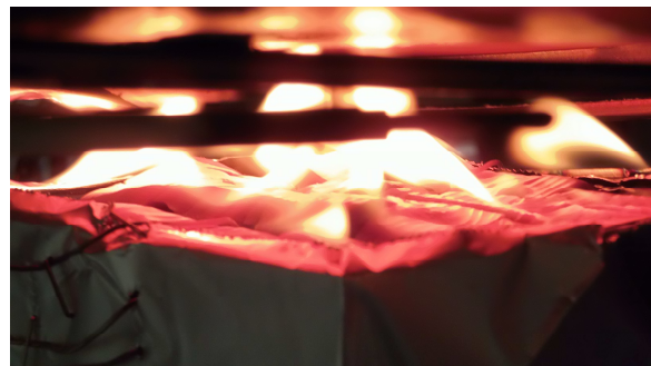
Figure 6.4 Flaming occurred along cracks in the char and along the sample edges. Cracks formed in a typical “alligator” pattern.
