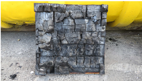
Figure 6.83 Various depths to which the charring front progressed and at which delamination and fall-off occurred.
