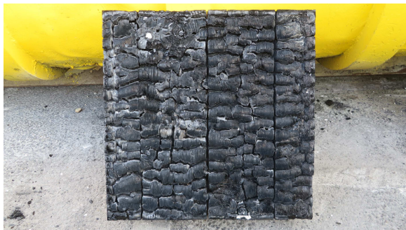
Figure 6.113 The charred surface had an alligator pattern. The boards are clearly visible.
