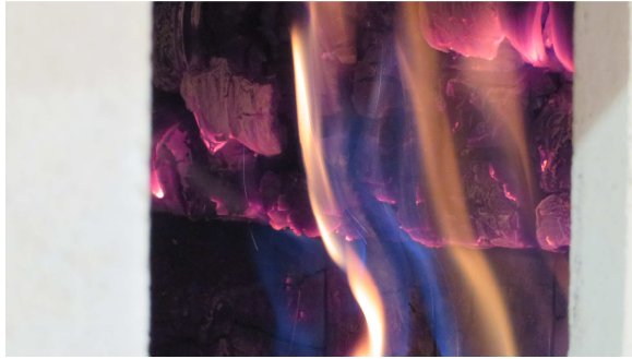
Figure 6.77 Local flaming occurred at the location where the CLT had fallen off.
