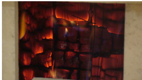
Figure 6.48 Flaming quickly seized and the char glowed. Glow could be clearly observed along the edges where pieces of CLT had fallen off.
