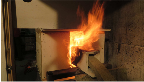
Figure 6.105 After ignition, the compartment became completely involved in flaming combustion.
