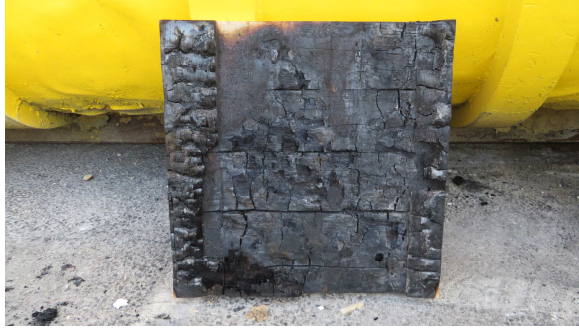
Figure 6.98 In the middle of the right side wall, the char front has progressed into the third layer. Both the 1 st and 2 nd layer had fallen off.
