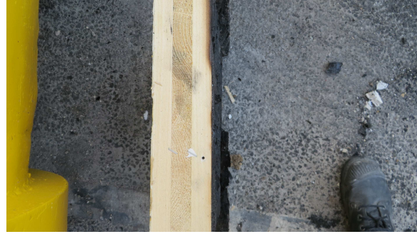
Figure 6.99 Along this edge of the right side wall, the char front progressed to the interface between the 2 nd and 3 rd layer. The 1 st layer has fallen off and the 2 nd layer was removed to reveal unaffected wood.
