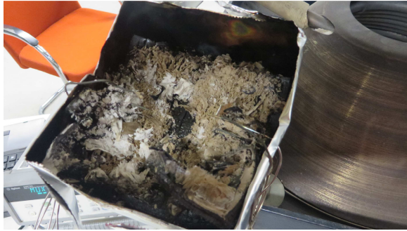
Figure 6.13 An ash layer on top of the char is clearly visible after burn-through at a 10 kW/m 2 exposure.
