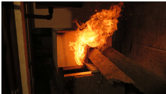
Figure 6.55 After ignition, the compartment became completely involved in flaming combustion.
