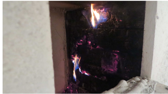
Figure 6.95 After increased glowing, delamination and fall-off, some flaming occurred on the right side.
