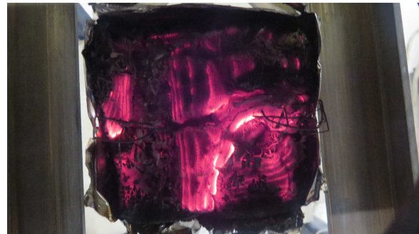
Figure 6.12 15 minutes after switching, intense glowing occurred fairly uniform over the surface, at 6 kW/m 2 exposure and additional airflow of 1,0 m/s.
