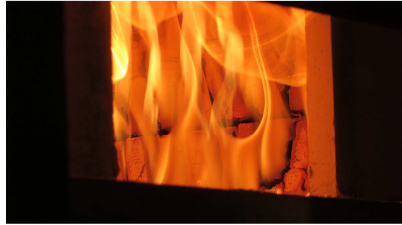
Figure 6.106 No fall-off of char was observed during the initial fire and flaming combustion of the CLT.
