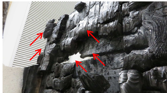
Figure 6.64 Up to 5 different levels of charring and delamination can be observed. In the top left 4 layers remains. Adjacent, 3 layers, then 2 layers, and surrounding the gap only 1 layer.
