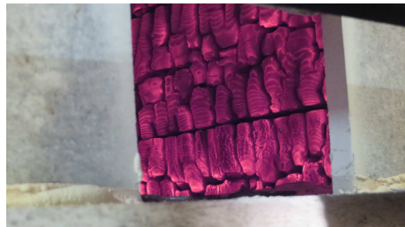
Figure 6.108 The CLT transformed from flaming combustion to smouldering combustion at 30 minutes.
