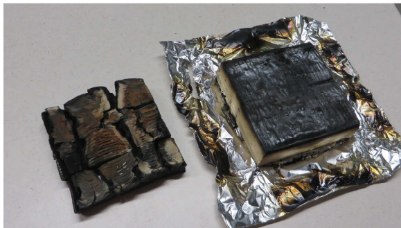
Figure 6.15 Delamination of the sample in experiment 3 with a 0 kW/m 2 exposure. Left the delaminated 20 mm thick top layer, right the remaining sample.
