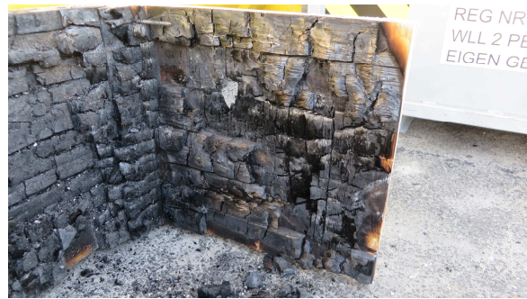
Figure 6.62 Various depths to which the charring front progressed and at which delamination and fall-off occurred.
