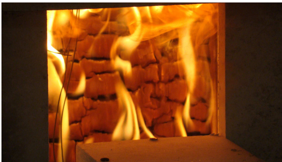
Figure 6.47 Once the propane fire was stopped, flaming quickly decreased and could be observed over the charred CLT surfaces.
