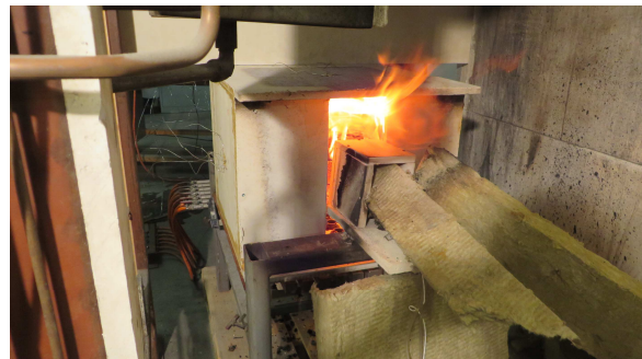
Figure 6.56 After seizing the propane fire, the intensity of flaming reduced.
