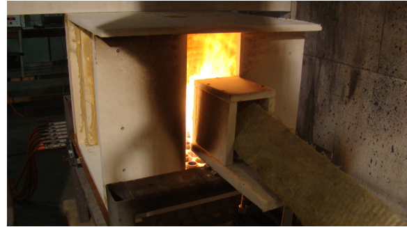
Figure 6.46 After reduction of the burner bed HRR to 41 kW, flaming was largely contained within the compartment.
