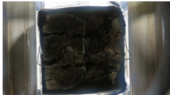
Figure 6.8 2 hours after switching, glowing and smoke production are no longer observed. The sample has extinguished under 6 \text{ kW/m}^2 exposure.
