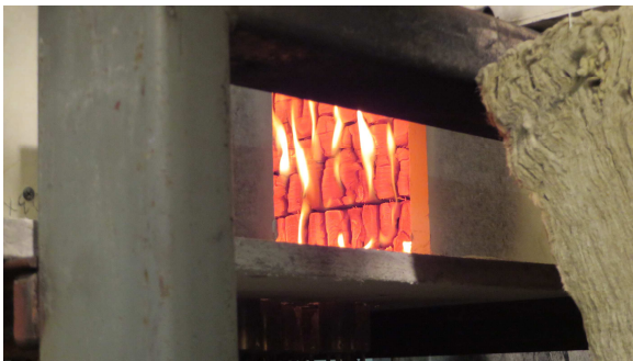
Figure 6.107 After seizing the propane fire, the intensity of flaming reduced. The CLT was in flaming combustion. No pieces of char had fallen off.
