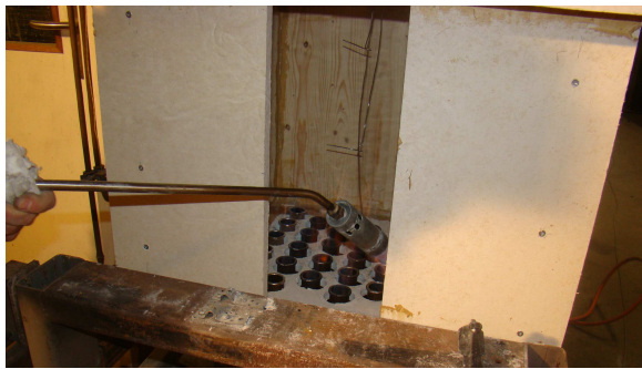
Figure 6.43 At the start of the experiment, all propane burners were ignited with a torch. The burner bed HRR was increased to 63 kW.
