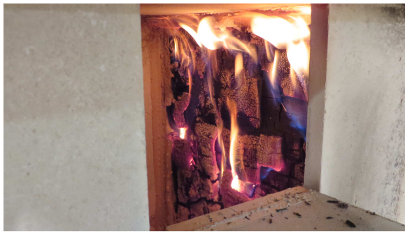
Figure 6.79 At 140 minutes, delamination and fall-off occurred on both side walls. Both walls again entered a phase of flaming combustion.
