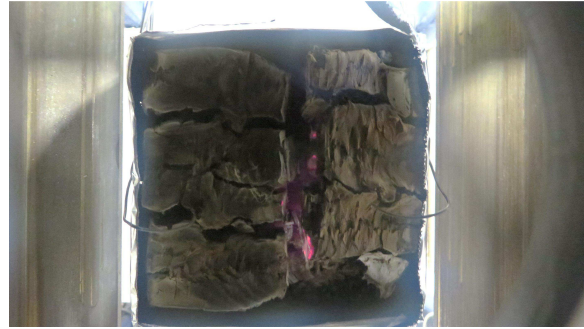
Figure 6.6 After an initial decrease, glowing and smoke increased again in a wide central crack, 40 minutes after switching at 6 \text{ kW/m}^2 exposure.
