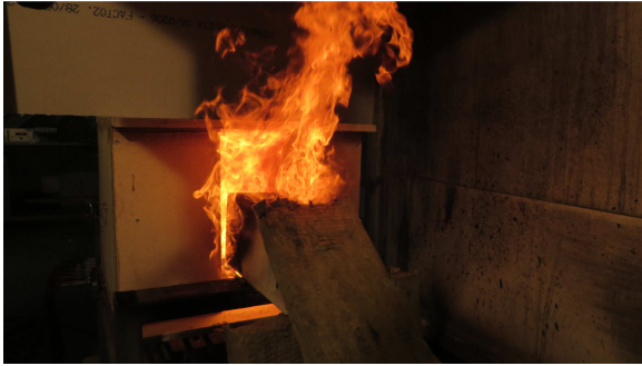
Figure 6.71 After ignition, the compartment became completely involved in flaming combustion. External flaming was observed.
