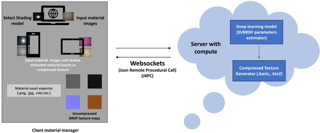
Figure 2: The architecture of our material predictor framework
