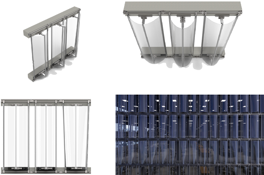
Figure 2: Renderings of the proposed adaptive thin glass façade [Ribeiro Silveira, 2016]
