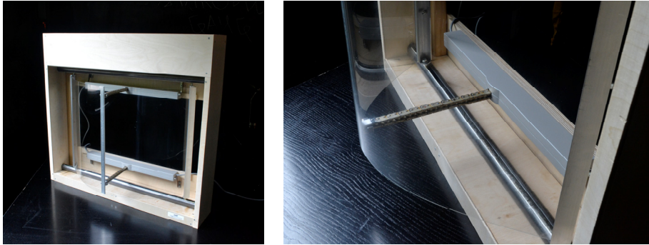
Figure 3: Mock-up of the proposed adaptive thin glass façade [Ribeiro Silveira, 2016]
