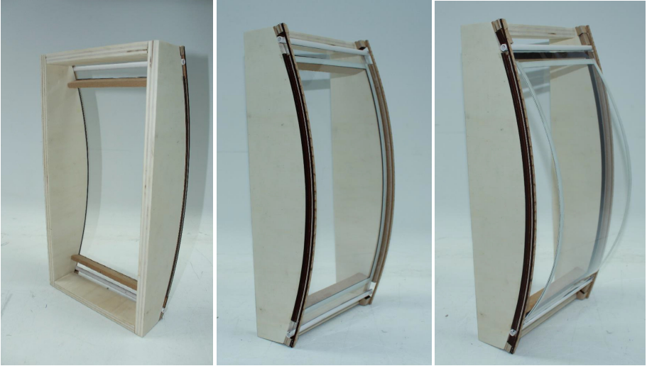
Figure 5: Mock-up of adaptive thin glass façade with magnetic sealing at the edges [Topcu, 2017]
