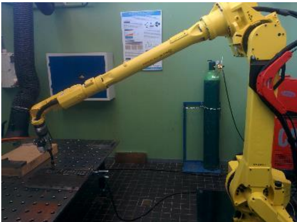
Figure 3-1: The welding setup is a FANUC M710iC 6-axis robotic arm with Fronius welding torch. Photo was taken at the TU Delft welding labs.
