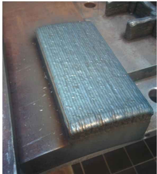
Figure 3-5: Block C consisting of 10 layers, deposited in a unidirectional deposition strategy.
