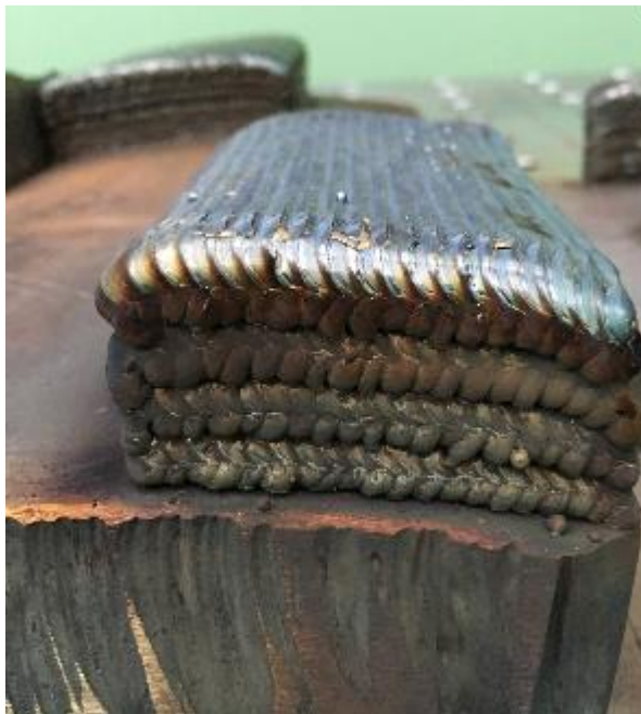
Figure 3-4: Block B consisting of 10 layers, deposited in a back and forth deposition strategy. (shows only 8 here)
