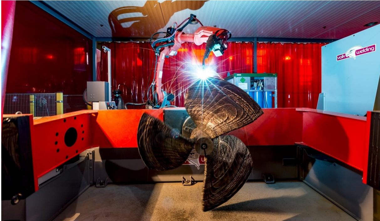
Figure 1-1: WAAMPeller, designed and produced by RAMLAB in collaboration with DAMEN [1]. The propeller is made of 298-layers of nickel-aluminium-bronze alloy.
