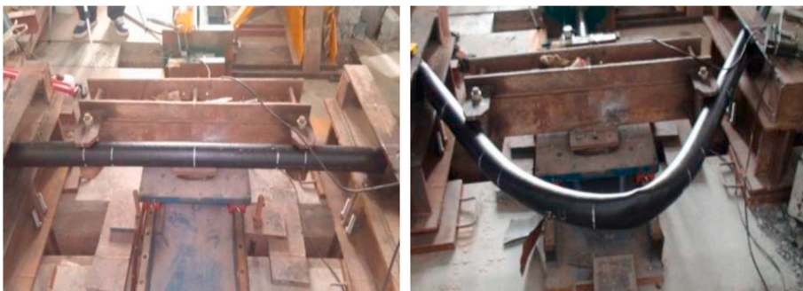
Fig. 12. MFSP specimen before and after bending.
