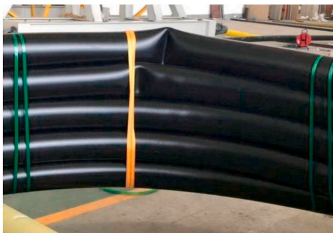
Fig. 3. Buckling failure of MSFP.
