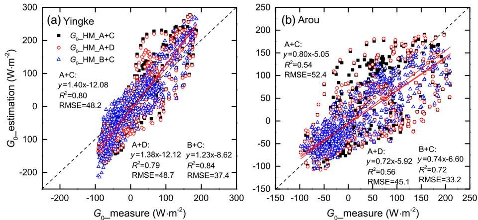
**Fig. 6** Scatterplot of  $G_0$  estimation for cases A, B, C, and D in Table 3 versus *in situ*  $G_0$  measurement, respectively, on 14 days (14, 22, 23, 25, 28, 29, 30 in May and 17, 19, 21, 23, 24, 26, 28 in July of 2009) (a) at the Yingke site and (b) at the Arou site.
