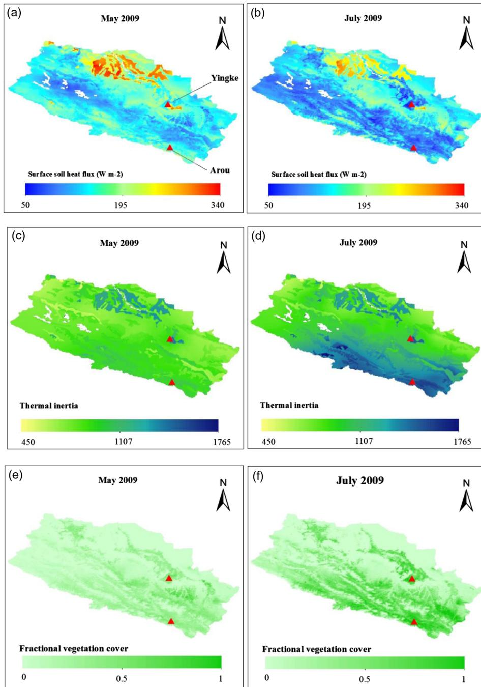
**Fig. 4** The distribution of mean monthly  $G_0$  estimation at 10:30 am local time (a) in May and (b) in July, the distribution of mean monthly thermal inertia (c) in May and (d) in July, and the distribution of monthly  $f_c$  (e) in May and (f) in July in 2009 in the upper and middle reaches of the HRB.
