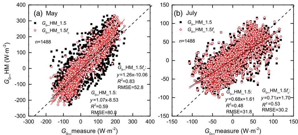
**Fig. 3** Scatter plot of  $G_0$  measurement and  $G_0$  estimation by HM model in the whole (a) May and (b) July of 2009 at the Yingke site.  $G_{0\_measure}$ ,  $G_{0\_HM\_1.5}$ , and  $G_{0\_HM\_1.5f_c}$  are the same as in Fig. 2.
