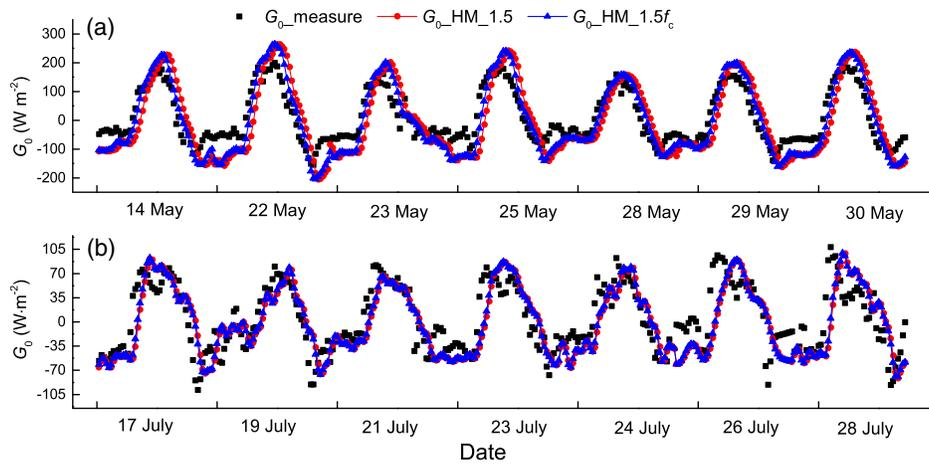
**Fig. 2** The diurnal variations of  $G_0$  on some days in (a) May and (b) July of 2009 at the Yingke site.  $G_{0\_measure}$  is the *in situ* measurements of surface soil heat flux,  $G_{0\_HM\_1.5}$  and  $G_{0\_HM\_1.5f_c}$  are calculated by HM model with time offset of 1.5 h and  $1.5f_c$  h, respectively, using *in situ* measurements of LST.
