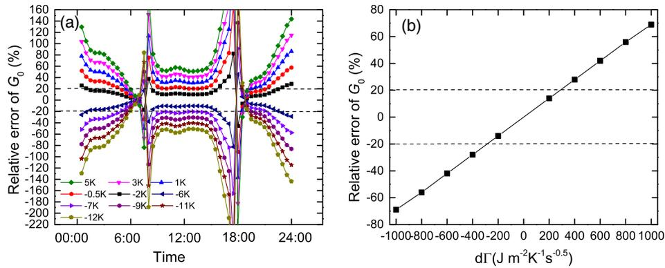
**Fig. 7** The mean RE on  $G_0$  in 14 days (14, 22, 23, 25, 28, 29, 30 in May and 17, 19, 21, 23, 24, 26, 28 in July of 2009) with (a) varied amplitude of LST and (b) varied thermal inertia at the Yingke site.
