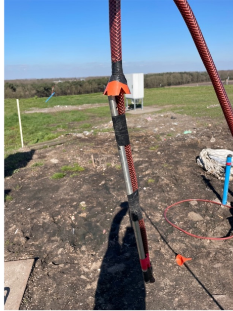
Figure 4.5: One cone with added cutouts attached to the end of the hosepipe.
