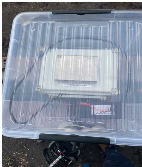
Figure E.1: Overnight set-up of a dilution test, datalogger and external battery were secured in a plastic box. The rod with the fluorometer was attached to the piezometer with tape. A hole in the box allowed for the rod to attach to the datalogger.
