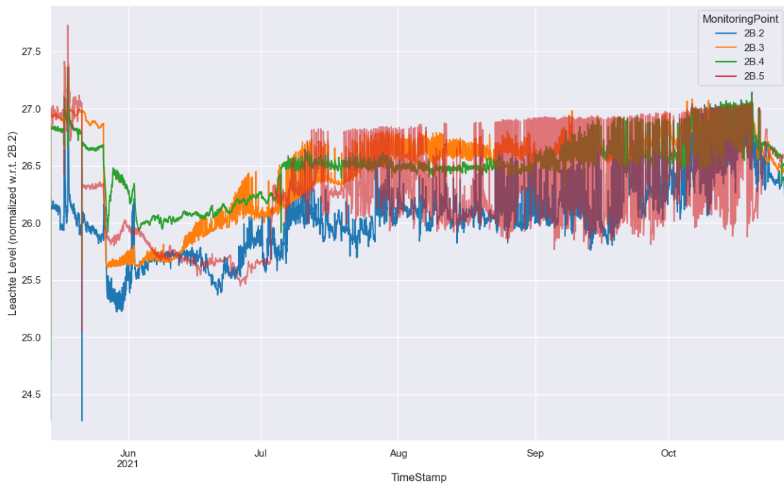
Figure F6: Leachate levels measured by pressure gauges across RIS drain 2B, normalized with respect to point 2B.2.
