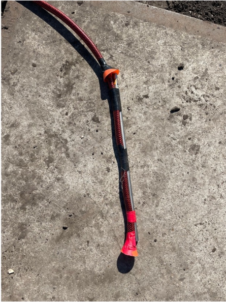
Figure 4.4: Two cones attached to the end of the hosepipe, used for dilution test 5.13-1.
