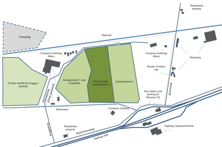
Figure 2.1: Aerial overview of landfill De Kragge II, indicating the division in different compartments (1 to 4). Former landfill De Kragge I is located on the left side. Figure adapted from Kanen & Kedzia-Kowalski (2021).
