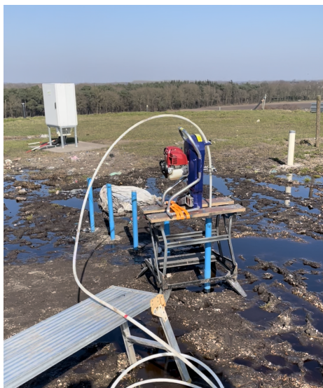
Figure D.2: Purging set-up, the water sampling pump was strapped to a bench and the leachate was collected in a bucket (not visible on picture).
