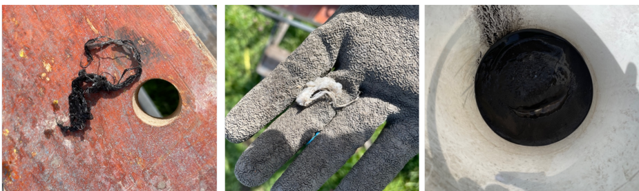
Figure 4.3: Left and middle picture: pieces of plastic attached to the dip-meter and inertial pump. Right picture: \pm 1 cm of sediment (clay/silt) that came out while purging 7.15 (volume of the bucket is about 10 L).
