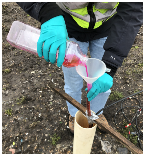
Figure 4.7: Adding the tracer to the hosepipe through a funnel.
