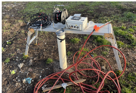
Figure 4.6: Set-up for a uniform dilution test. From left to right on the bench: Cyclops-7F sensor attached to a 22 m rod, which is attached to the data logger. A funnel to pour in the tracer and the hosepipe with a cone and weight attached.
