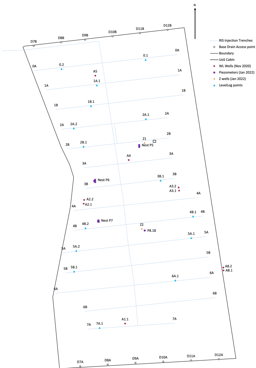
Figure 2.5: Schematic overview of the infiltration trenches and wells and piezometers in compartment 3 of De Kragge. RIS = Recirculation-infiltration-system, UoS = University of Southampton, WL = water level, LevelLog = automatic leachate level measuring device.
