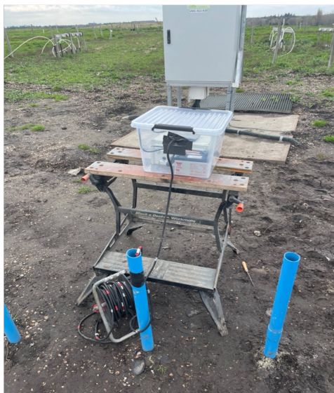
Figure E.1: Overnight set-up of a dilution test, datalogger and external battery were secured in a plastic box. The rod with the fluorometer was attached to the piezometer with tape. A hole in the box allowed for the rod to attach to the datalogger.
