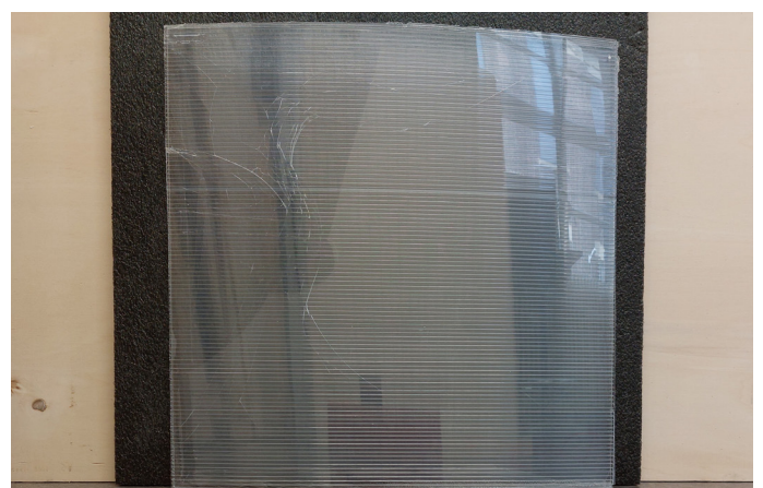
Specimen 3: Permanent deformation of the PC sheet and detachment of the upper glass. Large crack lines on the top glass sheet, smaller ones on the bottom sheet which is still laminated to the PC.
