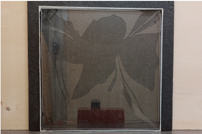
Specimen 1a: Failure of the bottom sheet with large crack lines. Centre pieces fell through.
