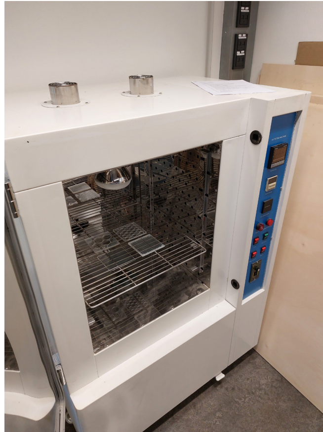
Figure 42: UV accelerated weathering test machine (Author)
