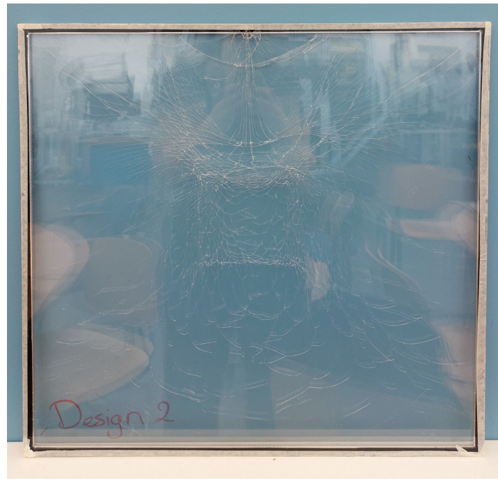
Figure 40: Cracks on specimen 3 after the test (Author)
