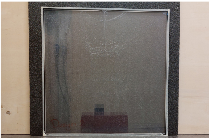
Specimen 2: Smaller crack lines due to lamination layer. The bottom layer was still intact. No pieces fell out.
