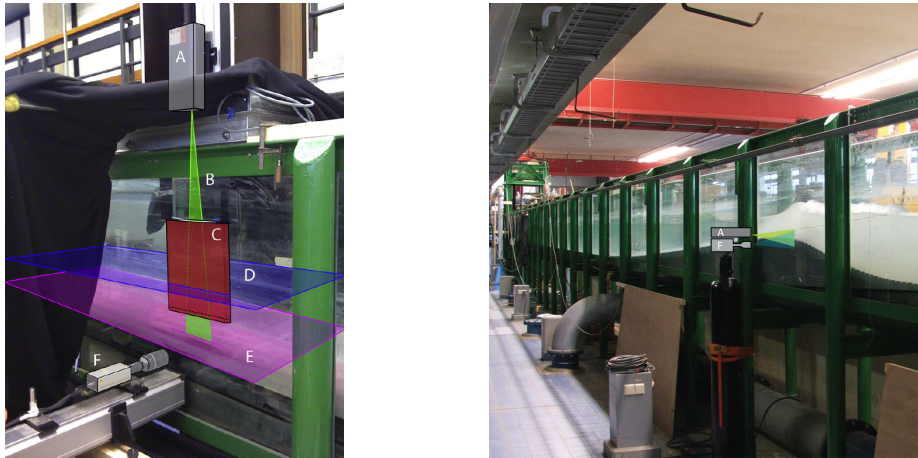
(a) Common PIV set-up with laser on top
