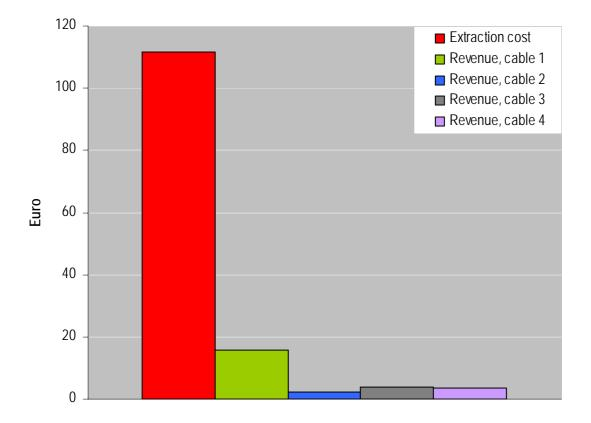
Figure 1. Scenario A: Total cost for separate extraction of hibernating cables in city environment versus revenues for different types of recovered cables (Cable 1=6–24 kV copper power cable; Cable 2=6-24 kV aluminum power cable; Cable 3=0.4 kV copper power cable; Cable 4=0.4 kV aluminum power cable). The data is presented in Euros per meter of excavated shaft.
