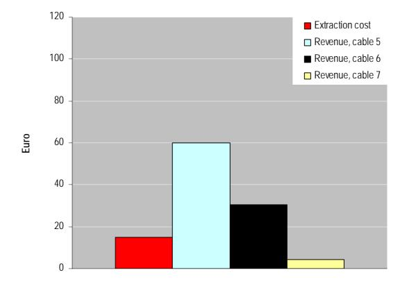
Figure 2. Scenario B: Total cost for separate extraction of hibernating cables in rural environment versus revenues for different types of cables (Cable 5: Transport communication copper cable; Cable 6: 36-72 kV copper power cable; Cable 7: 36-72 kV aluminum power cable). The data is presented in Euros per meter of excavated shaft.
