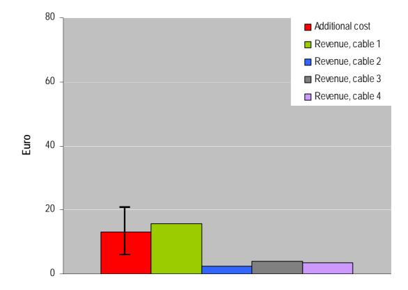
Figure 3. Scenario C: Estimated additional cost for integrated extraction of hibernating cables in city environment (including an uncertainty interval) versus revenues for different types of cables (Cable 1: 6-24 kV copper power cable; Cable 2: 6-24 kV aluminum power cable; Cable 3: 0.4 kV copper power cable; Cable 4: 0.4 kV aluminum power cable). The data is presented in Euros per meter of excavated shaft.
