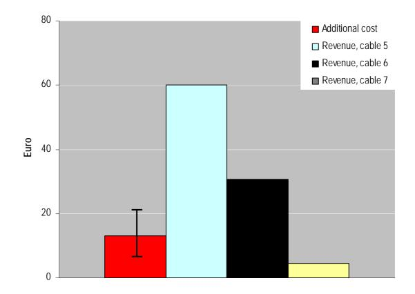
Figure 4. Scenario D: Estimated additional cost for integrated extraction of hibernating cables in rural environment (including an uncertainty interval) versus revenues for different types of cables (Cable 5: Transport communication copper cable; Cable 6: 36-72 kV copper power cable; Cable 7: 36-72 kV aluminum power cable). The data is presented in Euros per meter of excavated shaft.
